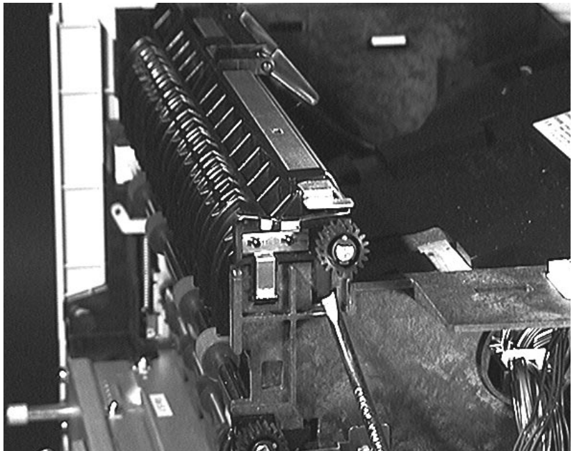
Figure 6-56 Upper Delivery Assembly Tabs
