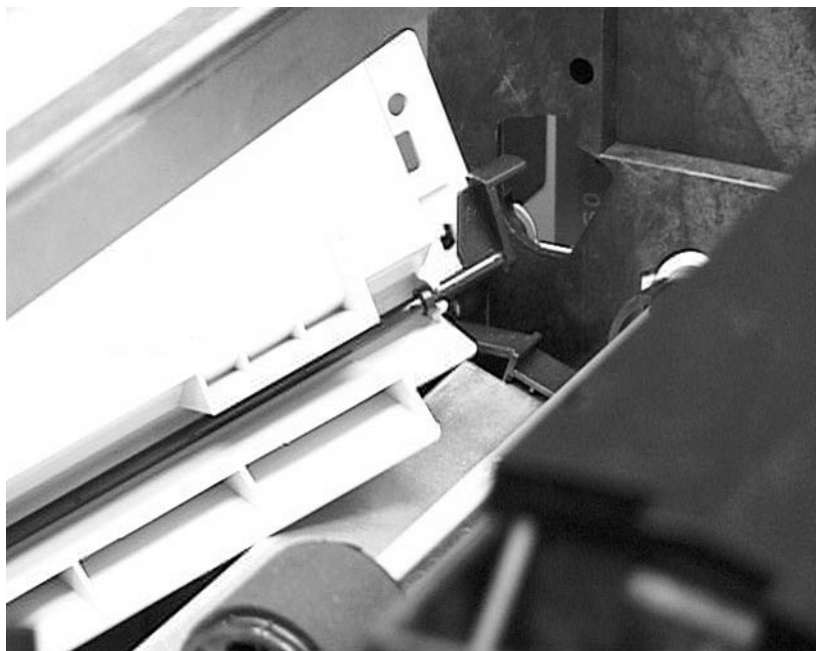
Figure 6-17 Tray 1 Inner Cover Flag (view from inside printer, left side)
