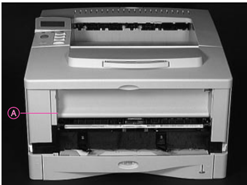
Figure 7-1 Location of the Engine Test Button
