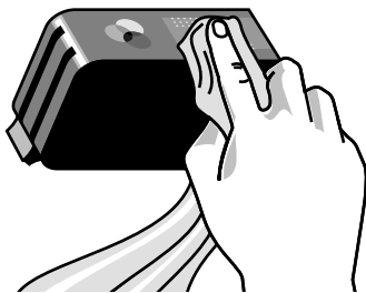
Figure 5.1 Cleaning the Electrical Contacts
