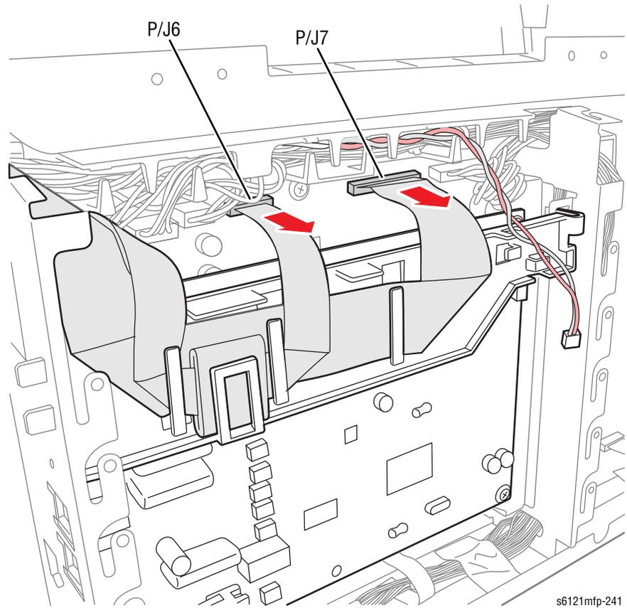
6. Remove 4 screws (metal, 6mm) and remove the Fax Board.
