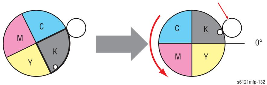
The cartridge replacement position is where the Toner Cartridge Rack is rotated 90° degrees from the developing position.
