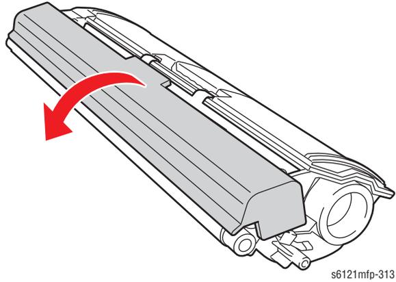
6. Aligning the shaft on both sides of the Toner Cartridge with the rails in the machine, install the cartridge.
