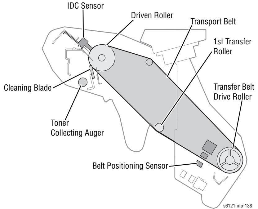
In addition to the Transfer Belt, a Transfer Roller (sometimes referred to as the 2nd Transfer Roller) transfers the composite image to the media for fusing.
