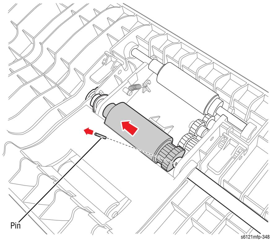
6. Rotate the shaft until you can see the pin sticking through the shaft.
