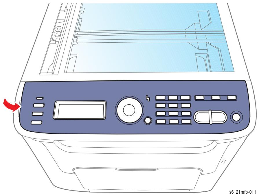
2. Remove 3 screws (silver, tap, 10 mm) that secure the control panel.
