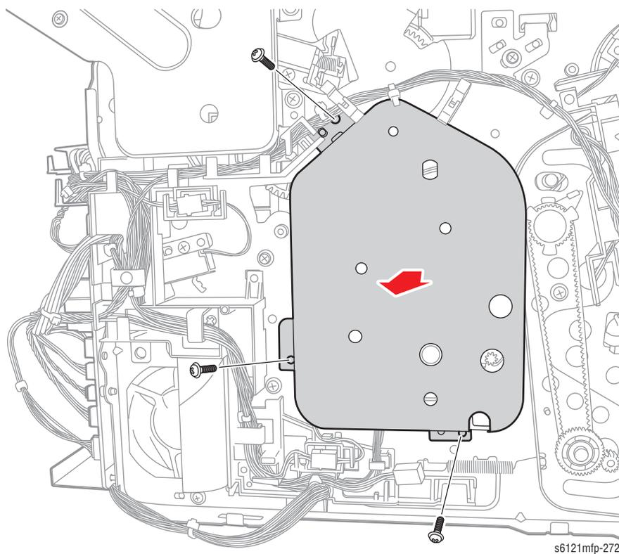
4. Remove the screw (metal, 6mm) and disconnect connector CN3 to remove the Registration Roller Solenoid.
