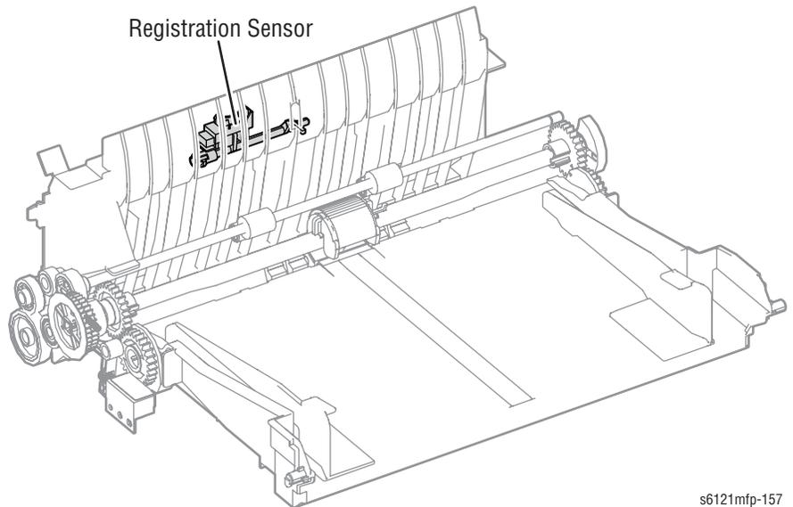
To reduce the number of detected paper misfeeds, another feed sequence is carried out if a registration sensor signal transition fails to occur within a predetermined period of time. If after the second feed attempt media is not detected, a media empty/misfeed condition is reported.
