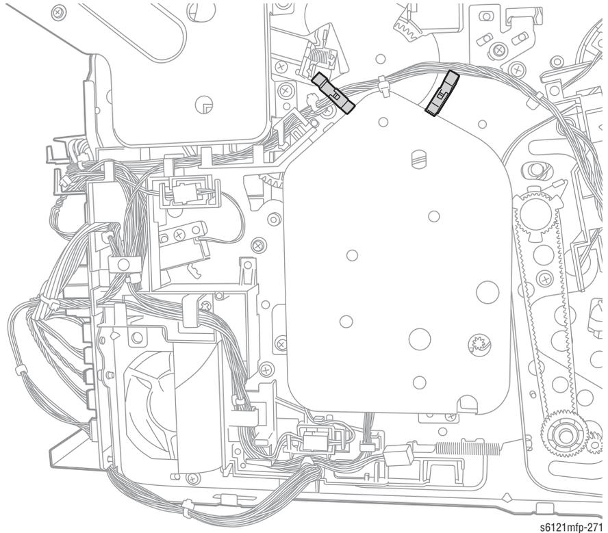
4. Remove 3 screws (metal, 6mm, with washer and lock washer) and remove the cover plate.
