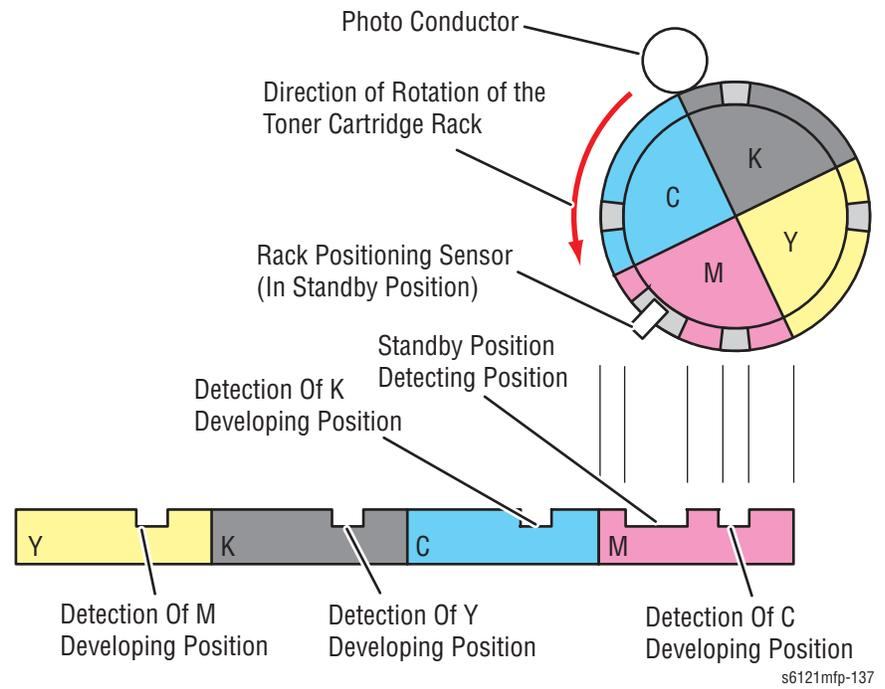
When a replacement request is made for a Toner Cartridge, the Toner Cartridge Rack is rotated 70 degrees from the depleted cartridges' developing position by the Rack Motor.
