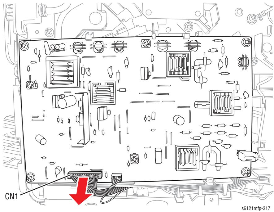
9. Remove 4 screws (one metal, 6mm, and three metal, 8mm). 2 screws are located on each side of the printer.
