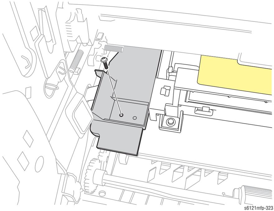
10. Remove 2 screws (metal, 8mm).
