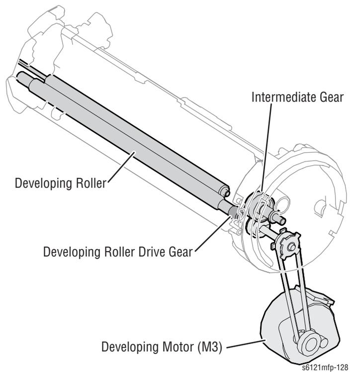
When the Toner Cartridge Rack is stationary at the developing position, the Developer Roller drive gear meshes with intermediate gears allowing the Developing Motor to engage the roller.
