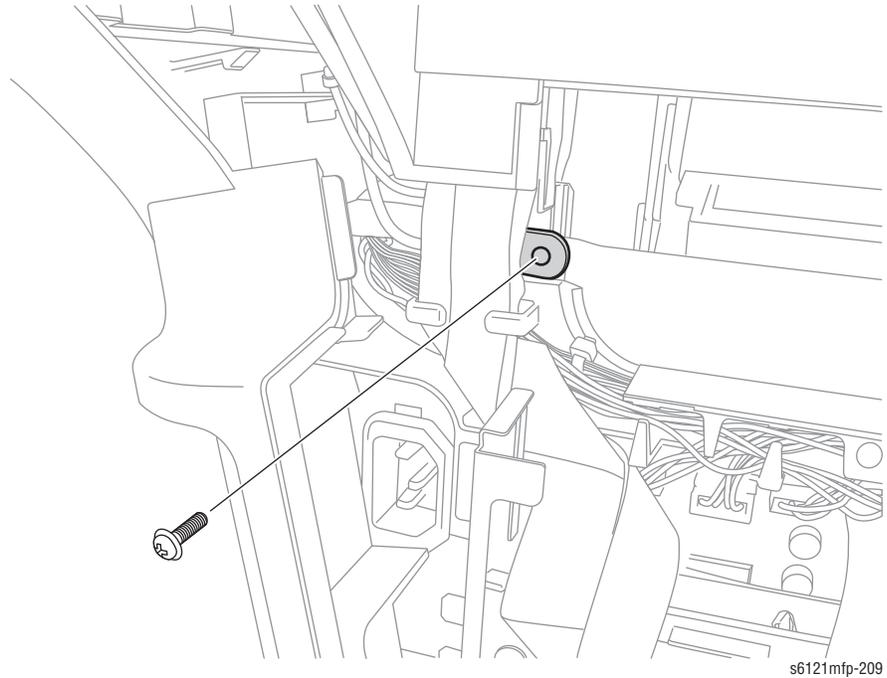
8. On the right side of the printer, remove the ground wire screw (metal, 6mm, with lock washer and flat washer).
