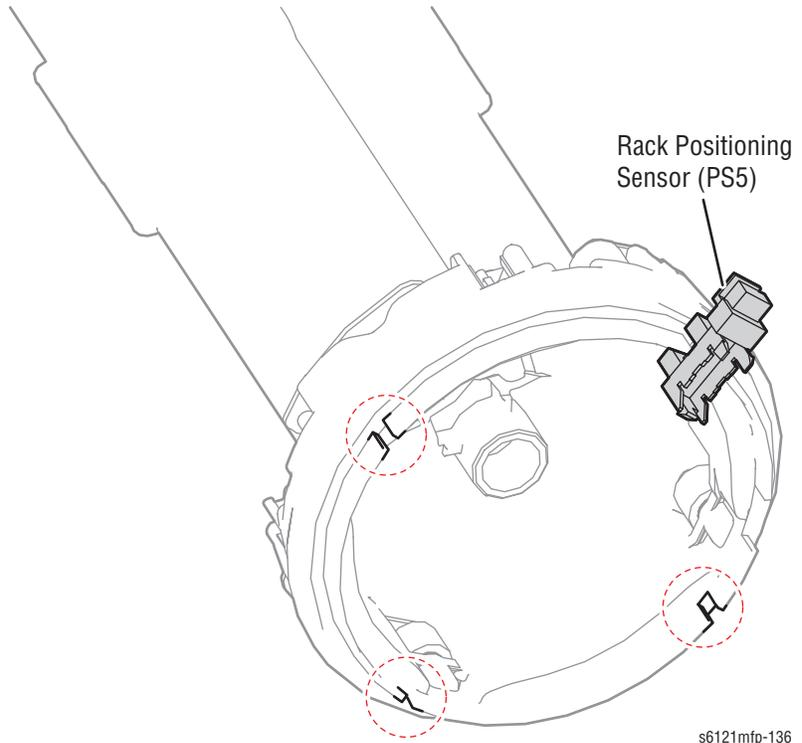
The Magenta Toner Cartridge includes a slit for detecting the standby position. When the Toner Cartridge Rack is rotated, the Rack Positioning Sensor (PS5) detects the standby position slit. To bring the toner cartridge rack to a stop at the corresponding developing position, the rack is rotated from the standby position 62° degrees by the Rack Motor.
