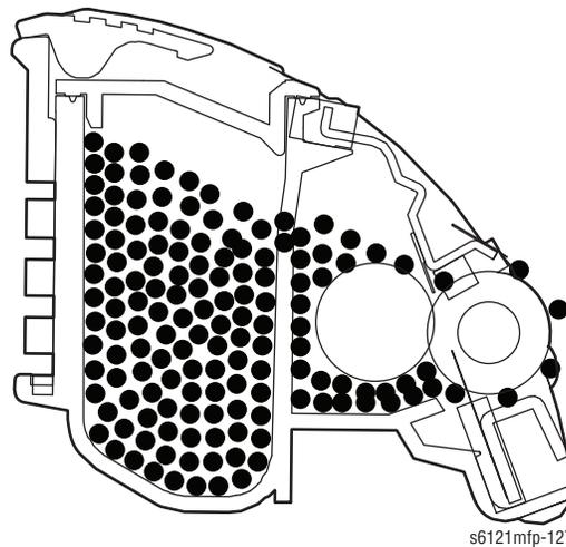
3. Toner then sticks to the electrostatic latent image formed on the surface of the photo conductor drum. That part of toner left on the surface of the developing roller is returned to the toner supply portion.
