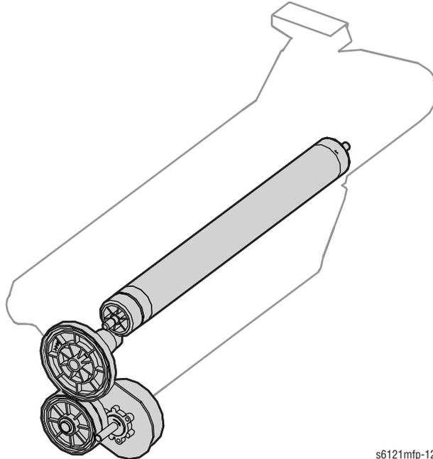
The cleaning blade is pressed against the drum to remove excess toner. Waste toner is stored in the Imaging Unit.
