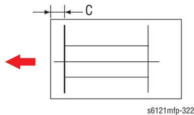
2. Check width C on the printed page produced.
