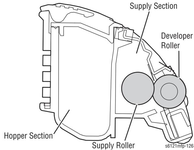
1. Toner stored in the hopper is moved into the toner supply portion by the rotation of the Toner Cartridge rack
