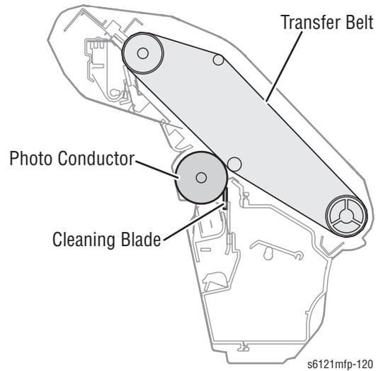
The photo-conductive drum is driven by the Main Motor through a series of gears. When the Main Motor is energized, it turns the drive gear, which in turn rotates the drum.
