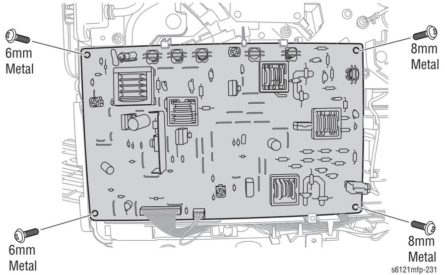
4. Press down on the lower tab and remove the High Voltage Board.
