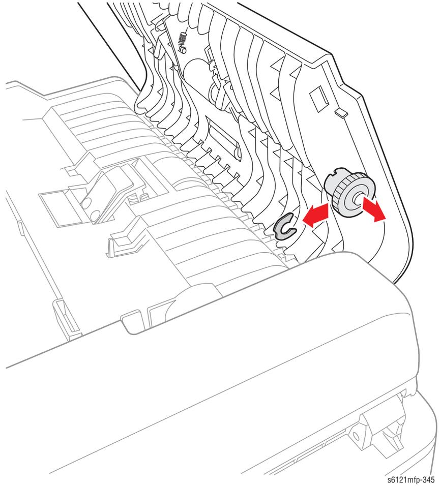
3. Pull up on the bushing tab and rotate the bushing clockwise until you can pull the bushing off of the shaft.
