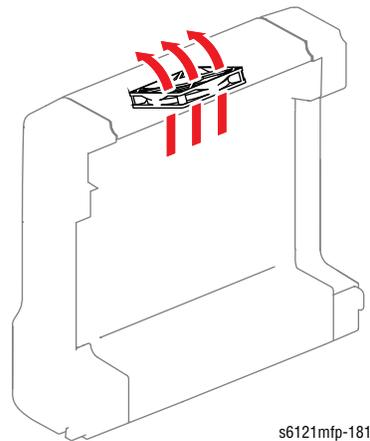
The Duplex Unit Fan operates at full-speed at the start of a duplex operation, and then slows to half-speed after the duplex operation ends. The fan is off when the Duplex Unit is not in use.
