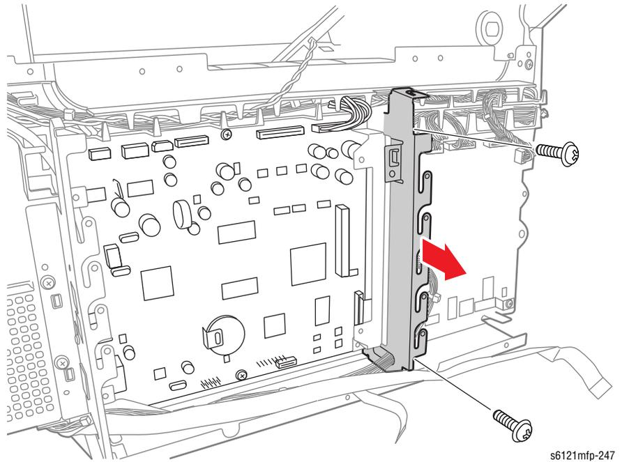
6. Disconnect all connectors from the Image Processor Board.
