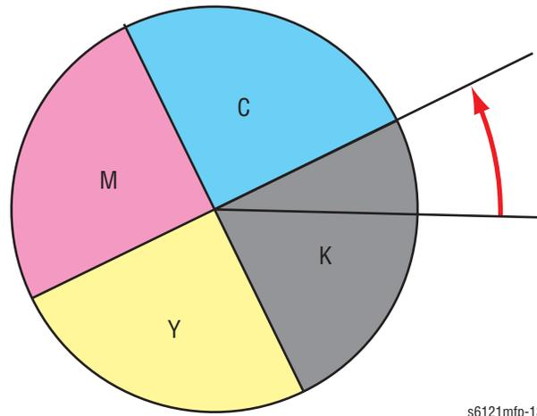
The developing position is where the Toner Cartridge Rack is rotated 62° degrees from the standby position.
