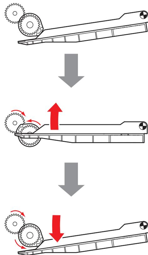
The fixed Separation Pad system plus the Retard Rollers are used for paper separation. This ensures that only one sheet of paper is fed.
