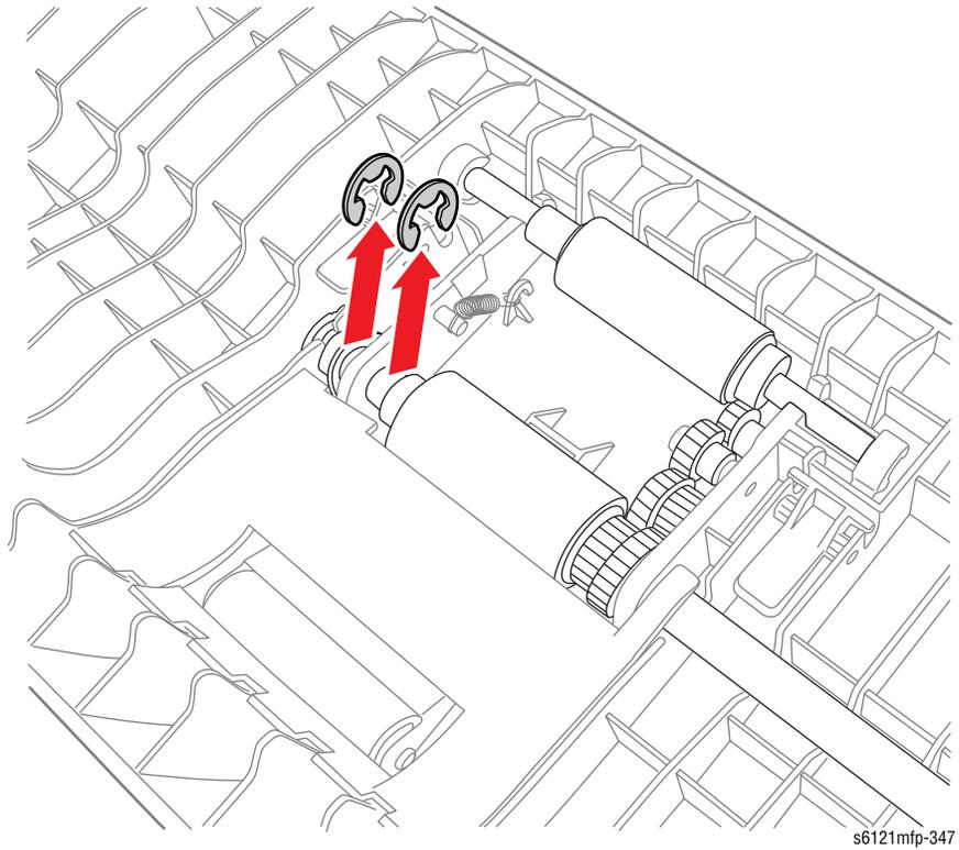
5. Slide the roller and gears in the direction of the arrow.
