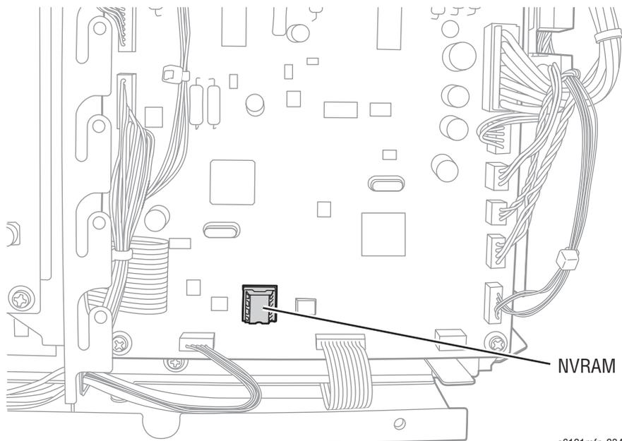
Align the notch on the chip with the notch in the socket.
