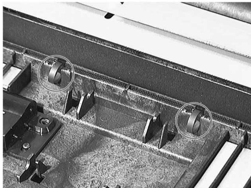
Figure 7-67 Installing the A-1 Belt and Roller
