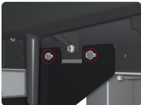
6. Remove two screws that secure the Waste Bottle Holder to the printer.
