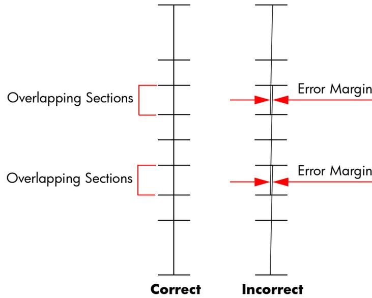
**7** If the Check Slant pattern still shows slant, then loosen very slightly the three screws that secure the Printhead Slot Assembly, and manually adjust the slant.
