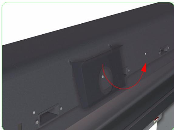
3. Remove five screws that secure the Top Cover to the rear of the Printer.
