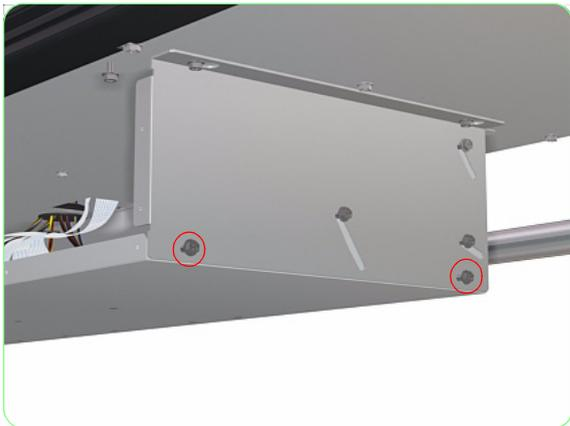
**13.** Remove two screws from the left and right side of the Electronics Module.
