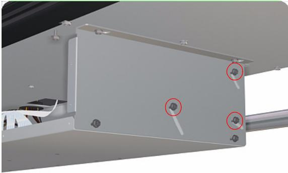
**5.** Loosen three screws on the left and right side of the Electronics Module
