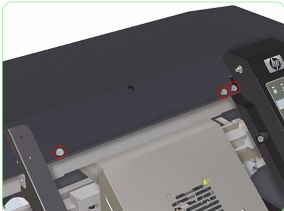
4. Remove two screws that secure the Right Top Cover to the rear of the Printer.
