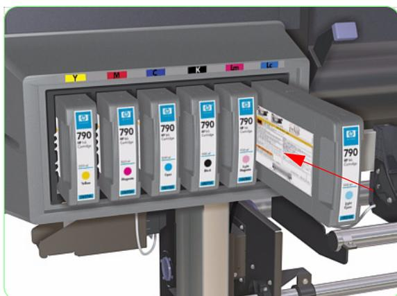
31. When this message is displayed on the Front Panel, re-install the Ink Cartridge that you removed earlier.
