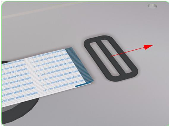
**19.** Remove the Black Cable Clip from the Trailing Cable.
