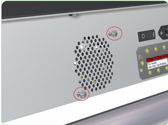
**8.** Remove two screws that secure the Electronics Cooling Fan from the rear of the Electronics Module.
