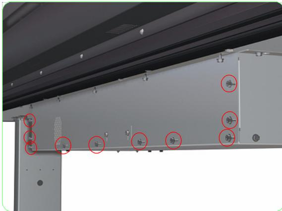
2. Remove ten screws that secure the Front Electronics Module Cover.
