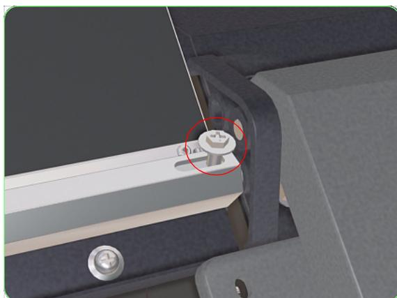
**2.** Loosen the screw that secures the Right Hinge Pin.
