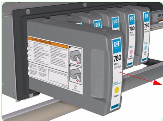
**14.** Remove the Ink Cartridge of the sensor you need to replace.
