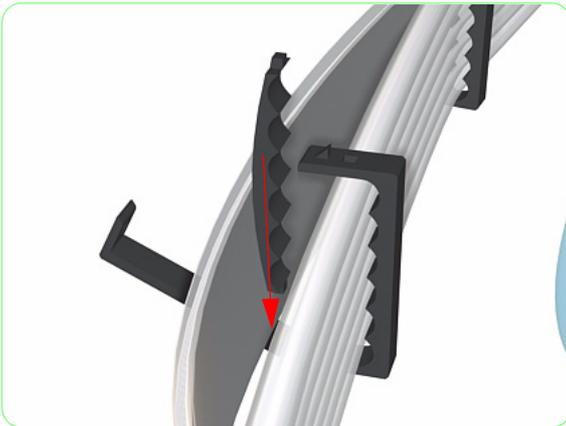
**7.** Insert the center strip and install the clamps along the length of the Trailing Cable and Ink Supply Tubes (should be installed where there is a cutout in the plastic strip that sandwiches the Trailing Cable).
