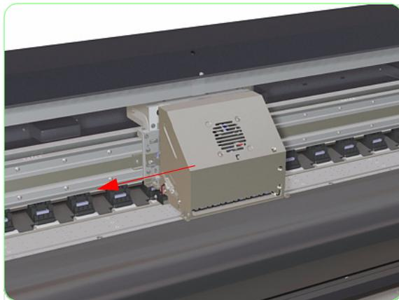
8. Once uncapped, manually move the Carriage Assembly to the left side of the printer.
