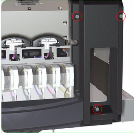
7. Remove three screws that secure the Maintenance Kit Drawer Cover to the Printer.
