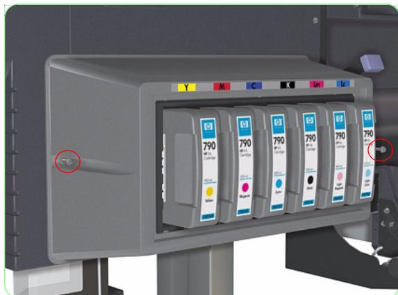
1. Remove two screws (one from each side) that secure the Ink Cartridge Bay Cover to the Printer.
