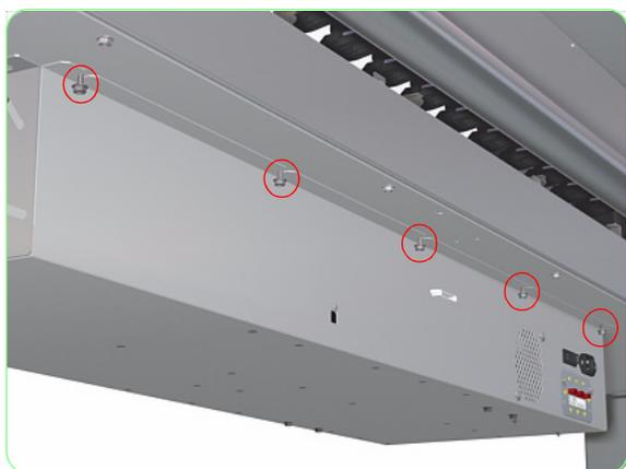
**15.** Loosen five screws that secure the rear of the Electronics Module.
