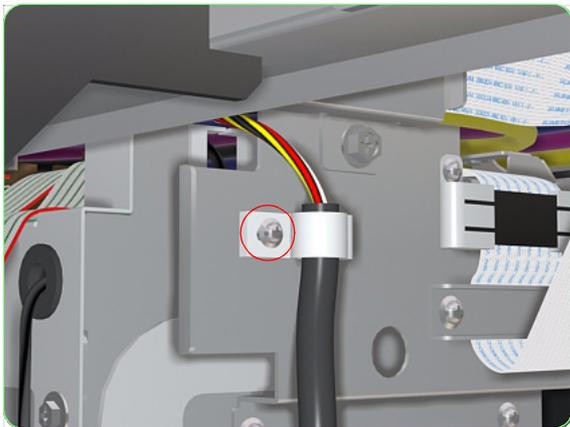
**12.** Remove one screw that secures the Cable Clamp to the Carriage Assembly
