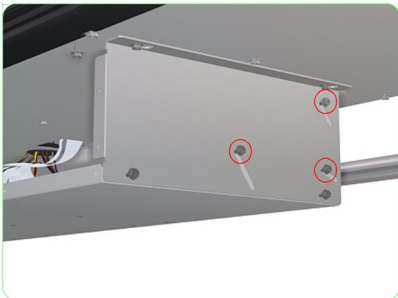
**14.** Loosen three screws on the left and right side of the Electronics Module
