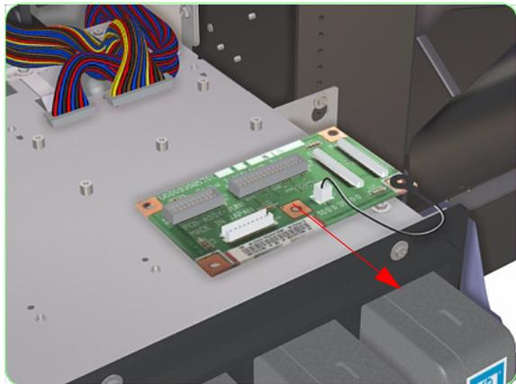
**11.** Remove the ISS PCA from the Printer.
