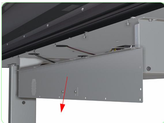
3. Remove the Front Electronics Module Cover.
