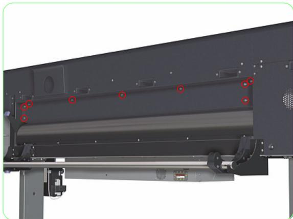
1. Remove nine screws that secure the Back Cover to the Printer.
