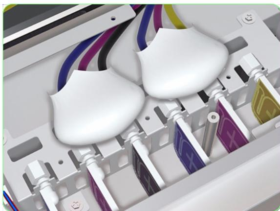
**31.** Use a lint-free cloth or a polyethylene bag to cover the ends of the Ink Tubes so that ink does not drip into the Printer.
