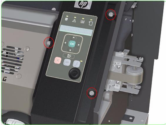
6. Remove the Front Panel from the Printer.
