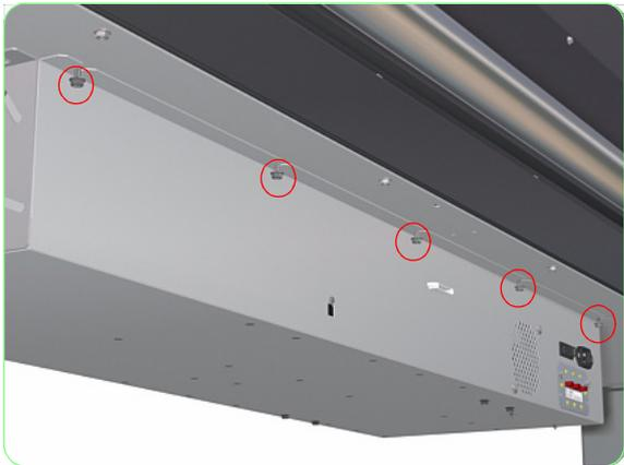
**6.** Loosen five screws that secure the rear of the Electronics Module.
