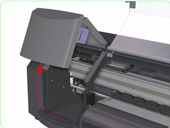
3. Remove two screws that secure the Left or Right Trim to the printer.
