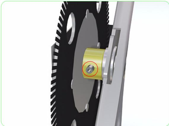
**8.** Loosen the screw that secures the Encoder Disc to the Shaft.
