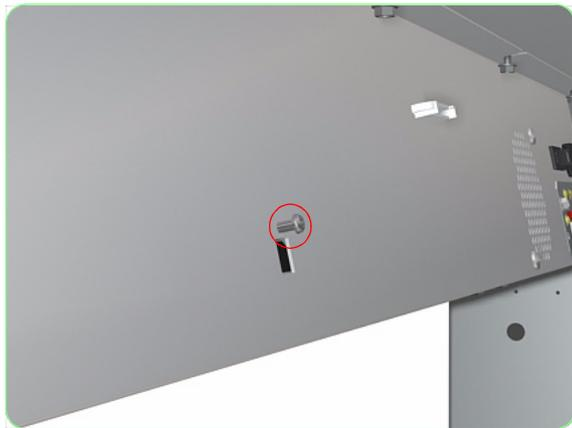
**8.** Remove one screw from the rear of the Electronics Module.
