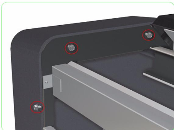
5. Remove two screws (located underneath the Front Panel) that secure the Right Side Cover to the Printer.
