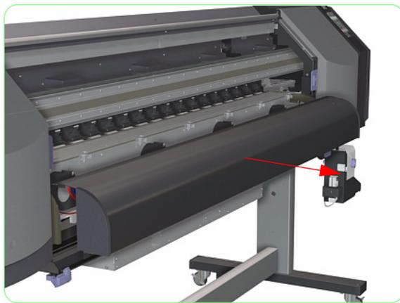
**4.** Pull out the Front Heater slightly.
