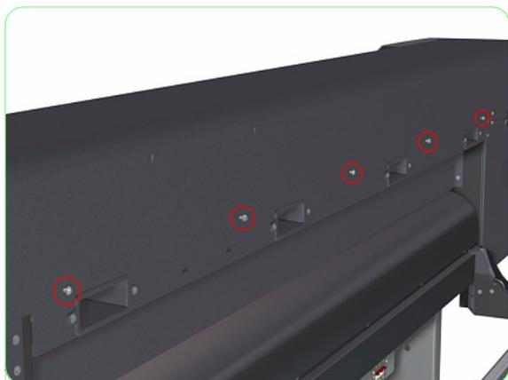
4. Remove three screws that secure the Top Cover to the front of the Printer.
