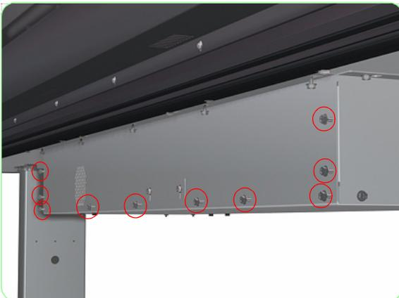
11. Remove ten screws that secure the Front Electronics Module Cover.
