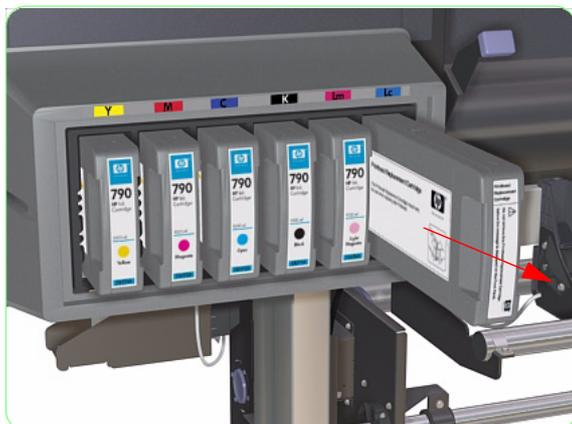
30. When this message is displayed on the Front Panel, remove the Printhead Replacement Cartridge.
