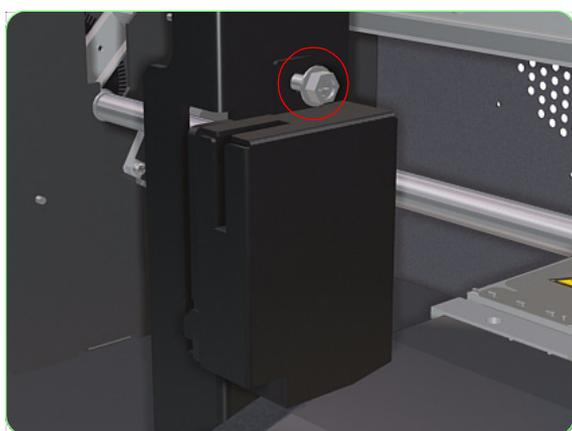
3. Remove one screw that secures the Window Sensor Cover to the Printer.
