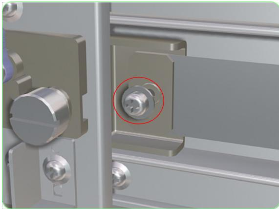
**13.** Remove one screw that secures the Belt to the right side of the Carriage Assembly.
