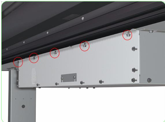
1. Loosen five screws that secure the top of the Front Electronics Module Cover.
