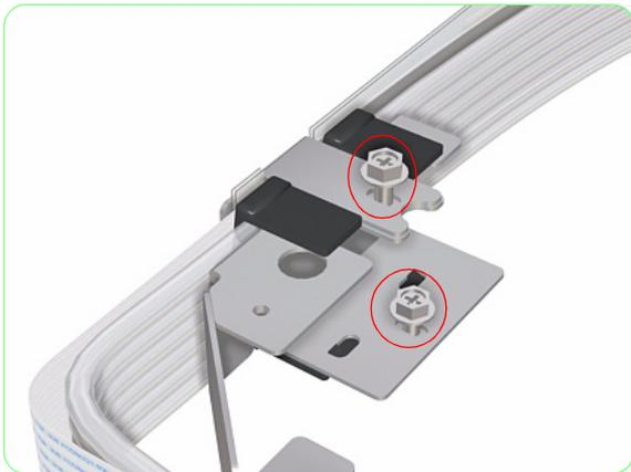
5. Secure the Metal Bracket with two screws.
