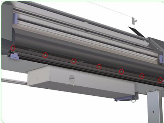
**2.** Remove seven screws from the bottom that secure the Front Heater to the Printer.
