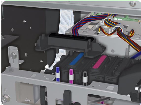
9. Remove the Valve Assembly from the Printer.
