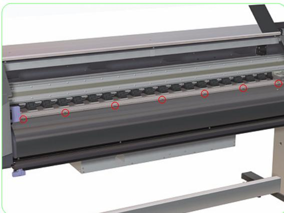
**3.** Remove seven screws from the top that secure the Front Heater to the Printer.
