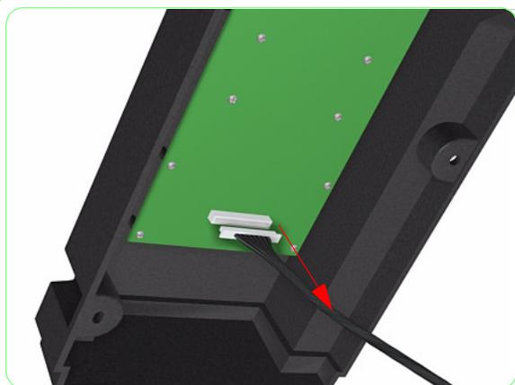
7. Disconnect the Cable from the Front Panel.
