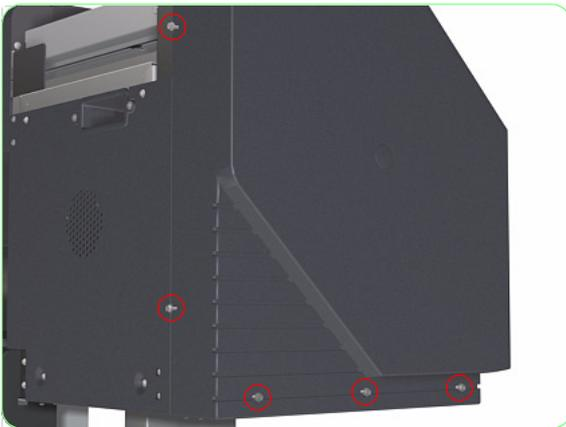
5. Remove five screws that secure the Left Side Cover to the Printer.
