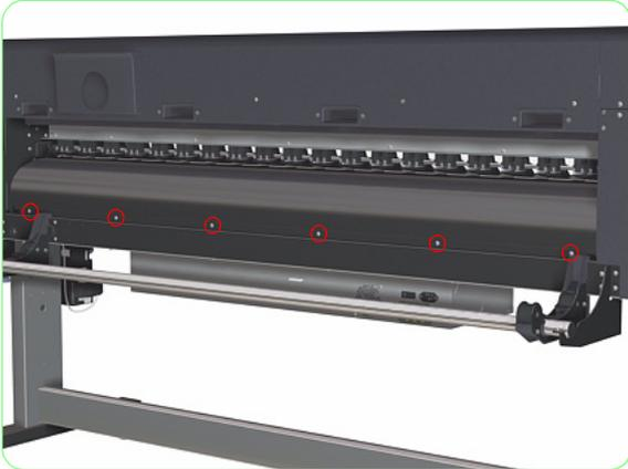
4. Pull out the Rear Heater slightly.
