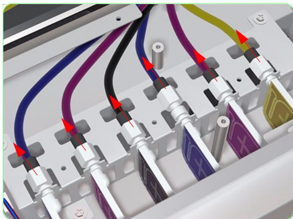
**29.** Disconnect the Ink Tubes from the Air Dampers.
