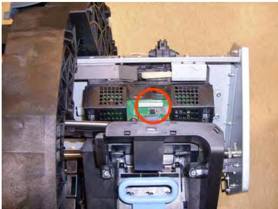
8. Remove the four T-15 screws that secure the Ink Supply Tubes to the Carriage Assembly.
