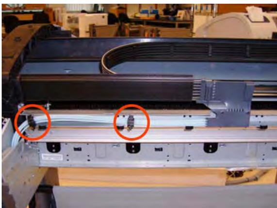
19. Remove two T-10 screws that secure the Left Side Plate of the Left Ink Supply Station.
