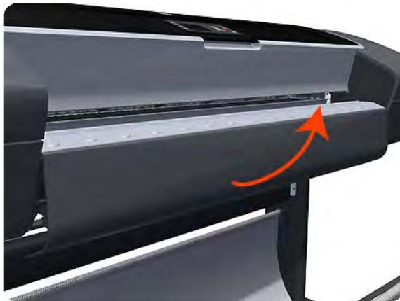
4. Unhook the Front Cover from the four attachments and remove it from the printer.
