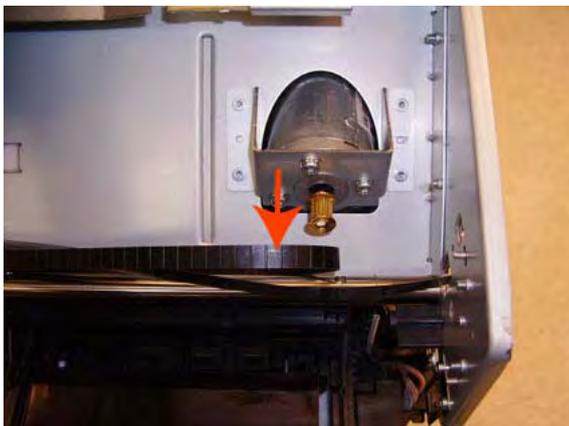
26. Remove the two T-10 screws that secure the Media Lever attachment plate.
