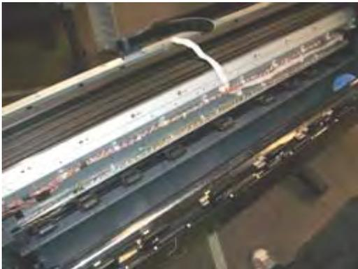
12. Keep the cable ties and screws to for reuse after replacing the cable.
