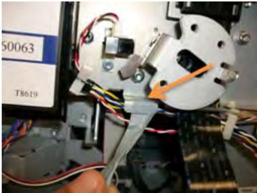
9. Remove the RFID tag support.
