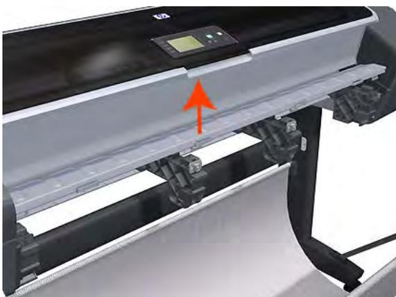
6. Slide the Media Output Assembly forwards out of the printer.
