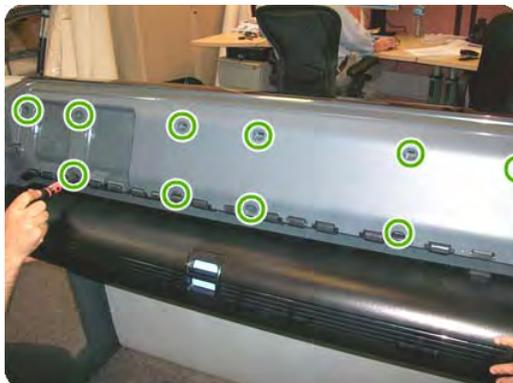
5. Remove the Rear Cover from the printer.
