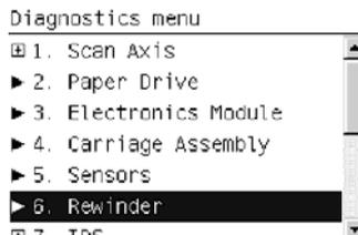
The printer will start the Open Loop, Rewinder Servo System, and Media Driver PWM tests.
