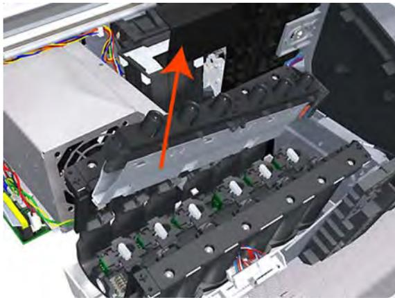
13. Carefully lift the Left Ink Supply Station enough so that you can rotate it counterclockwise to release the front attachment from the printer.
