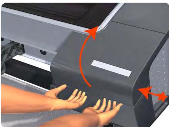
5. Remove one T-15 screw that secures the Right Cover to the printer (at the rear of the printer).
