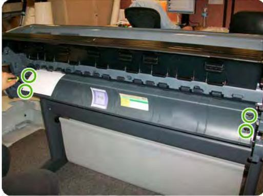
6. First extract the right side of the cleanout, as shown, and then the left side. Be careful with the paper sensor cable.
