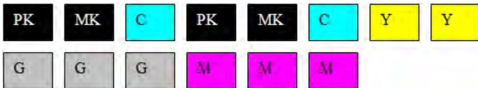
Once the printer has correctly printed and scanned the Printhead Alignment Diagnostic print, the Front Panel displays the results. The top row displays the printhead, and the left column displays the test.
