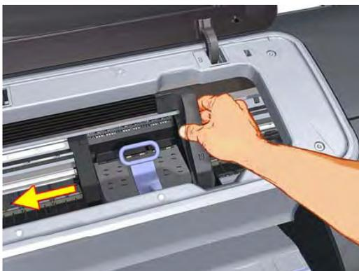
9. Clean the part of the encoder strip inside the Service Station by repeating steps 2 to 6.
