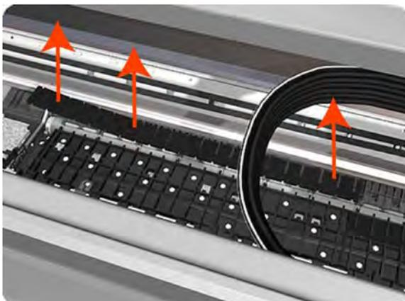
**NOTE:** When you reinstall the full bleed foams, take care to correctly seat them to avoid possible damage to the Carriage Assembly
