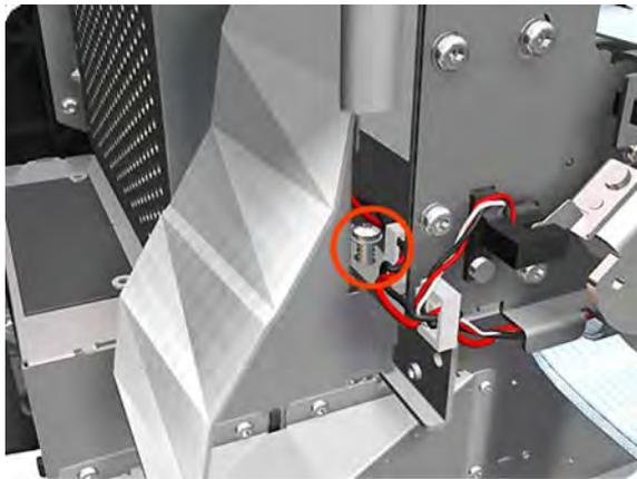
8. Remove two T-20 screws that secure the Electronics Module to the printer.
