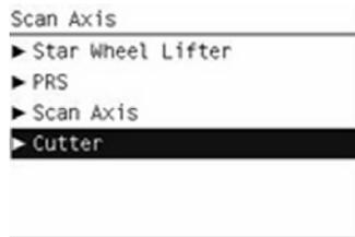
3. In the **Scan Axis** submenu, scroll to Cutter and press **OK** to start the test. The test prompts you to check that all paper is unloaded. Once the paper is unloaded, press **OK**.
