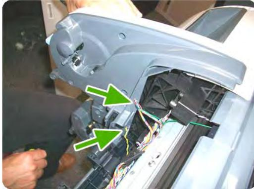
6. Disconnect the cable connector as shown.
