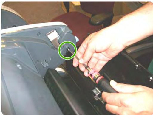
3. Remove the screw on the Roll Cover's right side that attaches to the Upper Right Roll Support.
