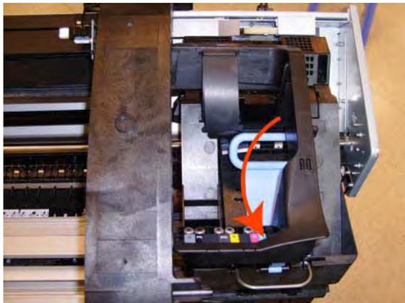
11. Carefully move the Ink Supply Tubes into the print path.
