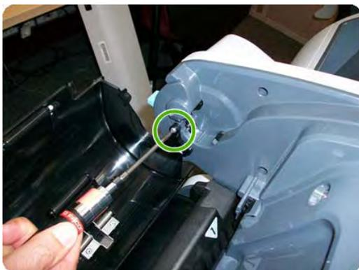
4. Remove the Roll Cover hinge from the Roll Left Support Pin.
