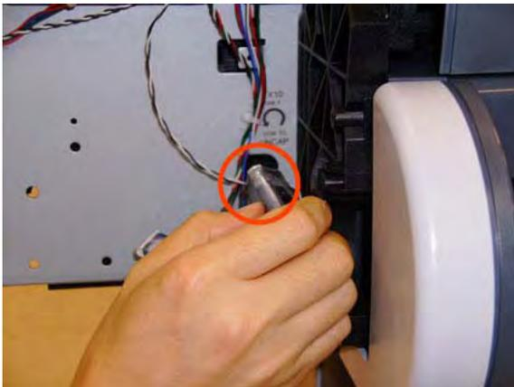
22. Push the Carriage Assembly into the print path.
