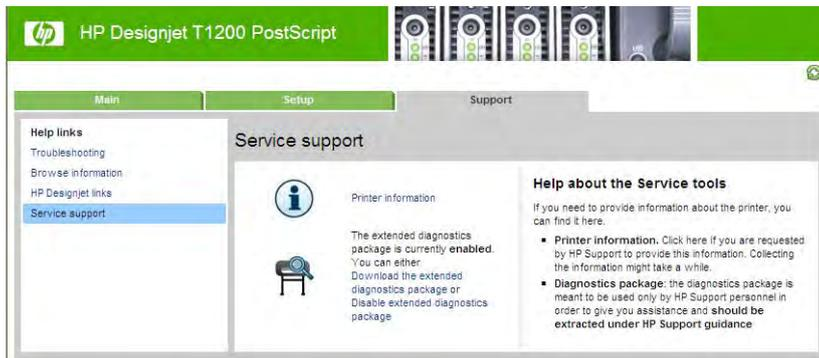
2. If the problem persists and is difficult to debug, try the extended diagnostics package. To enable the extended diagnostics package, click **Enable the extended diagnostics package**. The printer needs to be restarted after enabling or disabling the extended diagnostics package.
