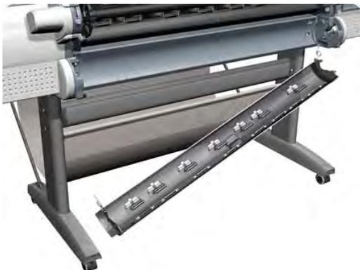
12. Hold the roll cover with one hand while unscrewing the other bi-stable spring from the printer.
