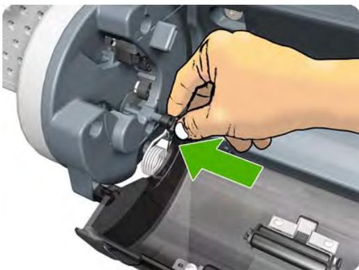
6. Insert the Lower Roll Cover left-side hinge into the Lower Left Roll Support pin.
