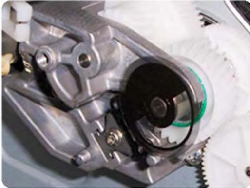
3. Press the encoder using the Media Advance Drive Adjustment Tool (reversed) so that it sticks to the roller.
