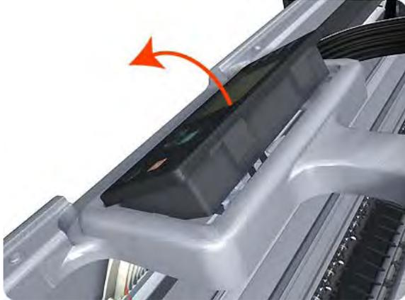
5. Disconnect the interface cable from the Front Panel.
