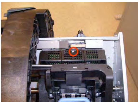
6. Remove the small cover of the Carriage PCA.
