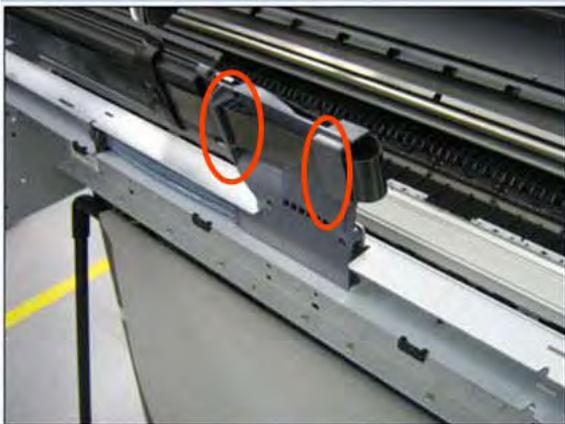
22. Remove the Trailing Cables from the printer.
