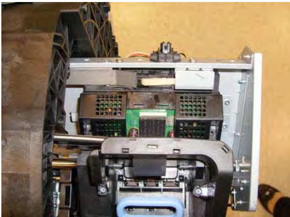
9. Disconnect the ribbon Trailing Cable from the Carriage PCA.
