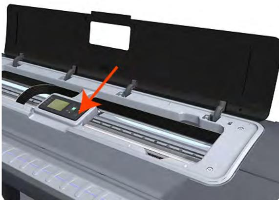
11. Lift the Window vertically out of the printer.
