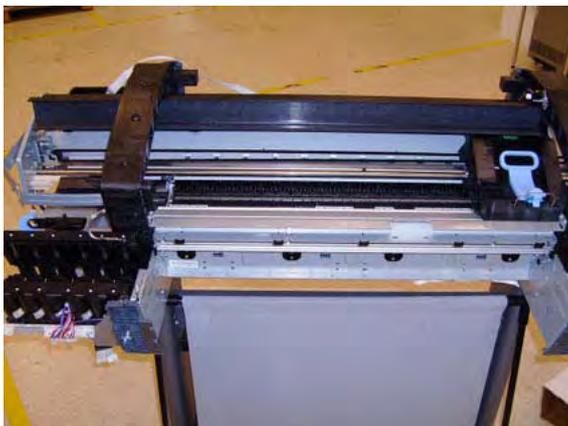
25. Carefully remove the Ink Supply Tubes from the assembly.
