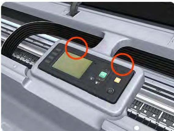
4. Rotate the front panel vertically.
