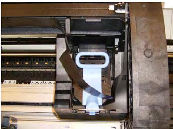
13. Slide the Trailing Cables out of the cable and tube holder.
