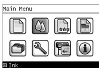
2. In the Ink Menu submenu, scroll to **Replace printheads** and press **OK**.
