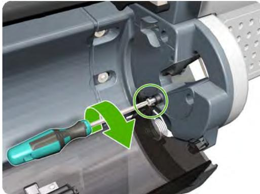
9. Close the Lower Roll Cover until the other end of the Bi-stable Screw is in front of the hole on the Lower Left Roll Support (if necessary, hold the Roll Cover for a moment with your head).
