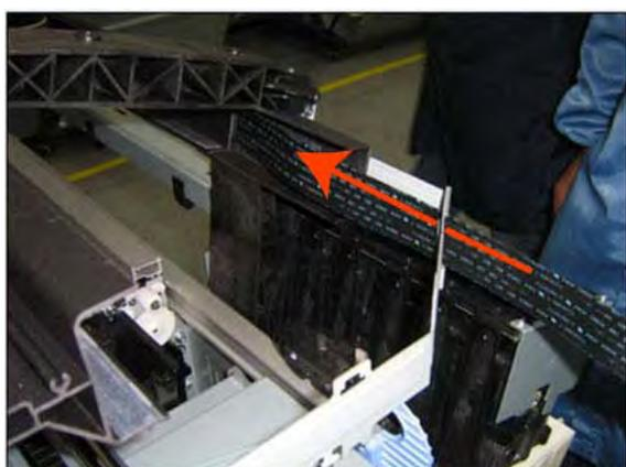
19. Pass the Trailing Cable through the slot.
