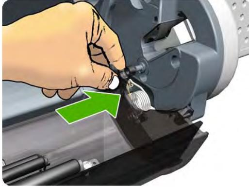
7. Screw the Lower Roll Cover to the Lower Right Roll Support.
