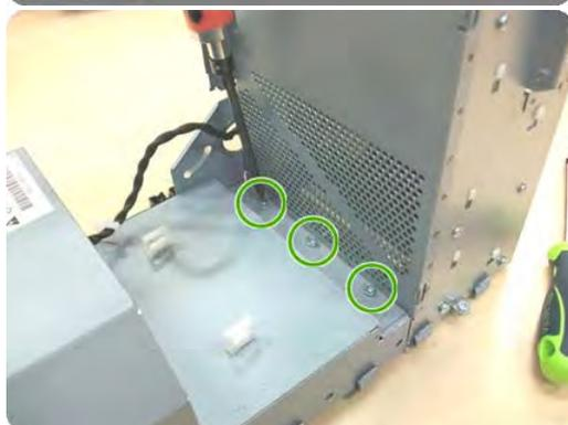
3. Remove the PSU module from the EE box base.
