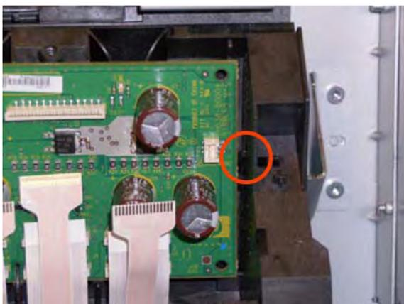
15. Remove the Carriage PCA from the carriage.
