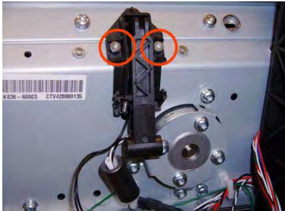
6. Remove the Pen to Paper Space (PPS) Solenoid from the printer.
