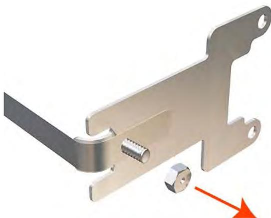
6. Remove the Encoder Strip Spring.
