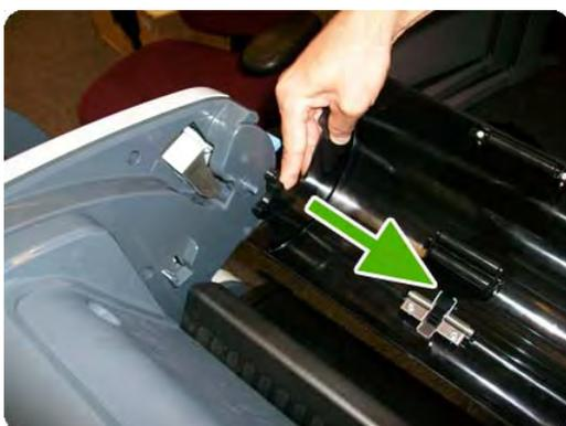
5. Remove the Roll Cover hinge from the Roll Right Support Pin.
