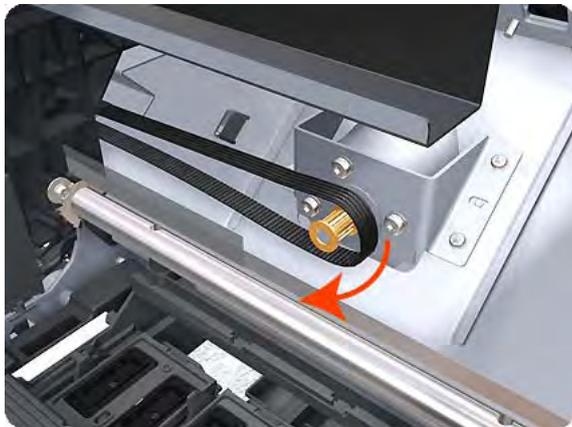
9. Remove three T-20 screws that secure the Scan-Axis Motor to the printer.
