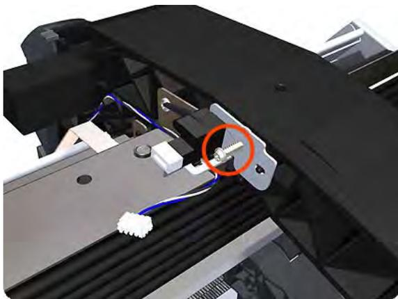
9. Remove the Window Position Sensor from the printer.
