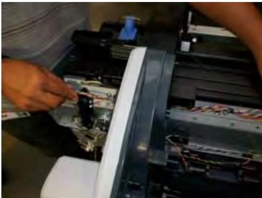
21. Back on the left side, detach the FP harness cable to leave space to detach the lower cable branch.
