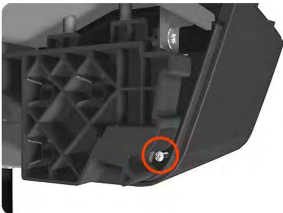
9. Remove one T-15 screw that secures the Right Cover to the printer.
