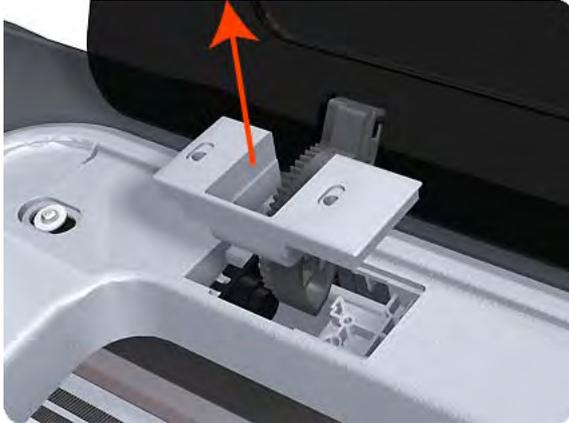
5. Remove the Damper Rotary from the Top Cover.
