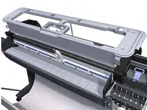
13. Unroute the Front Panel ribbon cable from the two cable clamps on the bottom surface of the Top Cover.
