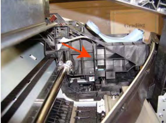
20. Remove one T-10 screw that secures the Line Sensor to the Carriage Assembly.
