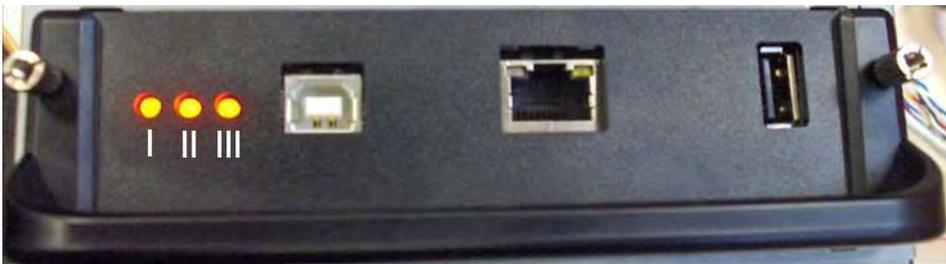
Use the following table to interpret the LEDs and find the source of the problem. Remember that you should read these LEDs when you push the **Power** button.
