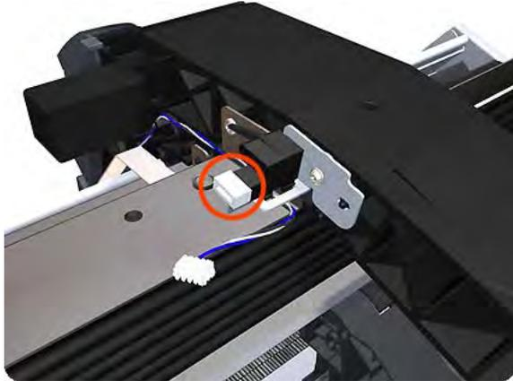
8. Remove one T-15 screw that secures the Window Position Sensor to the printer.
