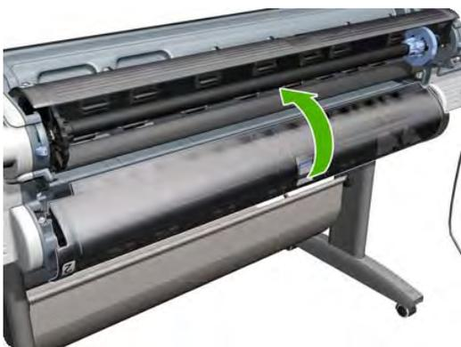
10. Screw the left pre-loaded Bi-stable Spring to the Lower Left Roll Support. Do not let the cover close completely.
