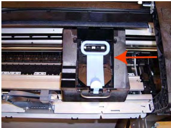
15. Remove the top T-15 screw that secures Ink Supply Tubes guide to the printer.
