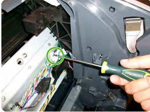
5. Unplug the Upper Left Roll Support, taking care not to damage the cables. Detach all cables from the Roll Support.
