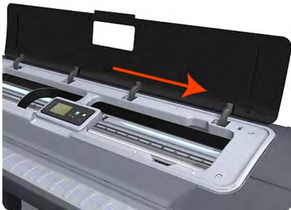
10. Pull the Window towards the front to disengage the hinges.
