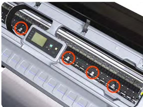
7. Use a flat-bladed screwdriver to unclip the left Print Zone Overdrive retaining clip and rotate the clip vertically.
