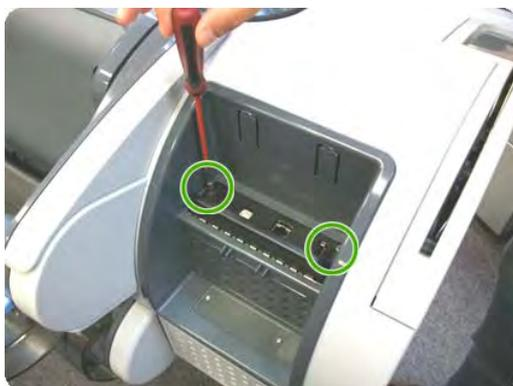
3. Lift the Formatter out of the printer.
