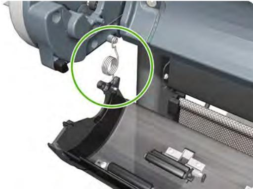
7. Detach the roll cover from the printer on the right-hand side.
