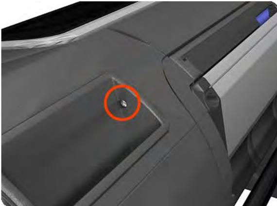
8. Remove one T-15 screw that secures the Right Cover to the printer (accessible under the Front Cover).
