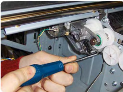
3. Loosen the encoder sensor adjustment screw.
