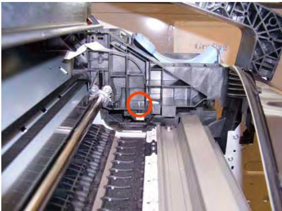
21. Remove the Line Sensor from Carriage Assembly.
