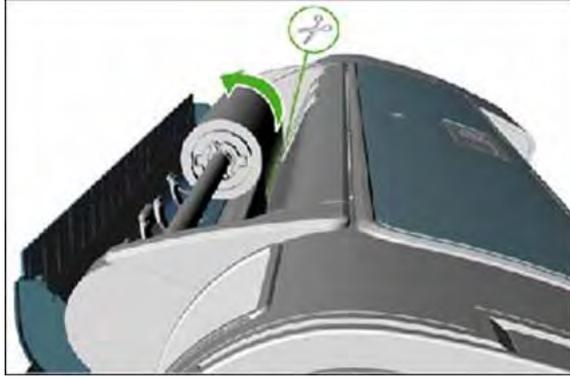
3. Rewind and remove the lower roll in the same way.
