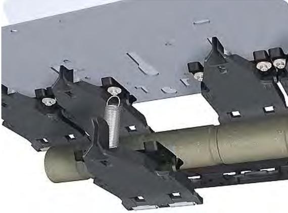
3. Hook the spring of the Pinchwheel Assembly you are installing with the Pinchwheel Insertion Tool.
