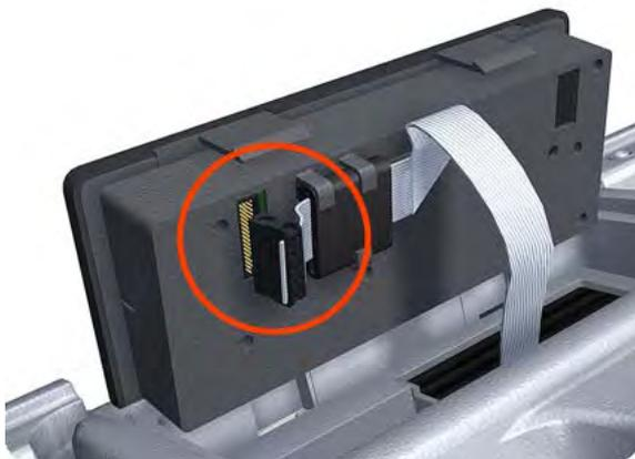
6. Push in the clip that prevents the Ferrite Core from being removed.
