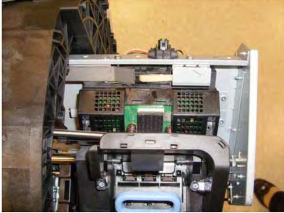
7. Disconnect the ribbon Trailing Cable from the Carriage PCA.
