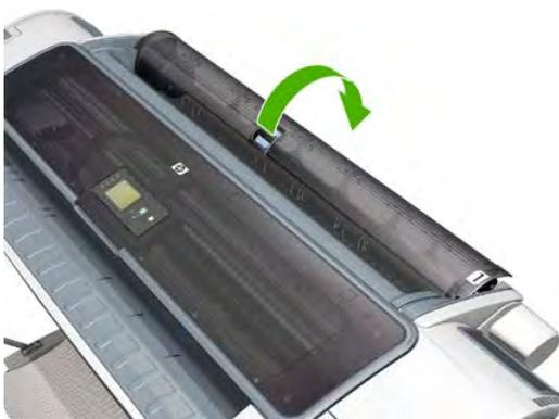
2. Remove the spindle.
