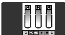
8. Remove **all** the Setup Printheads from the Carriage and install the previously removed Printheads.
