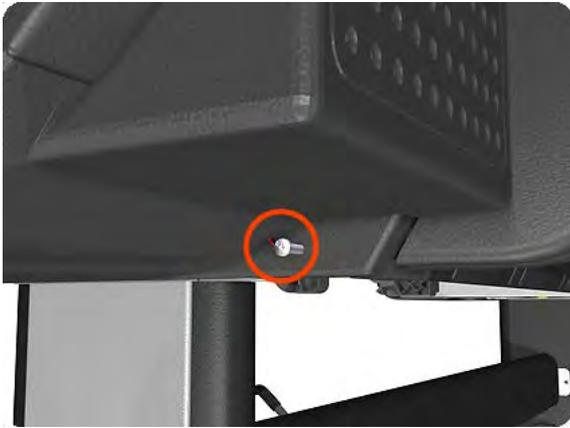
7. Remove one T-15 screw that secures the Right Cover to the printer (at the rear of the printer).
