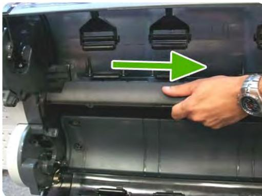
6. Move the right side of the converger in the direction of the arrow, then remove the whole converger from the printer.
