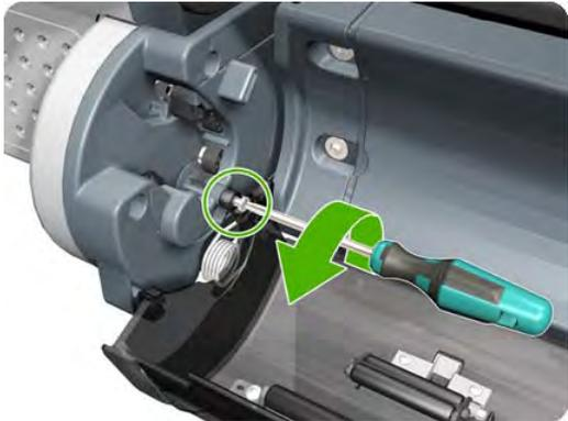
4. Remove the screw connecting the roll cover to the printer on the right.
