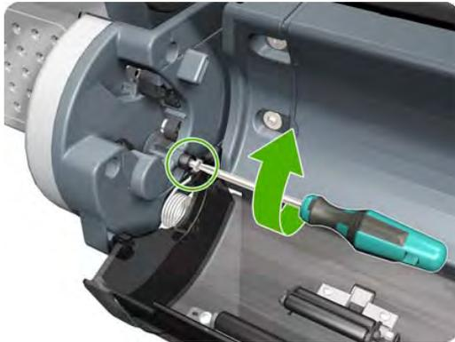
8. Screw the Lower Roll Cover to the Lower Left Roll Support.
