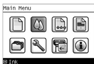
2. In the Ink Menu submenu, scroll to **Replace ink cartridges** and press **OK**.
