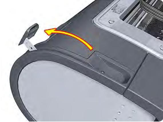
7. Use the Pinchwheel Insertion Tool to remove the spring from the attachment on the printer.
