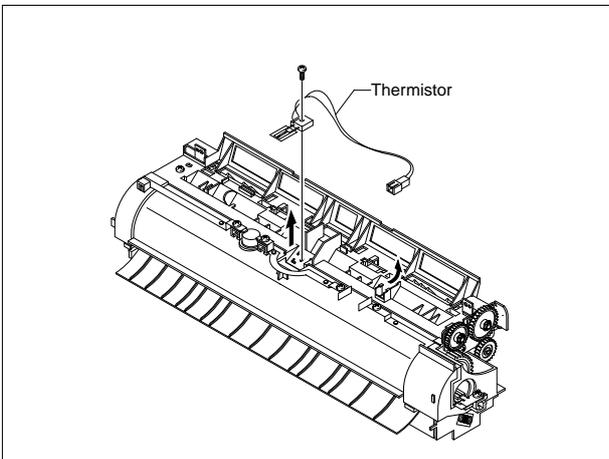
5. Remove two screws and take the Halogen Lamp out of the Heat Roller.
