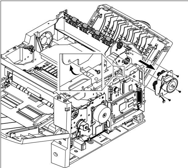
4. Remove two screws and take out the Exit Motor.
