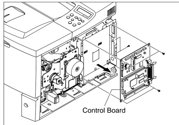
5. Remove four screws and take out the Control Board Bracket.
