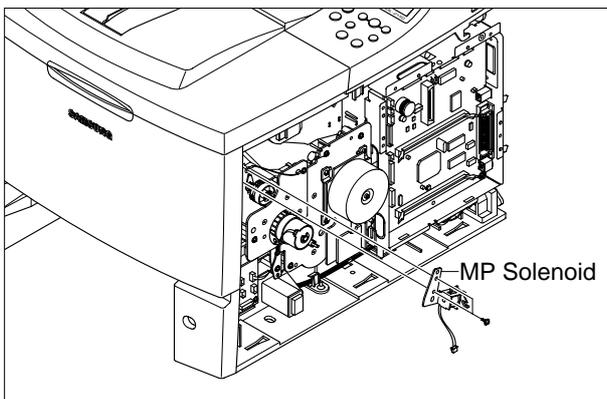
4. Remove two screws and take out the Main Solenoid.
