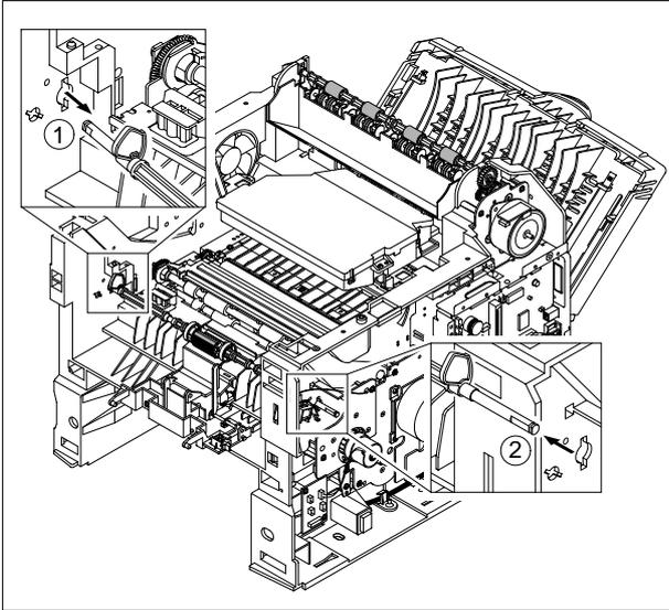
7. Push the idles toward the ends of shaft then take out the Housing as shown below.
