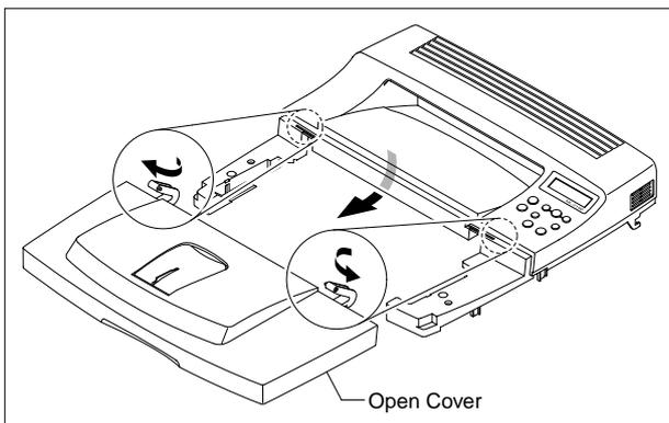
4. Release the lock as shown below and lift up the Sensor Cap.
