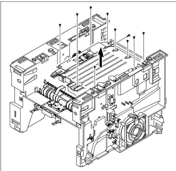
4. Unplug all of the connectors from the Engine Board. Then take out the Engine Shield Ass'y.
