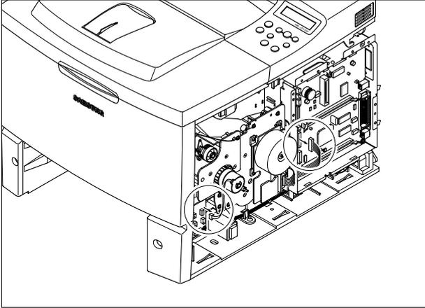
3. Remove the e-ring and take out the Clutch.
