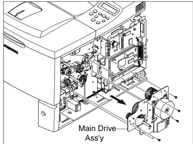
5. When separating the Main Motor ass'y, disconnect the connector from the Main PBA, remove 4 screws, and then remove the Main Motor ass'y.
