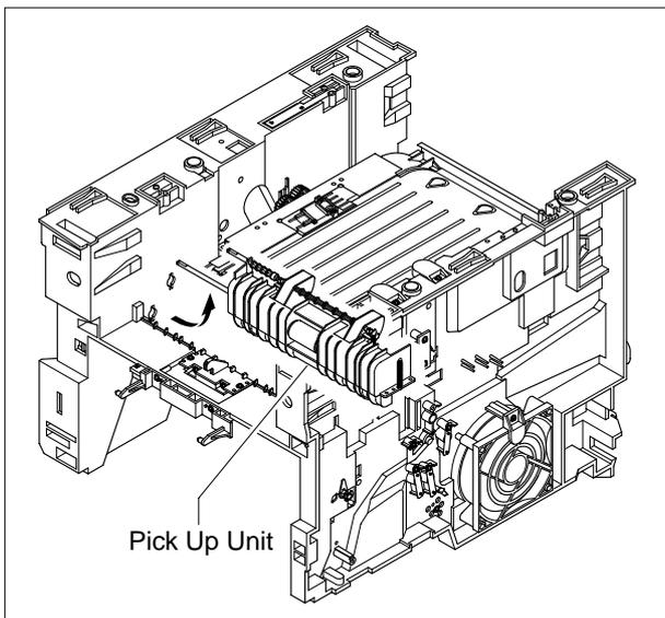
10. Remove the Pick Up Ass'y as shown below.
