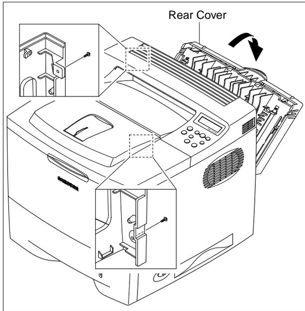
3. Remove two screws and take out the LH Cover.
