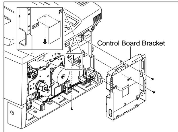
**NOTICE :** One screw among the screws is locked on the Engine Shield.(Refer to 5.25.3)
