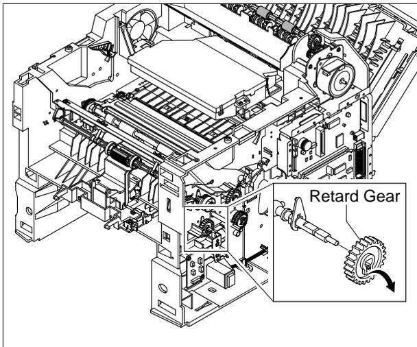
4. Remove the lock equipment and rotate the Bearing as shown below.
