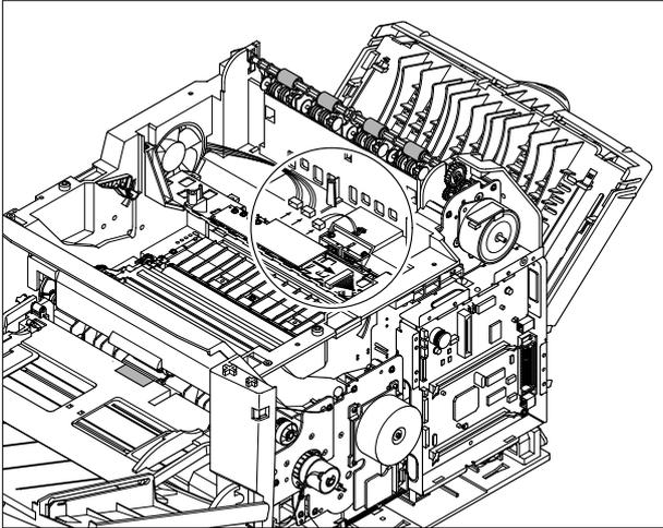
3. Remove 4 screws and take out the Toner Sensor Board.
