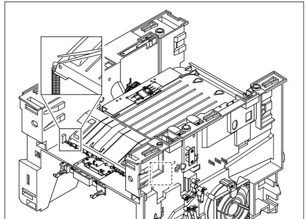
5. Release the lock as shown below and lift up the Stopper.
