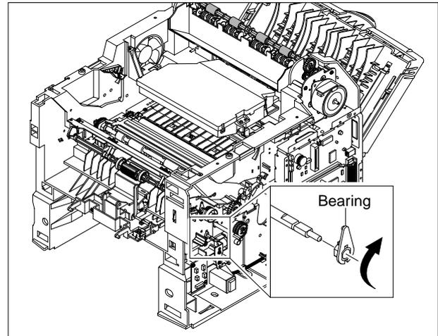
5. Slide the shaft (gear side) to the left side as shown in the picture. Next, left side of the shaft to the right side. Be careful not to mass up with the Holder Pad ass'y.
