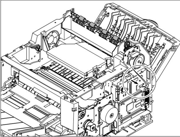
3. Remove three screws and take out the Exit Driver Ass'y.
