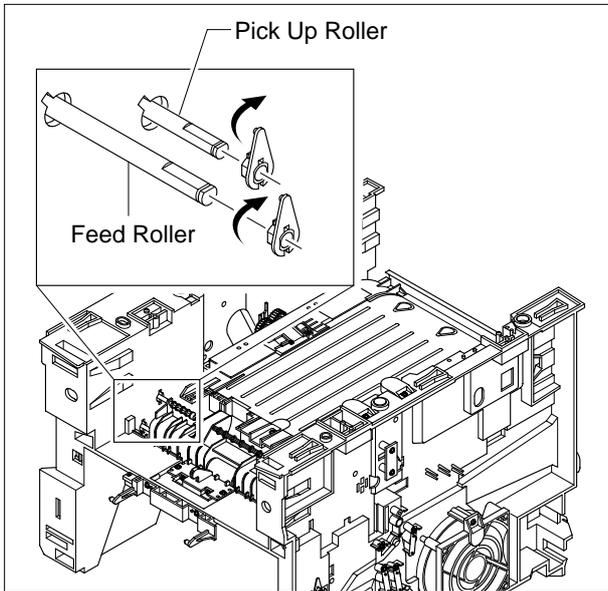
9. Remove the Feed Ass'y as shown below.
