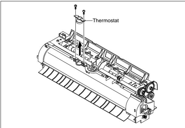
4. Remove one screw, and then take out the Thermistor from the Fuser Ass'y.
