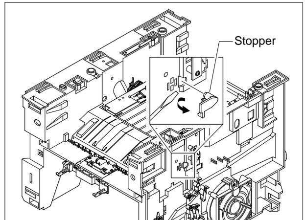
6. Lift ICU Shield out in the direction of arrow as shown below.
