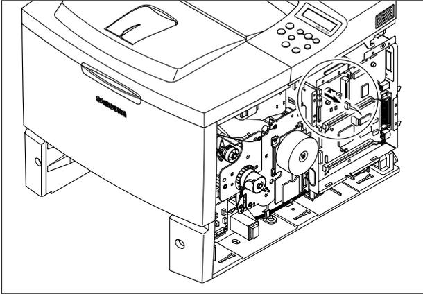
3. Remove one screw for taking out the Stopper, and then take out the DC Fan.
