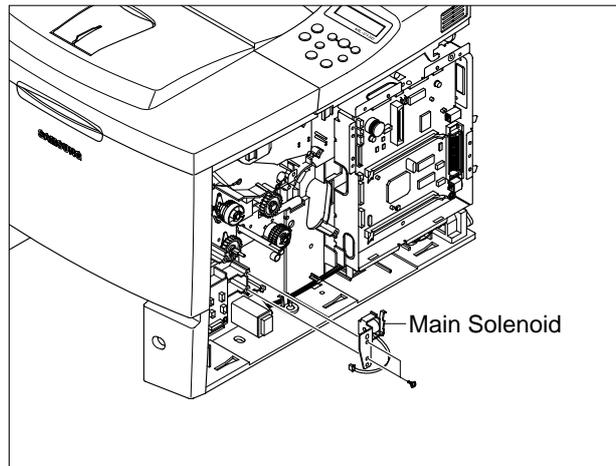
**NOTICE :** It is not necessary to disassemble the Main Drive Ass'y to remove the MP Solenoid
