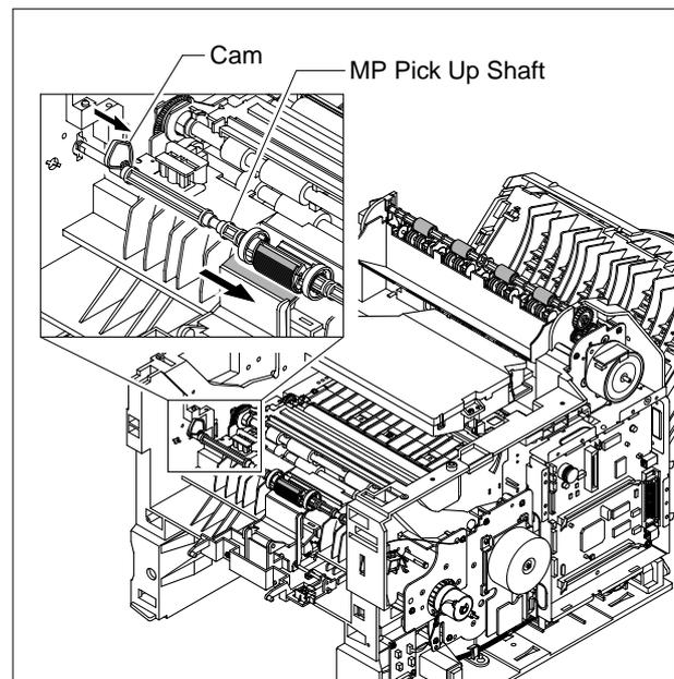
6. First lift the left side of the Shaft and then remove the Shaft.
