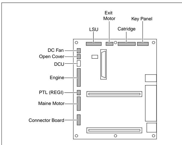
4. Remove six screws and take out the Control Board.
