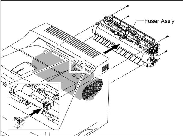
3. Remove two screws and take the Thermostat out of the Fuser Ass'y.
