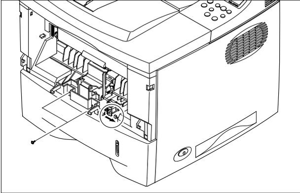
3. Remove the photo interrupter and the MP Actuator as shown below.
