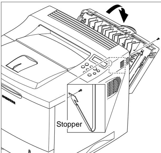
2. Remove the Rear Cover in the direction of arrow.
