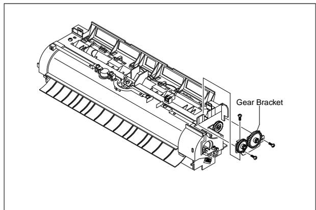
7. Remove two screws and divide the Fuser into two parts.
