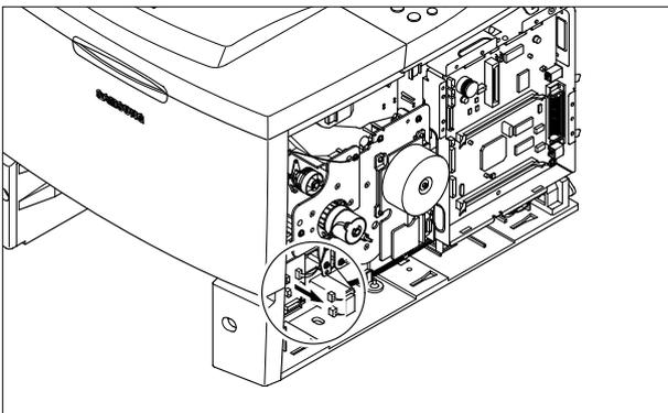
3. Remove two screws and take out the MP Solenoid.
