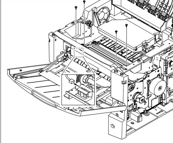
3. Release the lock as shown below and lift up the Gear Cap.
