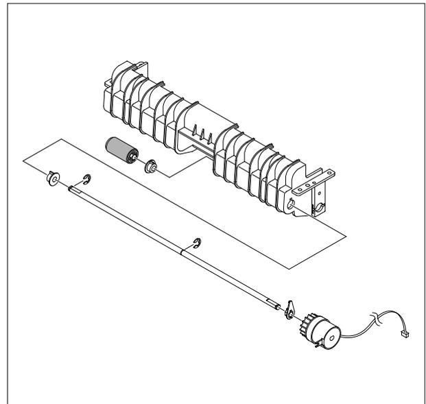
8. Remove four screws and lift the Pick Up Unit out in the direction of the arrow as shown below.
