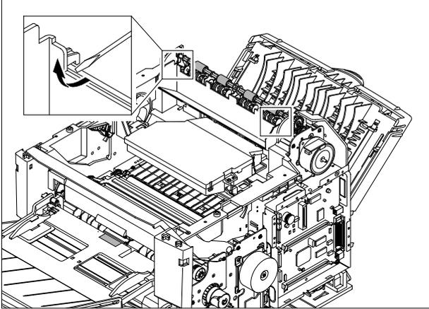
3. Remove the Exit Roller Rack in the direction of arrow.
