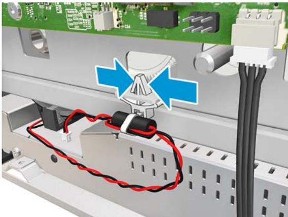
9. Remove the Carriage Motor Cable.
