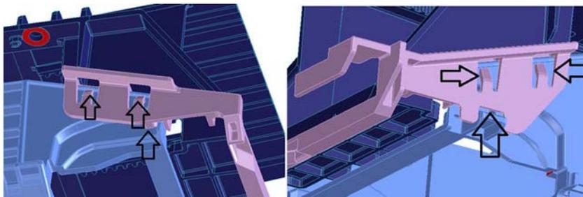
2. If the cutter bridge is well assembled and the cutter is not activated while cutting, the cutter assembly should be changed..
