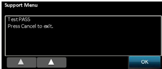
5. If any key does not work, the diagnostic will not pass to the next key, and will stay always in the screen of the failing key therefore the front panel should be changed, see [Front Panel on page 165](#). To recover the printer, if this occurs the printer should be restarted by switching it off and on with the power key.
