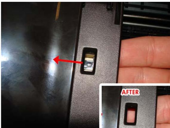
4. Take out the Top Cover Sensor, being careful not to damage the flat cable.
