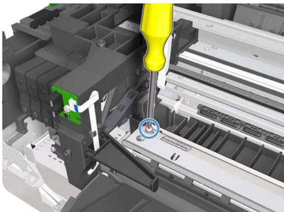
9. Remove one T-10 screw on the right side of the Starwheel Assembly.
