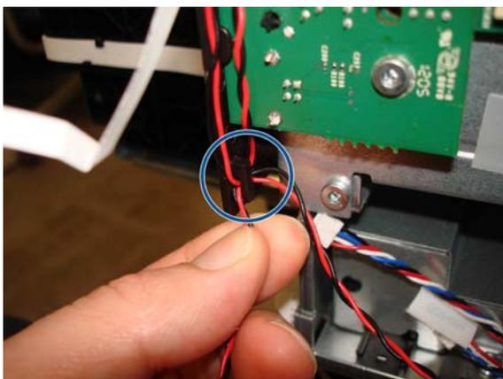
**10.** Unhook the two cables from the top hooks.
