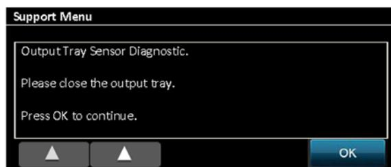
4. Close the Output Tray and press **OK**. If the sensor is not damaged then you will see:
