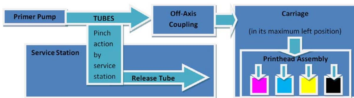
**NOTE:** There is no pressure sensor in the system. The Prime Pump operates at a certain time to reach a specific pressure level, the system is depressurized by releasing the pinching of the release tube in the Service Station (by moving the service station).
