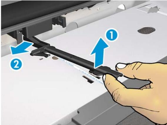
7. Press the retaining clips of the Out-Of-Paper Sensor Assembly.
