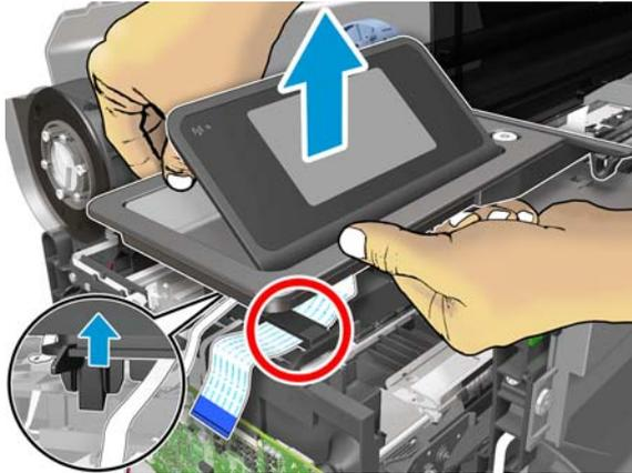
**17.** Remove the flat cable from the ferrite.
