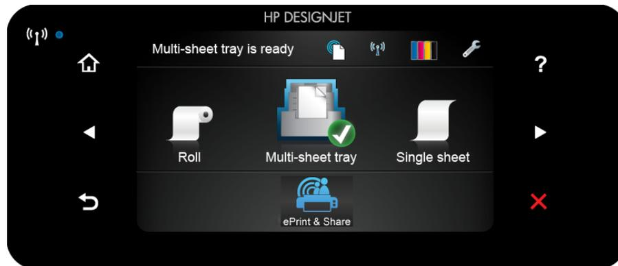
The front panel has a large central area to display dynamic information and icons. On the left and right sides you can see up to six fixed icons at different times. Normally they are not all displayed at the same time.
