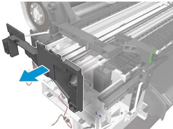
**23.** Pull the Left Bearing to unclip it from the hole (1), then rotate it (2).
