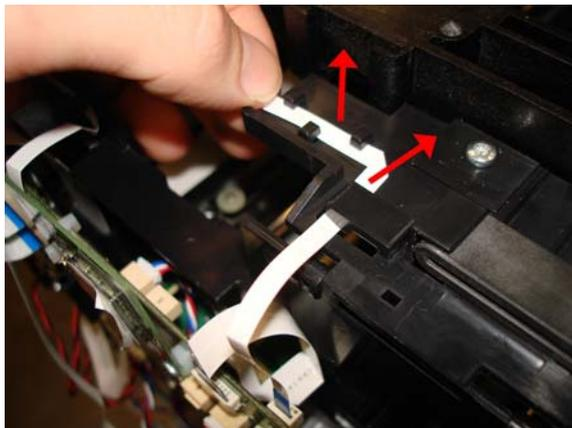
9. Disconnect the flat cable (Top Door Sensor FFC).
