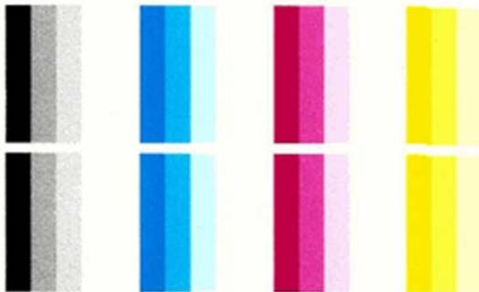
If any of the colored blocks in Test Pattern 2 show white lines, or are faded or missing completely, follow these steps to clean the printhead.
