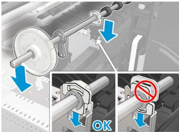
2. Make sure the Middle Bearing is mounted correctly.
