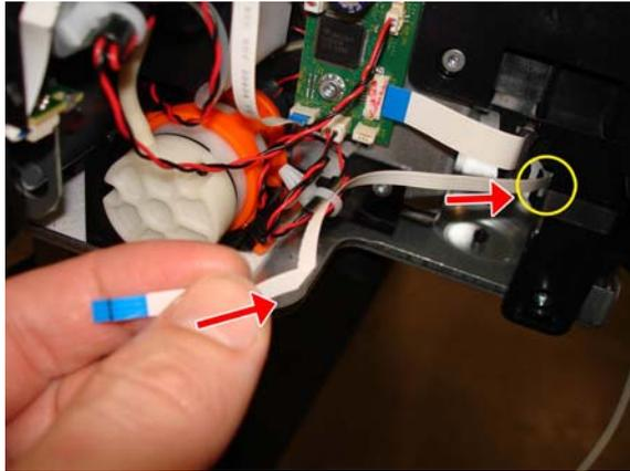
10. Remove the Out-Of-Paper Sensor Cable.
