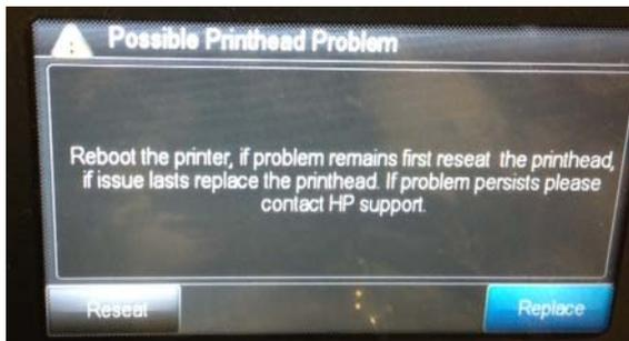
The printer is unable to determine whether the error is caused by a real hardware failure or which part may be failing (possible candidates: ink cartridges, Prime Pump, Carriage Assembly, Trailing Cable).
