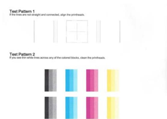
2. If the lines in Test Pattern 1 are not straight and connected, follow these steps to align the printer:
