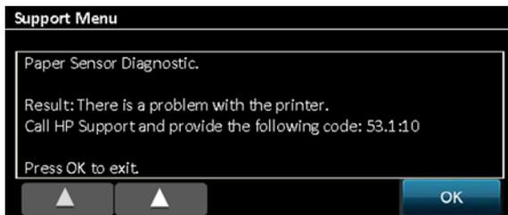
6. Replace the OOP sensor, see [Out-Of-Paper Sensor on page 281](#).
