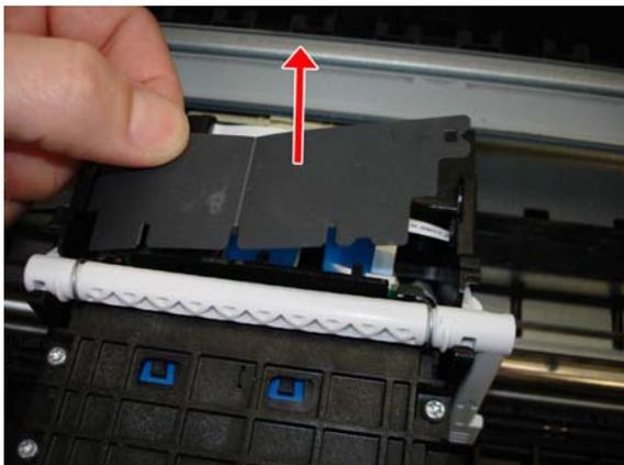
**10.** Unclip and remove the strain relief.
