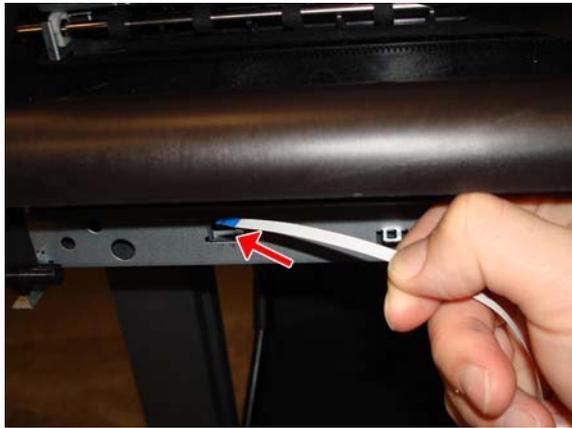
2. Pass the Output Tray Extender Sensor Cable through the hole of the left arch. **Important:** The blue color should be facing you.
