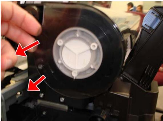
10. Unclip and detach the right side of the Roll Cover, bending it carefully.
