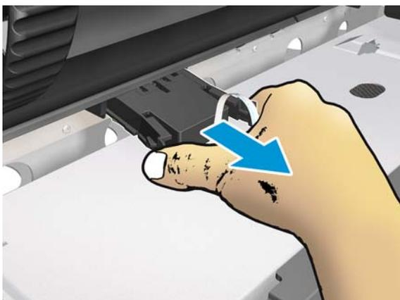
9. Turn over the Out-Of-Paper Sensor Assembly to get better access to the connector.
