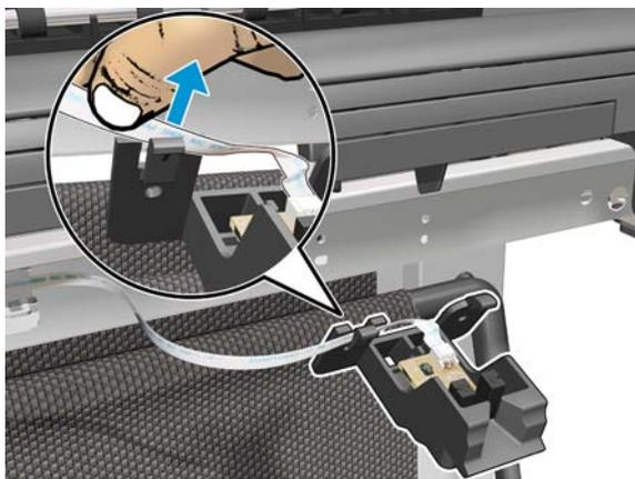
7. Disconnect the flat cable (Output Tray FFC).
