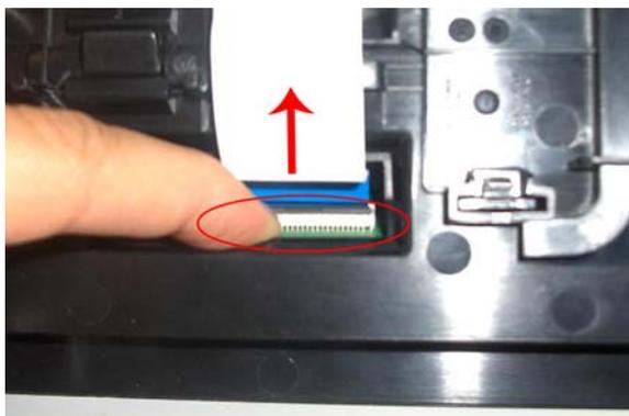
5. Remove the Front Panel FFC from its assembly by pushing it up.
