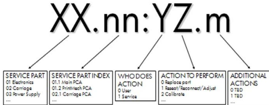
The two first fields before the (:) are the service part and the service index (if there is more than one, as in PCAs or motors). For call agents and service engineers the most important parts to know are the fields **WHO DOES THE ACTION** and **ACTION TO PERFORM**. These two fields can give guidance as to the most appropriate course of action if this error code is displayed.
