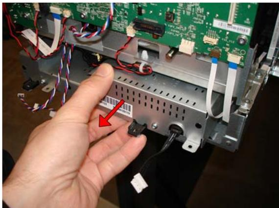
10. Remove the Power Supply from the front.
