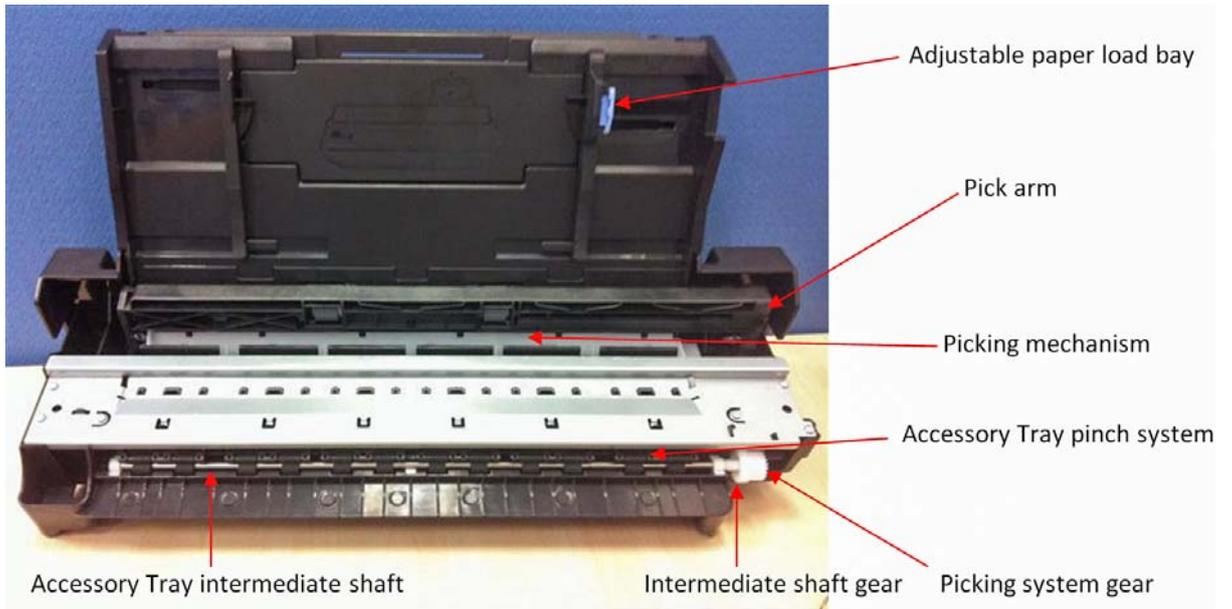
The Right Gear module has two main functions. It contains the motor encoder and gear drive system for the picking mechanism, and it contains the gear train system to transmit the movement from the drive roller to the accessory tray.
