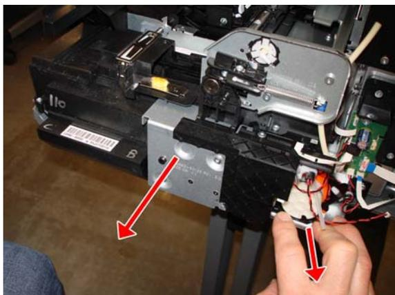
**17.** If, while you are sliding out the Service Station, there is an interaction with the metallic bracket, then you should push down the Service Station.
