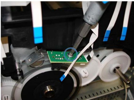
**11.** Release the PCA from the pin or locator.
