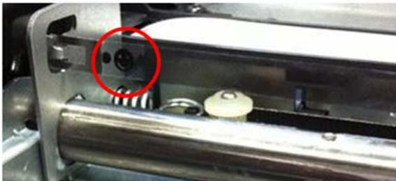
**NOTE:** Due to the proximity of the encoder strip to the greased sliding rod, it is easy to dirty the strip with grease when performing any repair operation in the area. Please clean any grease from the encoder strip if necessary. A dry cloth can be used for this purpose, to prevent any deformation or strain on the encoder strip while performing the cleaning.
