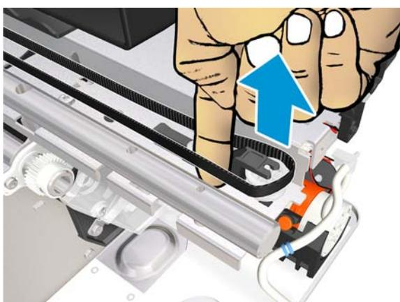
**20.** Remove the Carriage Belt from the end pulley.
