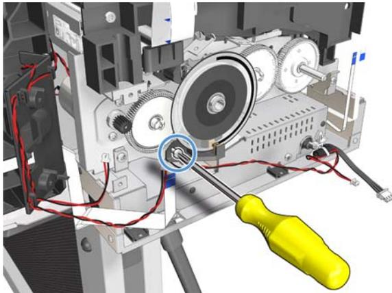
8. Remove the Holder Brush Feed Shaft.
