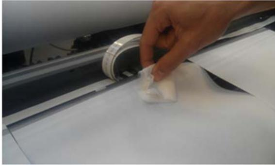
6. Move the Carriage towards the center of the printer and clean the remaining portion of the strip.
