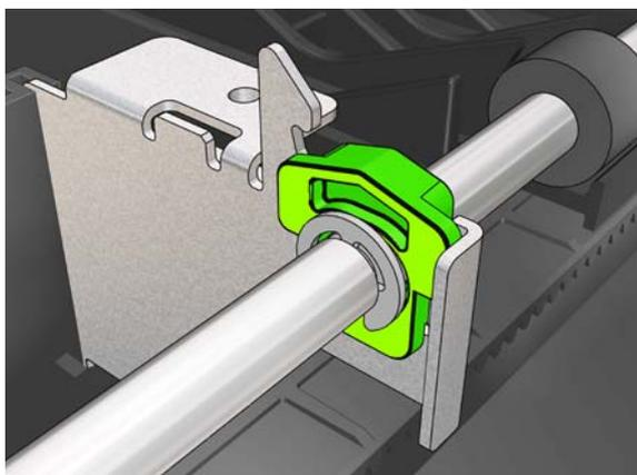
3. Put the Left Bearing in this position to mount to the left bracket.
