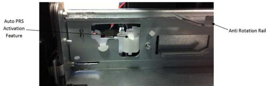
Auto-PRS feature located on the left-hand side of the scan axis.
