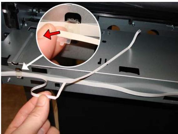
8. Disconnect the Out-Of-Paper Sensor Cable from the Bundle Board.
