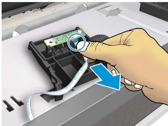
11. Remove the Out-Of-Paper Sensor Assembly.
