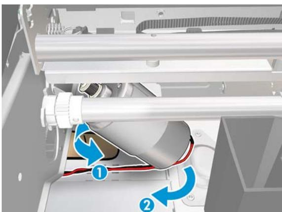
**14.** Remove the Carriage Motor.
