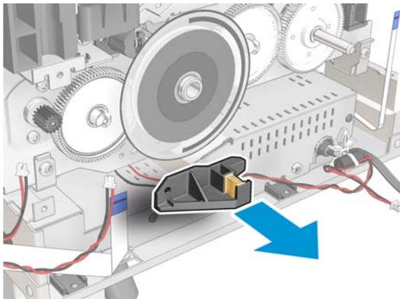
9. **IMPORTANT:** Do not remove the Encoder Disk without checking the position of the black reference mark.
