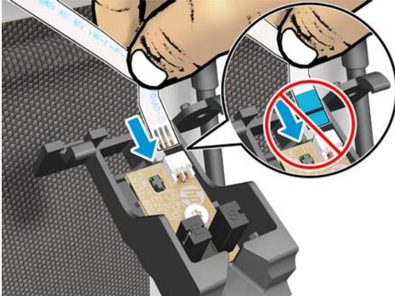
2. Attach the two pins of the Output Tray Sensor to the front of the printer.
