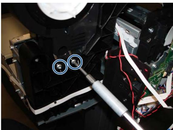
**17.** Rotate the Cover Left Roll Support to the left a little to detach it from the bracket.
