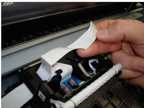
**13.** Slide out the Trailing Cable carefully through the hole.
