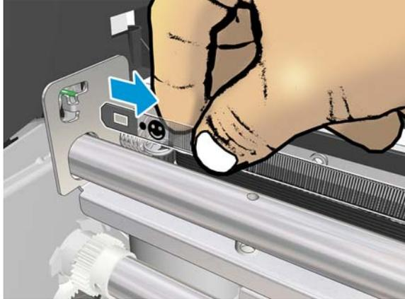
10. Slide the Encoder Strip carefully from the right side, and remove it.
