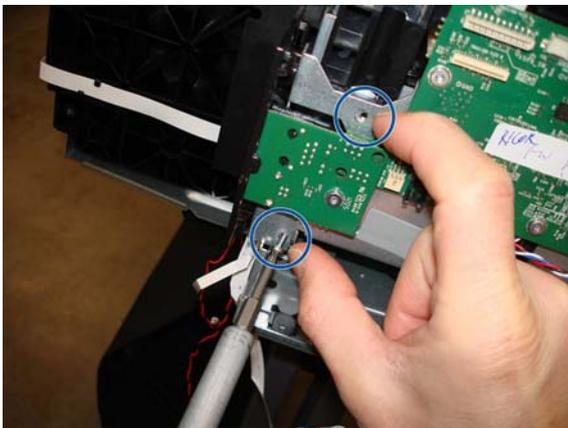
3. Push in the bracket of the Main PCA to align the two holes and screw the two screws without damaging them.
