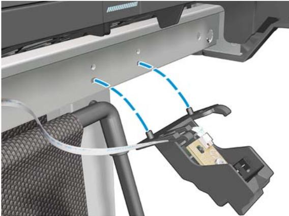
3. Make sure the Output Tray Sensor is mounted correctly.
