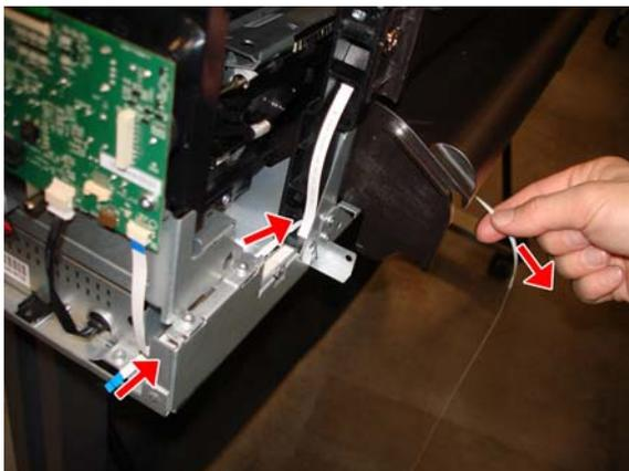
10. Remove the Output Tray Extender Sensor Cable.
