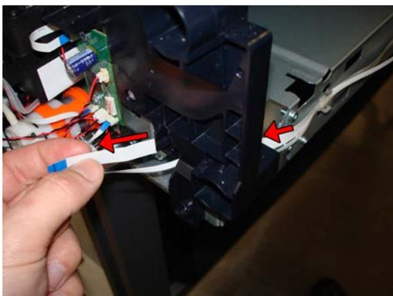
5. Re-install the Bundle FFC in exactly the same place where the ferrite was.
