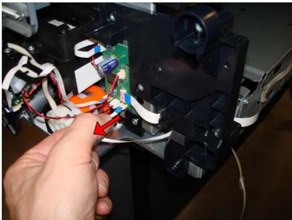
9. Unroute the Out-Of-Paper Sensor Cable through the hook.
