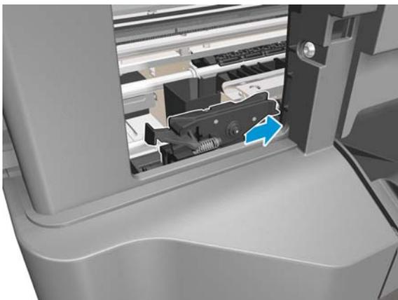
4. Unclip the flange of the Left Spittoon (1). Maintain it in the unclipped position and slide it up (2).
