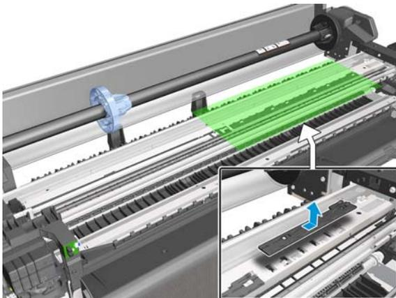
If the damaged Pinchwheels are in the zone indicated in green below, continue with the next steps.
