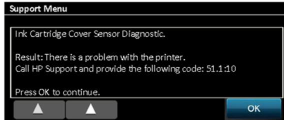
6. If there is a failure, replace the Ink Cartridge Cover Sensor PCA, see [Ink Cartridge Cover PCA Assembly on page 198](#).
