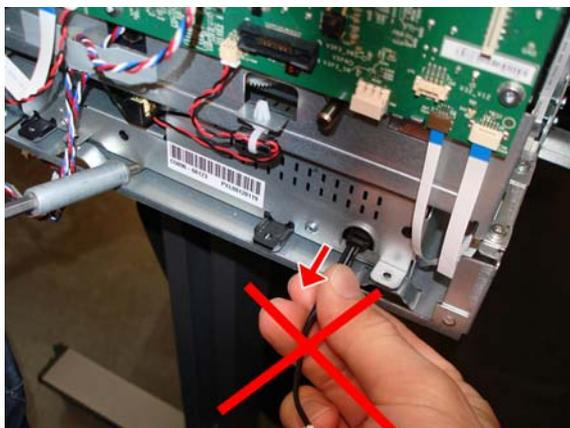
9. Slide out the Power Supply carefully.
