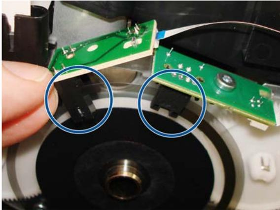
2. When connecting the cables to the PCAs, make sure that the blue side of the flat cables is facing up.
