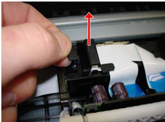
**11.** Disconnect the Trailing Cable by pulling the blue plastic.
