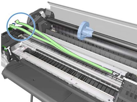
**18.** Disconnect the two parts of the Trailing Cable.
