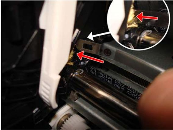
4. The Encoder Strip should go out through the other side of the Carriage as shown.
