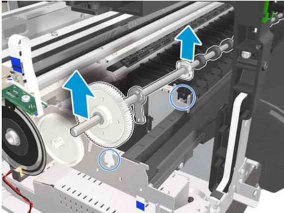
**26.** Slide the Output Shaft to the left to release it from the hole.
