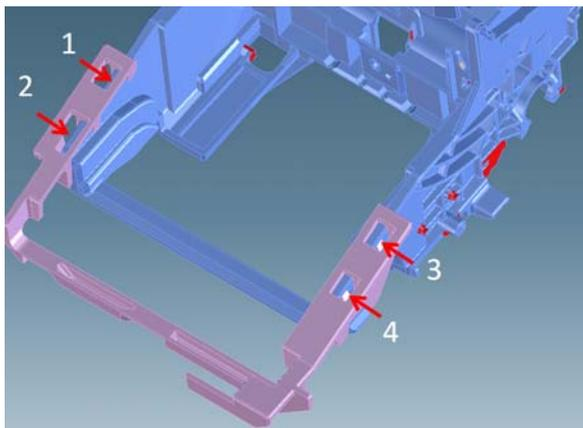
2. The Cutter Bridge is designed to fit over features of the Carriage.
