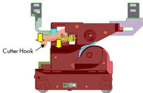
Left feature of the cutter bridge pushes down the cutter hook
