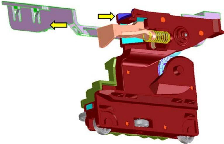
2. Move-away action: the Cutter Hook deactivates from the bridge by passing in front of it.
