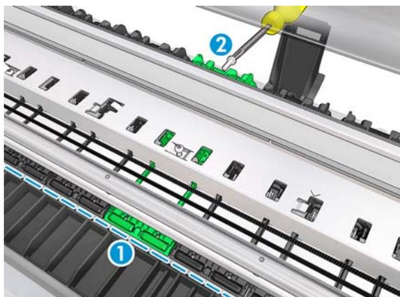
2. Attach the spring to the hook by pushing with the tool provided.
