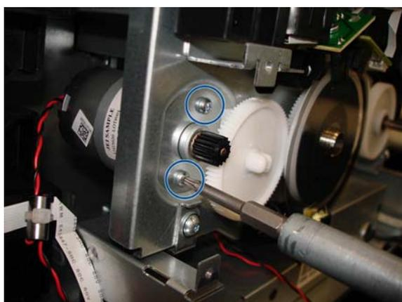
7. Slide the Paper Motor inwards, and hold it with a finger to stop it falling down.
