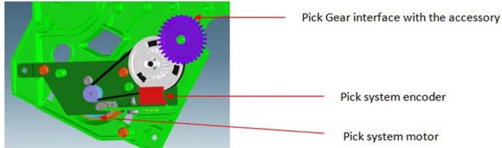
The Multi-Sheet Tray pick drive assembly is mounted in the right side gear module. The assembly contains a DC motor and pinion, belt, cluster pulley, and gear. An encoder (not shown, but it is located in front of the white gear shown in the picture) is read by the encoder sensor (in red in the picture) to servo-control the pick drive.
