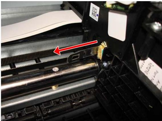
5. The right end of the Encoder Strip must have the triangle in the position as shown below.
