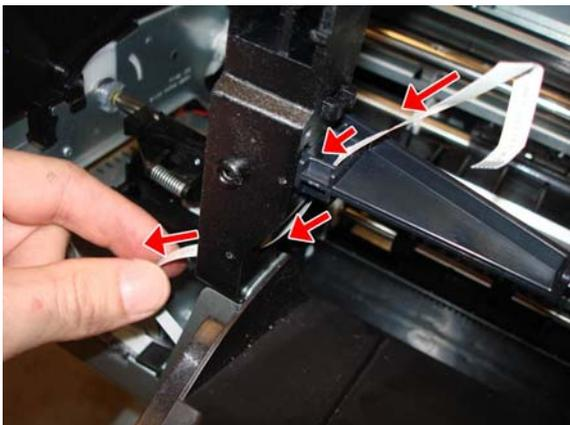
3. Be sure the Ink Cartridge Cover PCA Cable is free as shown.
