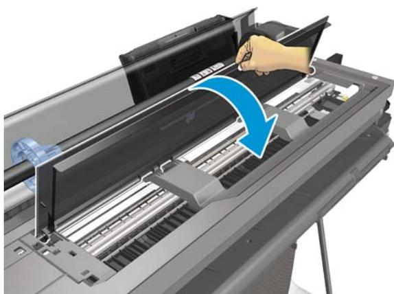
**10.** Ensure that the flat cable shown here is disconnected.
