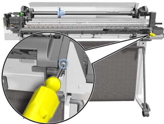
**18.** Remove the Output Platen.
