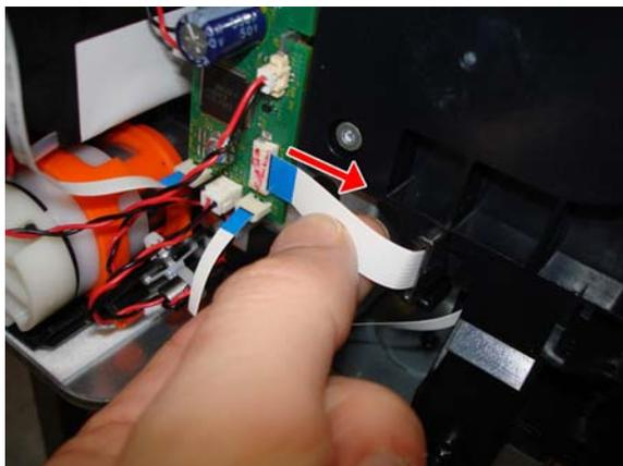
8. Unclip the two locators FFC, by first pushing up and pushing out.
