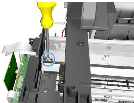
**14.** Unclip the trailing cable retainer clip shown here (1) and slide it to the right (2).
