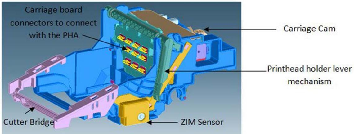
The Carriage holds all the necessary interface electronics for the main board to interact with the printhead via the trailing cables. A set of spring-loaded connectors are the main interface Carriage-printhead.
