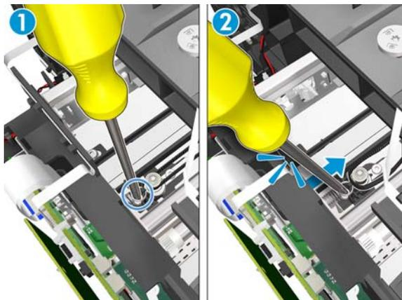
11. Remove the Carriage Belt from the pulley.
