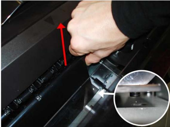
8. Slide the Upper-Roll Paper Guide to the left to release both pins from the holes.
