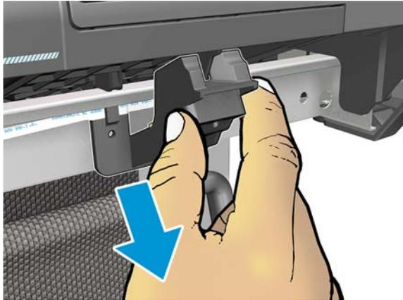
6. Remove the Output Tray Sensor Cable from the retainer clip in the assembly.
