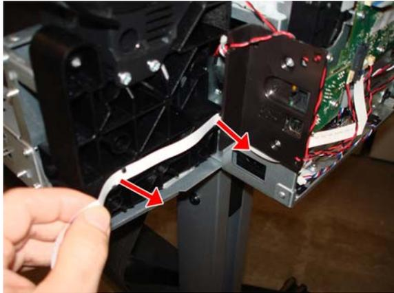
13. Disconnect the Bundle Board cable FFC from the Main PCA and remove it.
