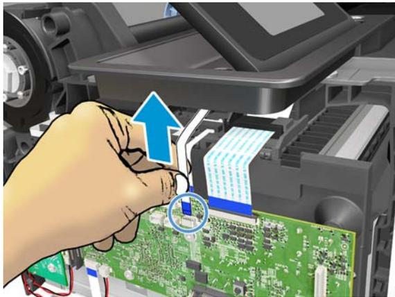
6. Hold the connector latch in these two positions and push it up to remove the FFC cable.
