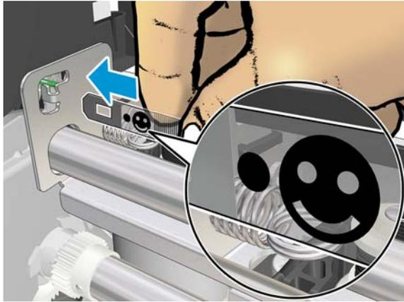
7. Attach the Encoder Strip at the left before attaching the spring at the right.
