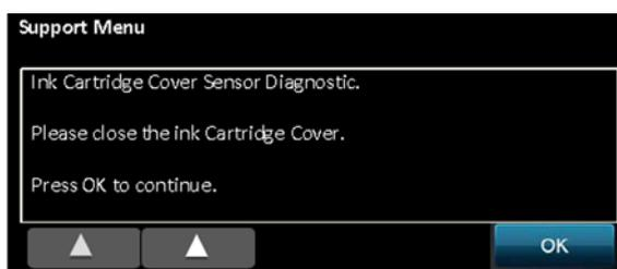
4. Close the Ink Cartridge Cover and press **OK**. If the sensor is not damaged then you will see:
