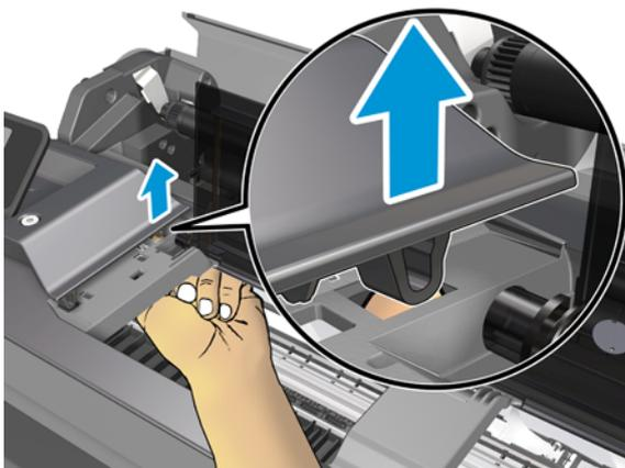
**16.** Slide up the Front Panel carefully, taking care not to damage the flat cable attached to the ferrite.
