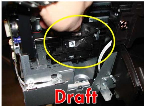
2. Move the Cutter to the right. Make sure that the cutter gears keep below the cutter guide rack and engage perfectly with it.
