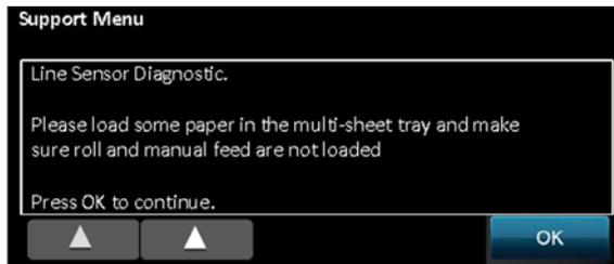
3. Check that there is paper in the Multi-Sheet Tray and the roll is unloaded and press **OK**. Then one sheet will be loaded to perform the test. If the test is correctly done you will hear 3 beeps, and the paper will be unloaded to finish the test, and the following will be displayed:
