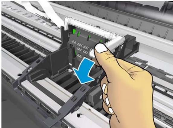
**25.** Slide the Carriage, the Belt, and the Trailing Cable to the right.
