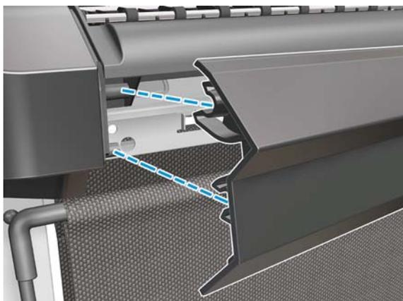
3. Snap the Front Cover into place, making sure that each of the clips is fully engaged.
