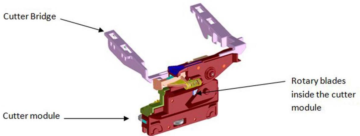
In order to operate the Cutter, it needs to be in the parked position. If not, the Cutter will not be engaged by the Cutter Bridge and the printer will not perform the cutting action.
