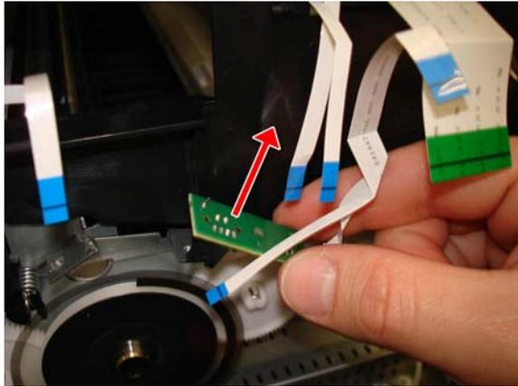
**12.** Rotate the PCA to see the connector.
