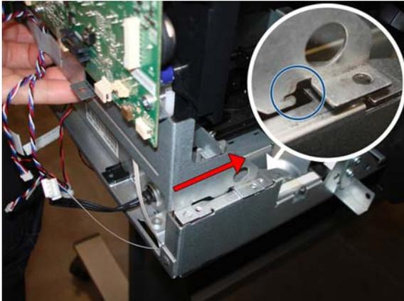
2. First place these two screws, because will be easier to screw in the next two screws.
