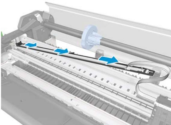
**16.** Leave the flex retainer with the trailing cable in the position shown below.
