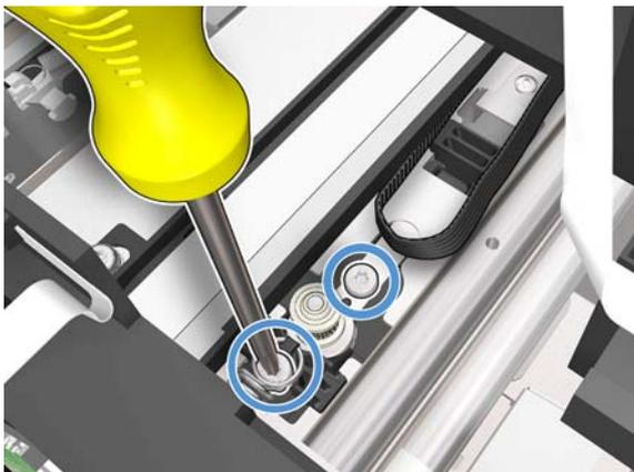
**13.** Rotate the Carriage Motor to have better access to it.
