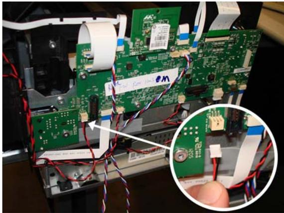
6. When you disconnect this flat cable, make sure to unlock it by pushing up the clip.
