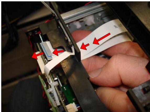
2. When connecting the cables to the Main PCA, remember that the blue side of the Trailing Cable must be facing up.
