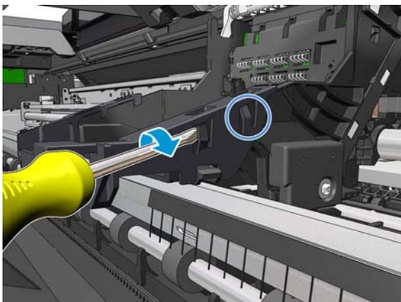
5. Use the tool again to lever up the two prongs attaching the Cutter Bridge to the left-hand side of the Carriage.
