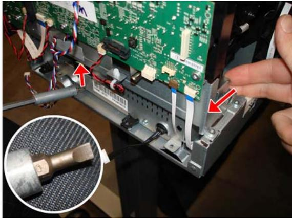
8. Never take out the Power Supply by pulling the cable, because you will damage it.
