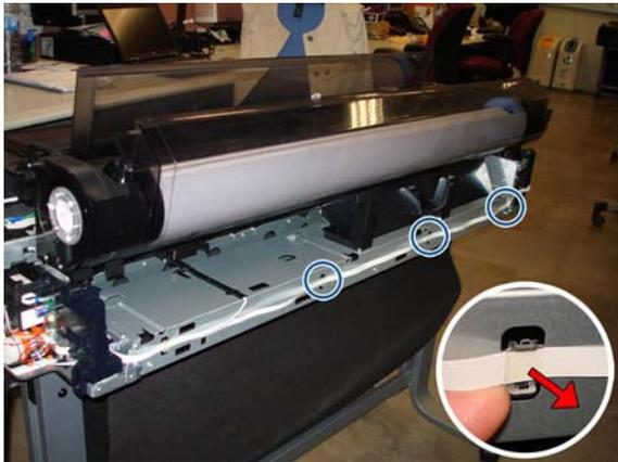
**11.** Carefully remove the FFC from the hook of the left arch.
