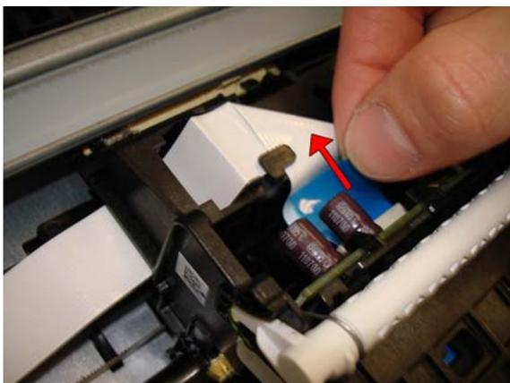
**15.** Put the Trailing Cable in a flat position, carefully avoiding making folds in the cable.
