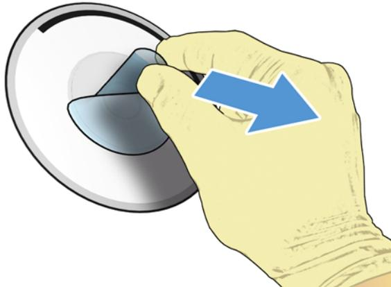
2. Clean the new Encoder Disk with a lint-free cloth dampened with alcohol to remove any remaining glue. Let it dry before proceeding.
