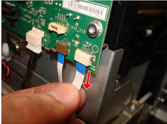
7. Remove the Ink Cartridge Cover PCA Cable.
