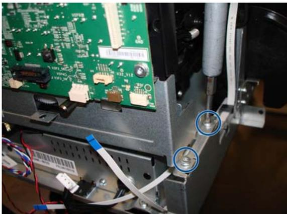
**14.** Slide out the Main PCA horizontally to disengage it from the hook.
