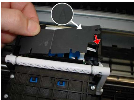
6. When the installation is complete, clean the Encoder Strip. See [Clean the Encoder Strip on page 315](#).
