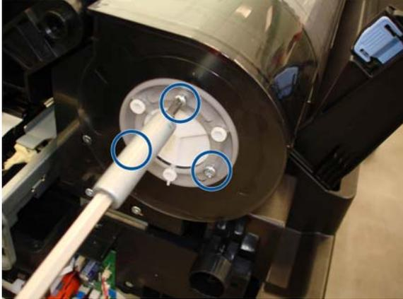
9. Unclip and detach the left side of the Roll Cover, bending it carefully.
