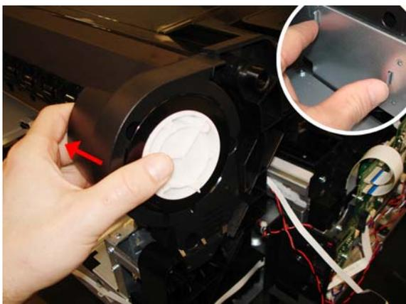
18. Remove the Left Roll Support, taking care not to damage the cables.
