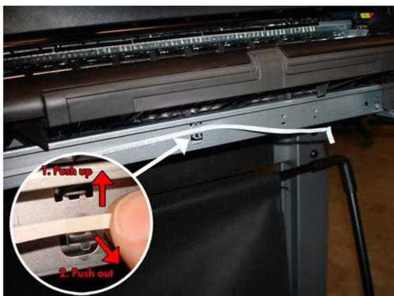
6. Unclip the locator FFC from the middle of the Front Cross Beam.
