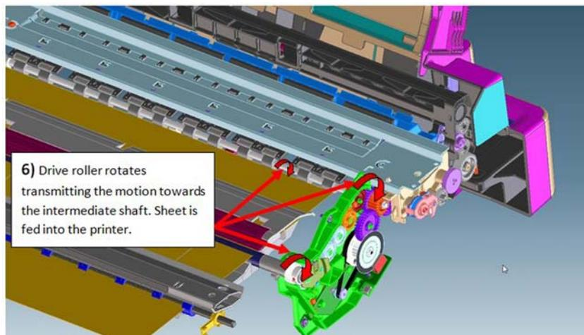
**NOTE:** It is possible to reproduce the picking and loading motions by extracting the Multi-Sheet Tray and rotating the gears with the hand, to validate module performance and troubleshoot any possible mechanical issues.
