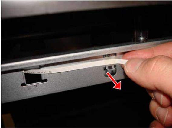
8. Disconnect the Output Tray Extender Sensor Cable from the Main PCA.
