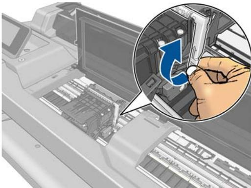
**12.** Remove the printhead, keeping it vertical to avoid spilling ink onto the connections.
