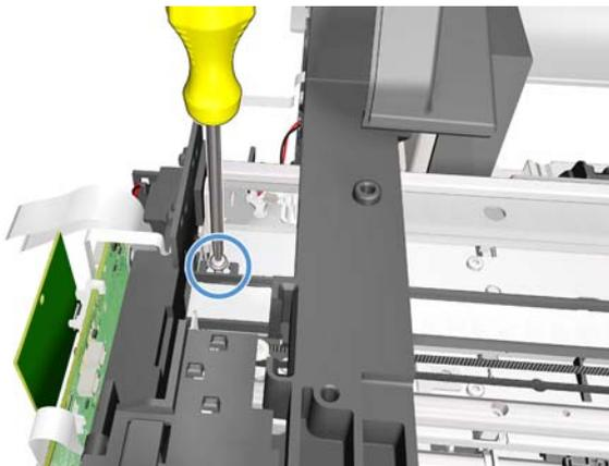
**14.** Detach the flex retainer assembly from the backbone.
