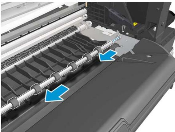
**27.** Remove the Output Shaft .
