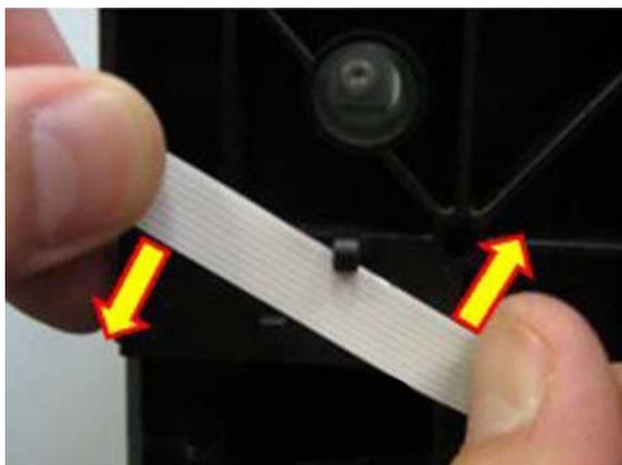
2. Unclip to remove the ferrite of the right arch.
