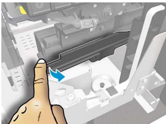
**11.** Slide the Cutter Extraction Lid to the left to detach it from the hole.
