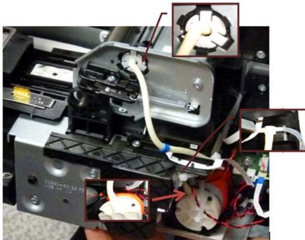
4. Replace the Pump motor, see [Prime Pump on page 233](#).
