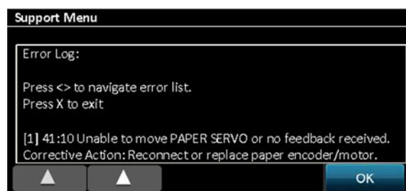
Keep using Left arrow (◀) and Right arrow (▶) in the Front Panel magic frame to navigate thru the errors list. The first error [1] is the most recently logged.
