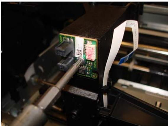
10. Remove the Ink Cartridge Cover PCA and Sensor.
