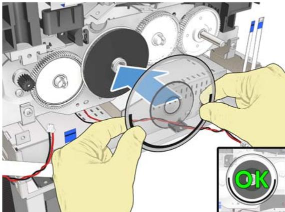
4. Make sure the Encoder Disk is firmly attached.
