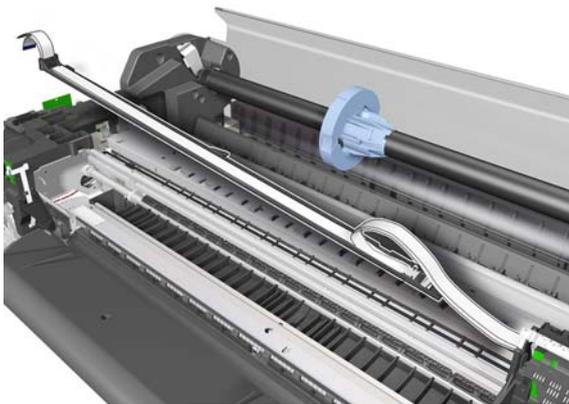
**17.** Remove two T-10 screws from the Right End Plate.
