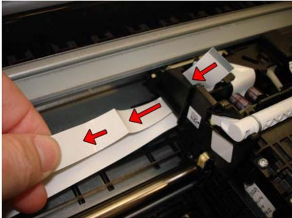
**14.** Disconnect the second Trailing Cable by pulling the blue plastic.
