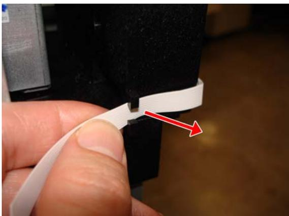
12. Carefully remove the FFC from the 2 hooks of the left arch.
