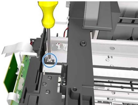
**20.** Unclip the flex retainer. You are recommended to wear gloves.
