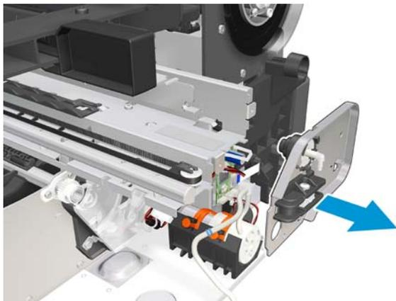
**19.** Unhook the Carriage Belt with a finger and lift it away.
