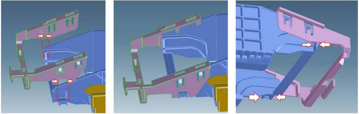
3. Use the tool provided with the Cutter Assembly Kit to press each of the four prongs attaching the Cutter Bridge to the Carriage, and make sure that all of them are correctly engaged; otherwise the Cutter may not work correctly.
