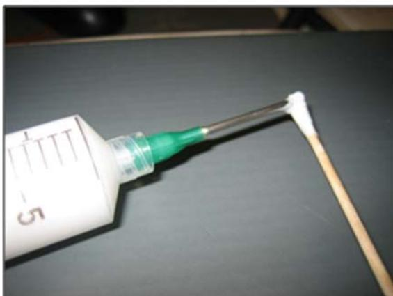
2. Apply grease to the front of the rod and smear for a distance of about 50 mm.
