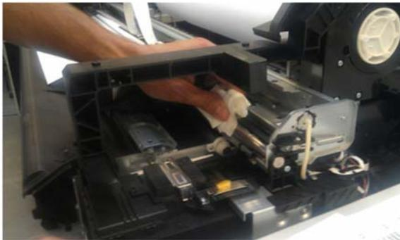
7. Return the Carriage to the capping position and cap it manually.
