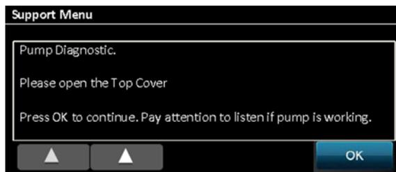
3. Open the Top Cover, the Carriage will be uncapped and moved outside of the Service Station. The Pump will start to pump for some seconds. If you can hear it, then the pump is OK.
