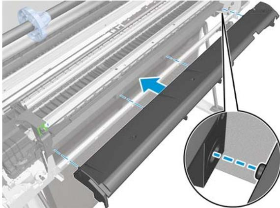
2. Introduce the Cutter Extraction Lid into the hole.
