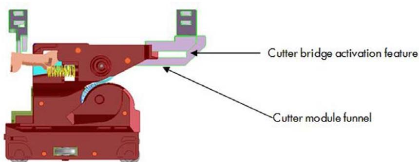
2. Hook catching: The cutter bridge continues moving to the left pushing down the cutter hook (in orange), after the left side of the cutter bridge passes the Carriage stops and the cutter hook returns to its position due to its spring motion.
