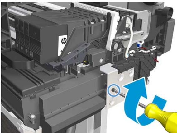
9. Move the Carriage slightly to allow access to the Carriage Line Sensor, maintain a separation of 4 cm.
