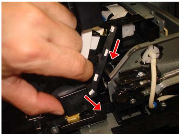
13. Remove the Carriage Line Sensor.
