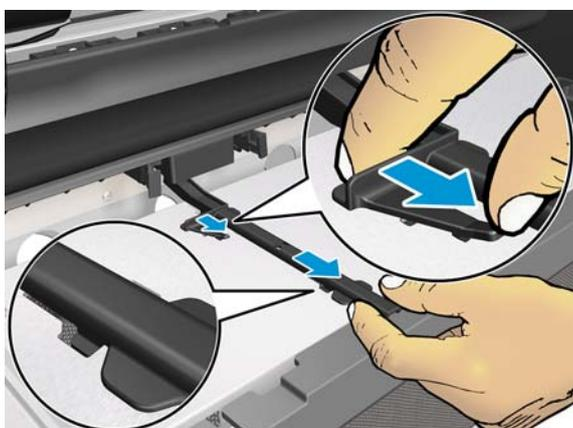
6. Lift up (1) the Out-Of-Paper Sensor FFC Cover and slide it to the left (2).
