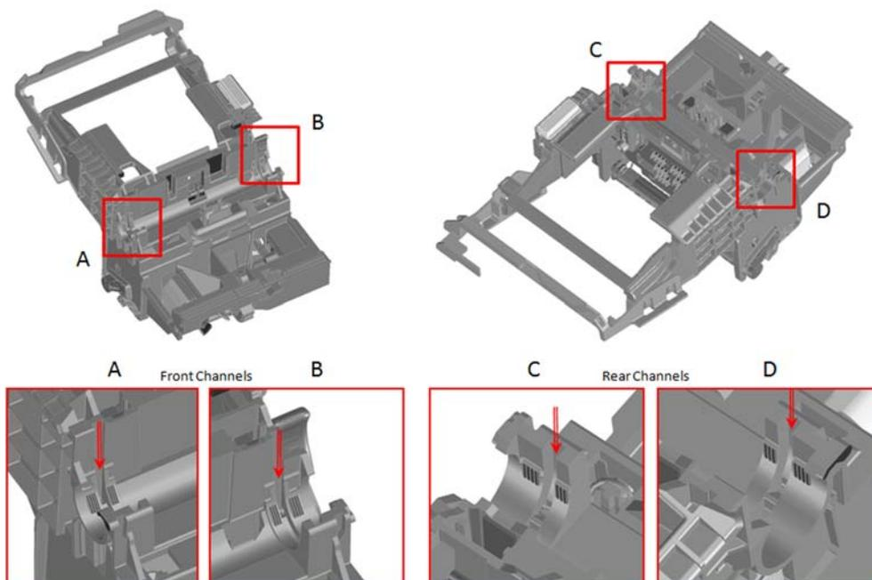
3. Use a syringe to inject grease into the ports. Push the needle against the ports firmly to direct grease into the channels.
