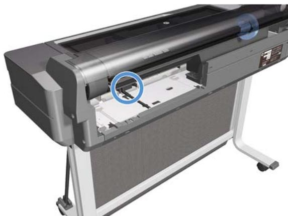
4. Unclip the Out-Of-Paper Sensor FFC Cover.
