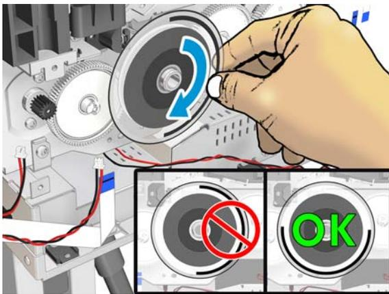
11. Remove the Encoder Disk by pulling it off (without moving the Roller).
