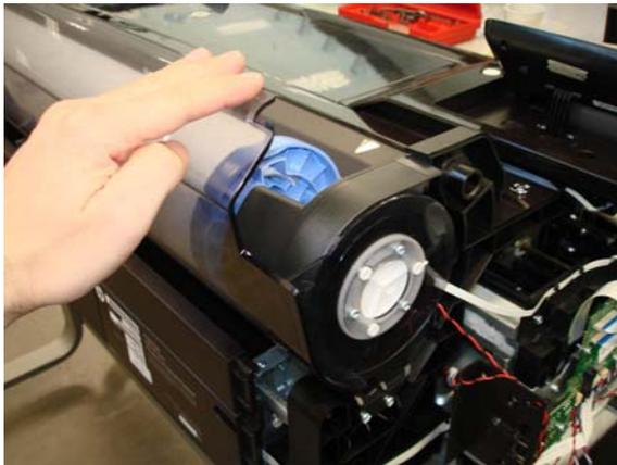
7. Remove three T-15 screws from the left side of the Roll Cover.
