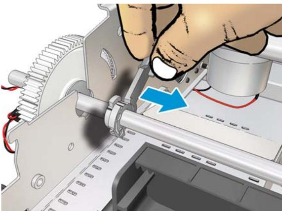
**25.** Move the Output Shaft up to detach the Middle Bearing.
