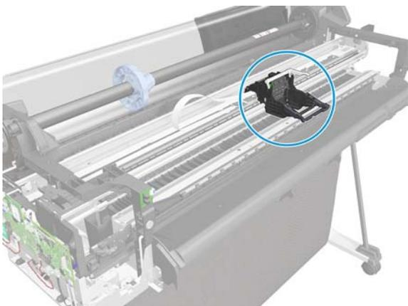
**12.** Disconnect the two flat cables from the PCA.
