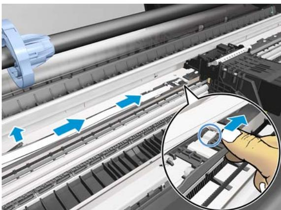
22. Slide the Trailing Cable to the right, passing the flat cables through the hole.
