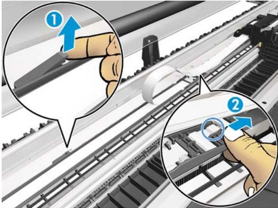
**15.** Slide the flex retainer with the trailing cable to the right. Be careful not to damage the trailing cable.
