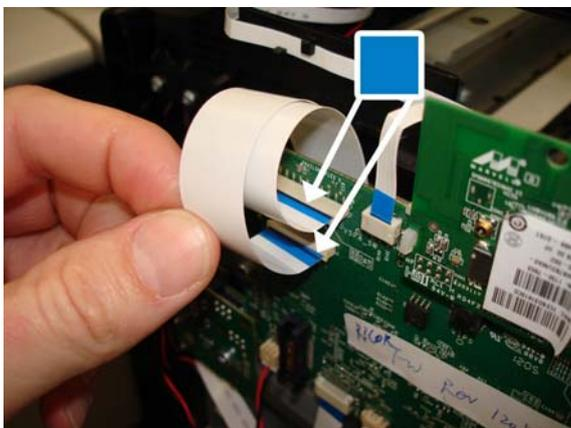
3. Hook the Trailing Cable to the two hooks.
