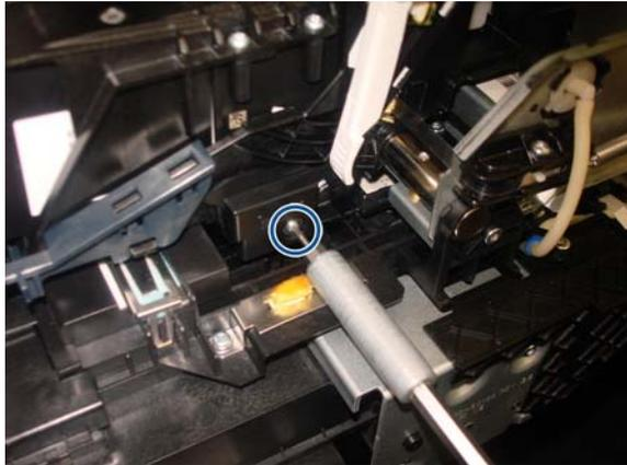
11. Open the Carriage latch upwards to allow access to the Carriage Line Sensor.
