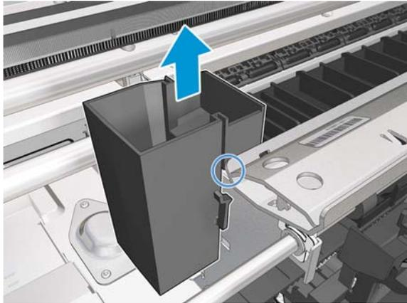
6. Remove the Left Spittoon in the vertical position. You are recommended to wear gloves.
