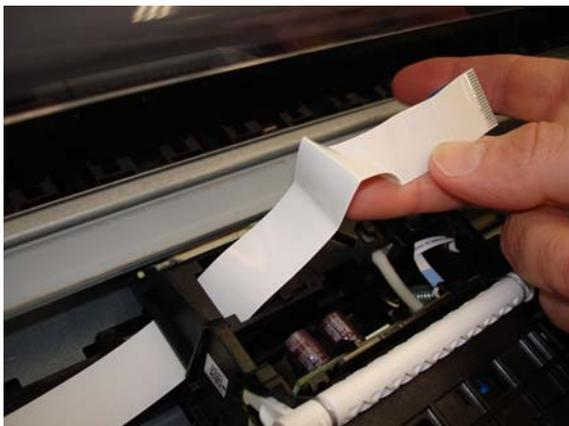
**16.** Slide out the Trailing Cable carefully through the hole.
