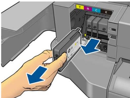
7. Insert the new ink cartridge. Make sure that you insert the ink cartridge into the slot that has the same colored letter as the cartridge you are installing.
