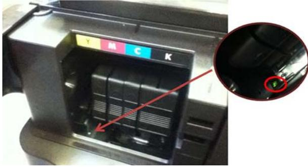
If there is no light or it is not flashing the Main PCA should be replaced.
