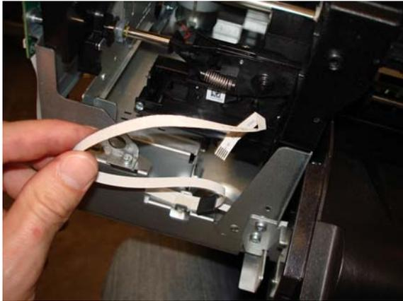
4. Unclip the Ink Cartridge Cover PCA Cable from the clip.
