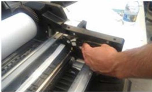
3. Place some paper over the slider rod in order to protect the lubricant and avoid cross-contamination with grease and alcohol.
