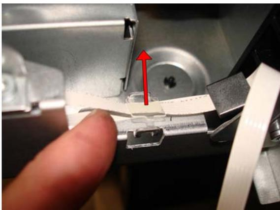
5. Slide out the Ink Cartridge Cover PCA Cable, taking care not to lose the ferrite.
