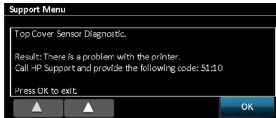
6. If there is a failure, replace the Top Cover Sensor PCA.
