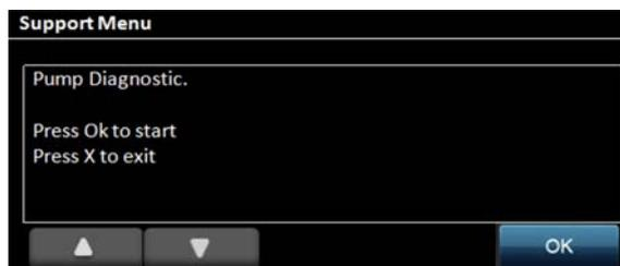
5. If you cannot hear the Pump then it should be replaced, see [Prime Pump on page 233](#).
