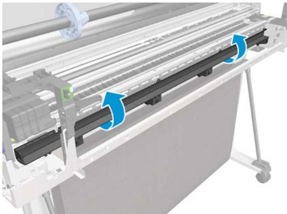
**12.** Slide the Cutter Guide to the right and remove it.
