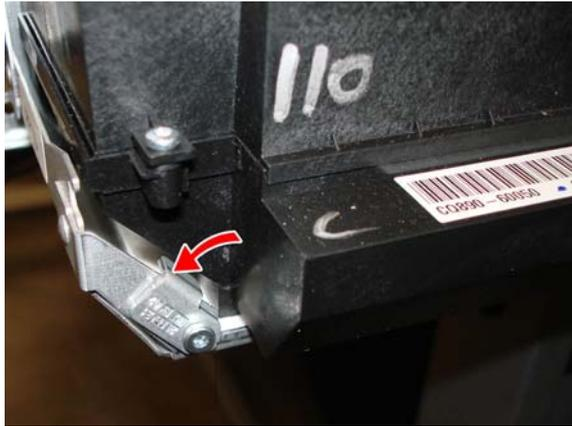
**16.** Push down the metal sheet and slide out the Service Station.
