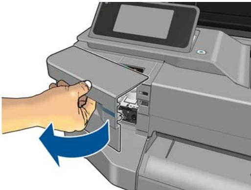
18. Insert the ink cartridges. Make sure that you insert each ink cartridge into the slot that has the same colored letter as the cartridge you are installing.
