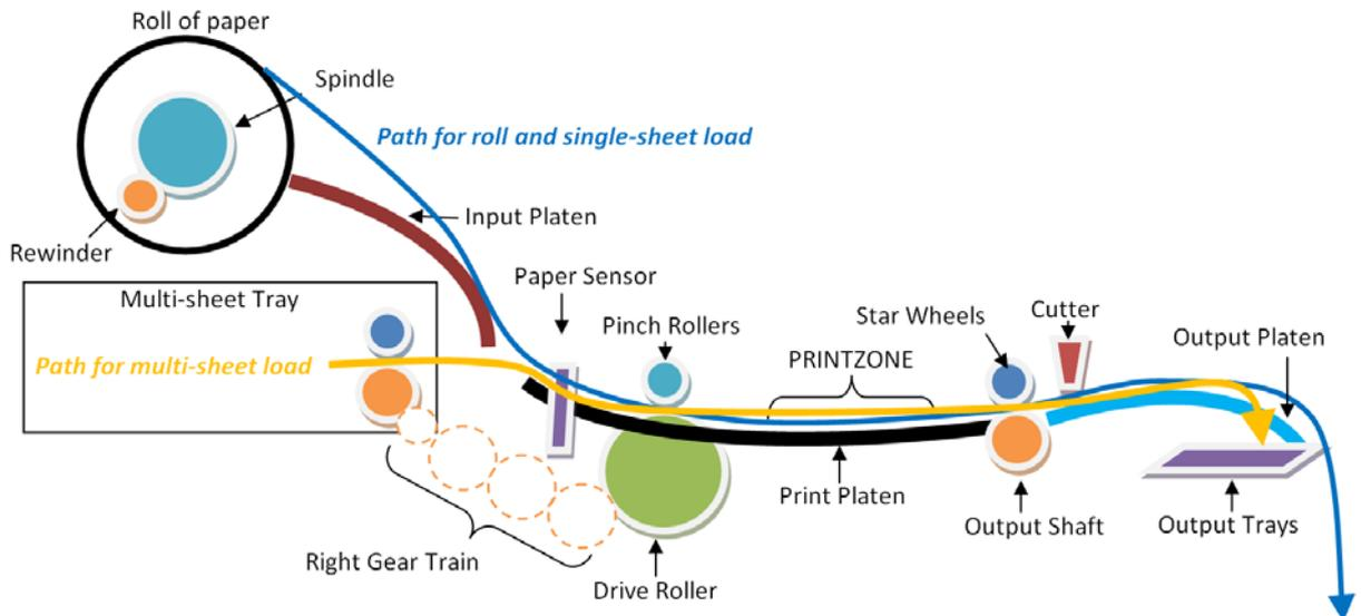
The printed paper then passes between the Output Shaft and the Starwheels (which keep the paper tension as flat as possible for printing) to exit on the Output Platen, where it is held in case of cut sheet or is cut to fall on the output basket in the case of roll paper.
