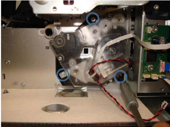
10. Slide the Right Gear Train Module horizontally to detach the pins.
