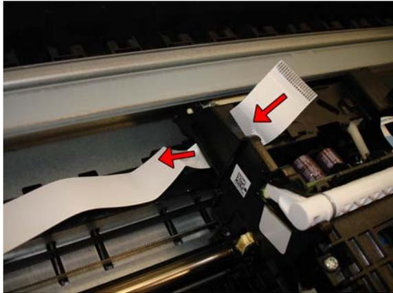
**17.** Leave the two parts of the Trailing Cable hanging on the right side.
