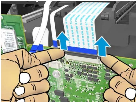
7. Take care! Do not pull up so hard that it damages the connector latch as you remove the cable.
