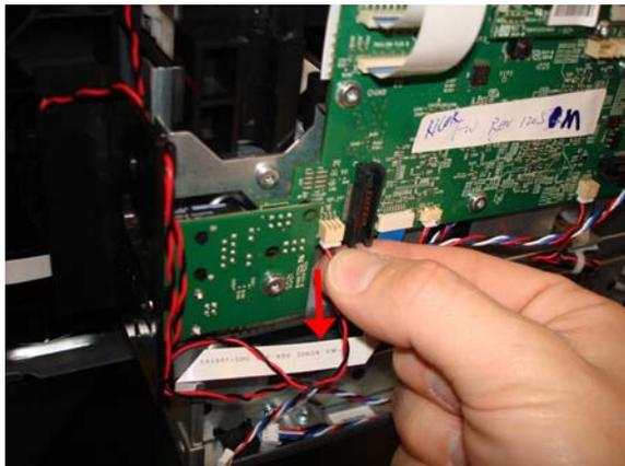
13. Detach the cable from the 3 clips of the LAN Panel USB.
