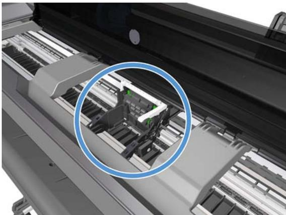
4. Use the tool provided with the Cutter Assembly Kit to lever up the two prongs attaching the Cutter Bridge to the right-hand side of the Carriage.
