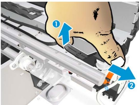
**23.** Remove the pulley latch..
