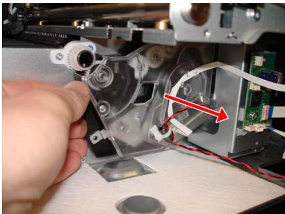
11. Remove the Right Gear Train Module.
