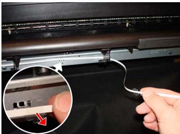
7. Unclip the locator FFC from the left of the Front Cross Beam.
