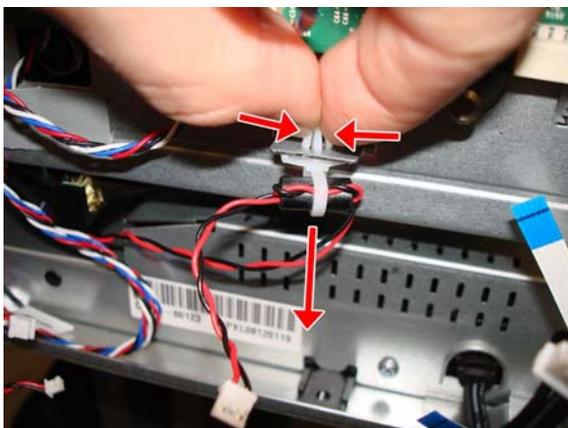
9. Unhook the two cables from the bottom hook.
