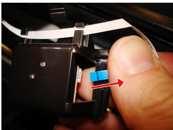
6. Slide the flat cable from the two hooks of the Top Cover Sensor.
