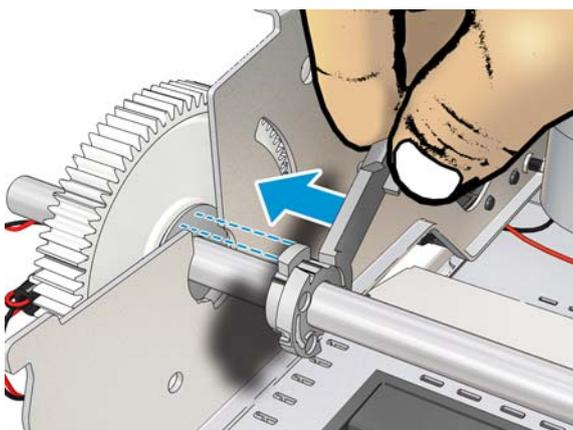
4. Rotate the Left Bearing until it clips into the hole.
