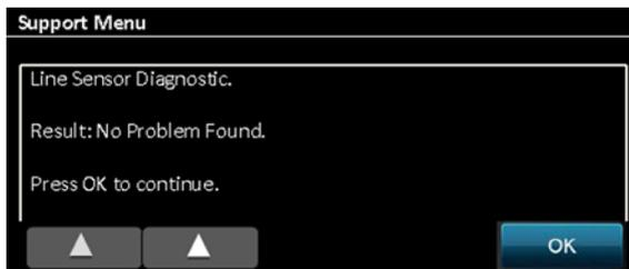
4. If the sensor is not working properly the system error 55:10 will appear. The Line Sensor should be replaced, see [Carriage Line Sensor on page 293](#).
