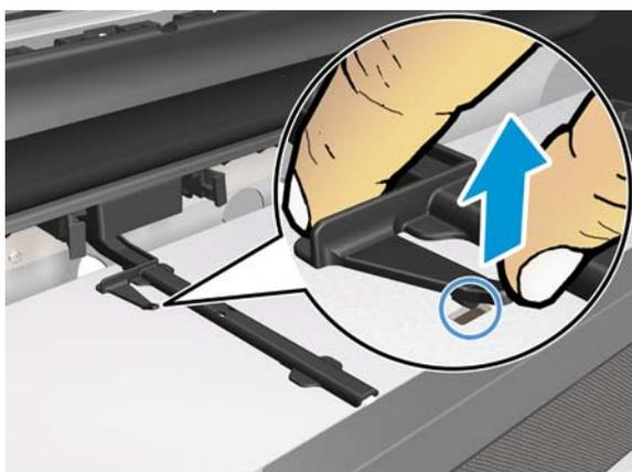
5. Slide the Out-Of-Paper Sensor FFC Cover.
