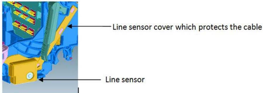
The Line Sensor is a reflective tool that generates a beam of LED light, whose reflection is detected by a luminance sensor. The signal from this sensor is used to determine the position of lines or paper edge according to the position of the Carriage.
