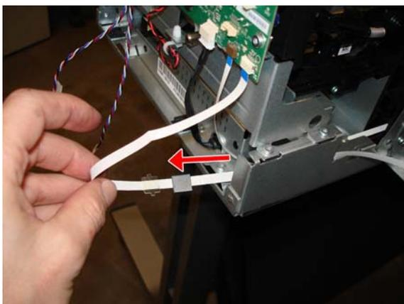
6. Disconnect the Ink Cartridge Cover PCA Cable.
