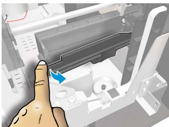
9. Slide the Cutter Extraction Lid to the left to detach it from the hole.
