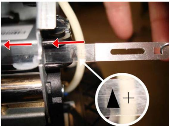
6. When you attach the left end of the Encoder Strip to the hook, make sure the position of the face is as shown below.
