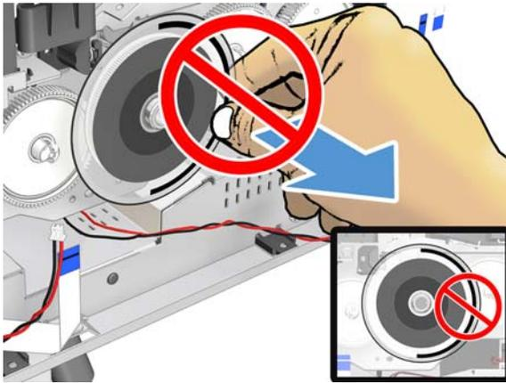
10. Rotate the Encoder Disk to a position where the black reference mark is entirely below the midpoint of the disk (so that it looks like a smile).
