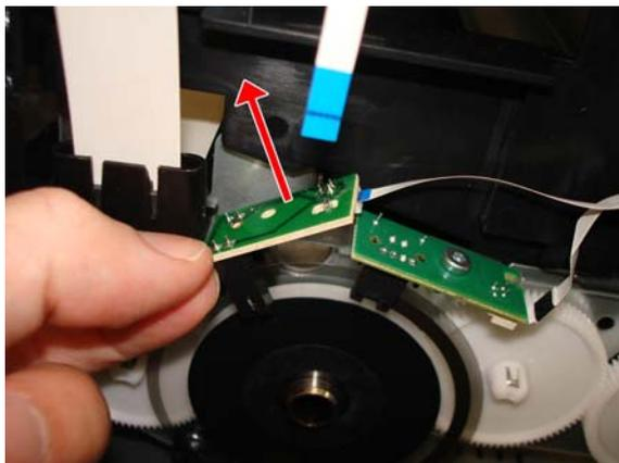
8. Rotate the PCA to see the connector.
