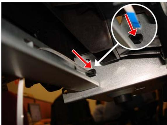
3. Slide the Output Tray Extender Sensor Cable through the hole of the left arch.
