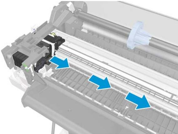
**14.** Leave the Carriage as shown below, without touching it with the Output Shaft.
