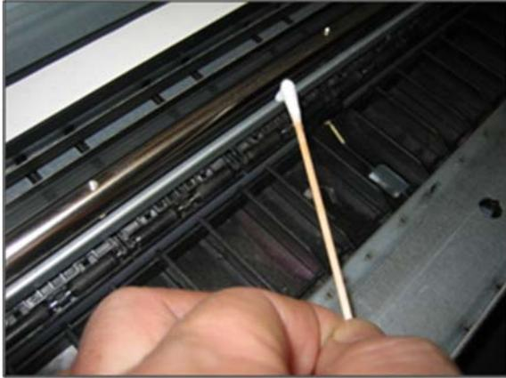
3. Apply grease to the rear of the rod and smear for a distance of about 50 mm.
