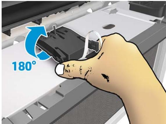
10. Disconnect the Out-Of-Paper Sensor cable.
