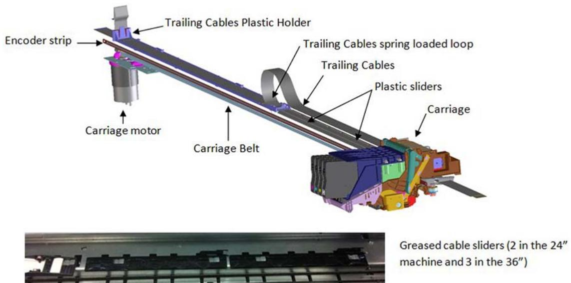
The Encoder Strip Sensor is located inside the Carriage, once the Carriage is assembled the Encoder Strip crosses the Carriage, passing by the detection area of the sensor inside the Carriage.
