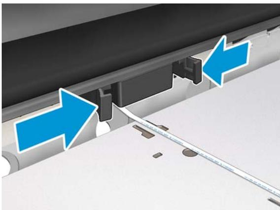
8. Slide out the Out-Of-Paper Sensor Assembly.
