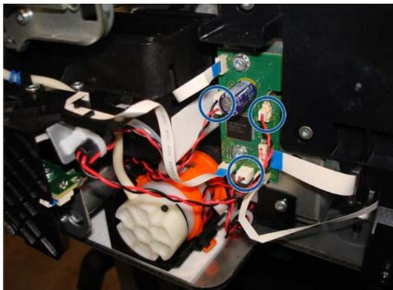
5. Disconnect four FFC (flat flexible cables) from the Bundle Board.
