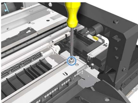
**10.** Detach the Starwheel Assembly from the two hooks by sliding it up.
