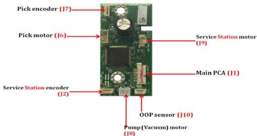
**IMPORTANT:** The pick encoder and Service Station cables are not poka-yoke cables: it is possible to connect them incorrectly, in which case a system error will result.
