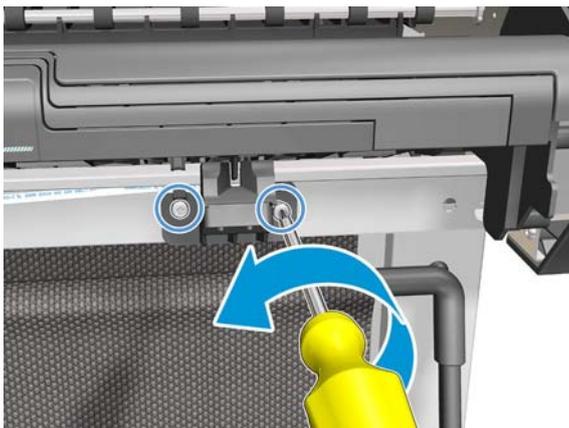
4. Detach the Output Tray Sensor from the two locator pins.
