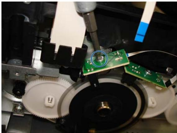
7. Release the PCA from the pin or locator.
