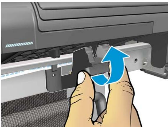
5. Remove the Output Tray Sensor Assembly in the direction shown below.
