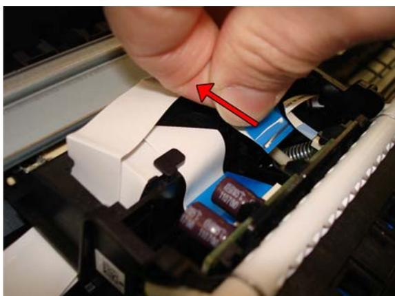
**12.** Put the Trailing Cable in a flat position, carefully avoiding making folds in the cable.
