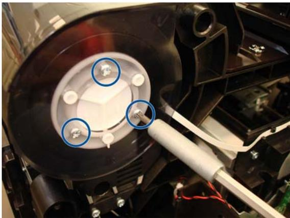
8. Remove three T-15 screws from the right side of the Roll Cover.
