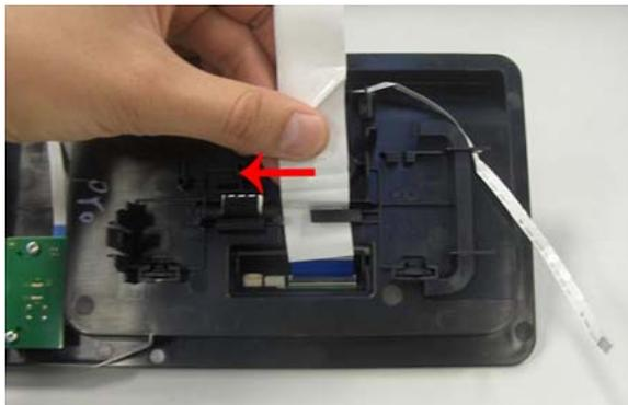
4. Push up the Front Panel FFC connector flap.
