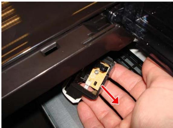
5. Disconnect the flat cable from the Top Cover Sensor.
