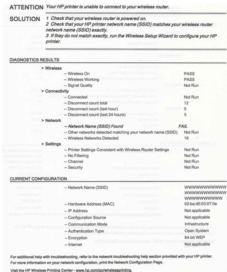
For more information about the contents of the Wireless Network Troubleshooting Report, see [Wireless troubleshooting report error cases on page 340](#). There is only one situation that requires on-site repair: when the Wireless PCA is defective. To replace the Wireless PCA, you must replace the Main PCA; see [Main PCA on page 205](#).
