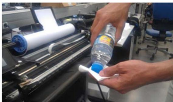
5. Clean the encoder strip carefully, not moving the papers underneath and not stretching the strip.
