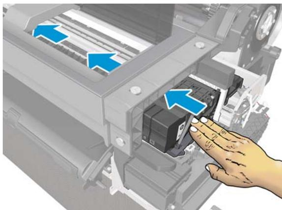
**⚠ CAUTION:** Make sure the Carriage is positioned at the far left, so that the Trailing Cable does not become damaged.
