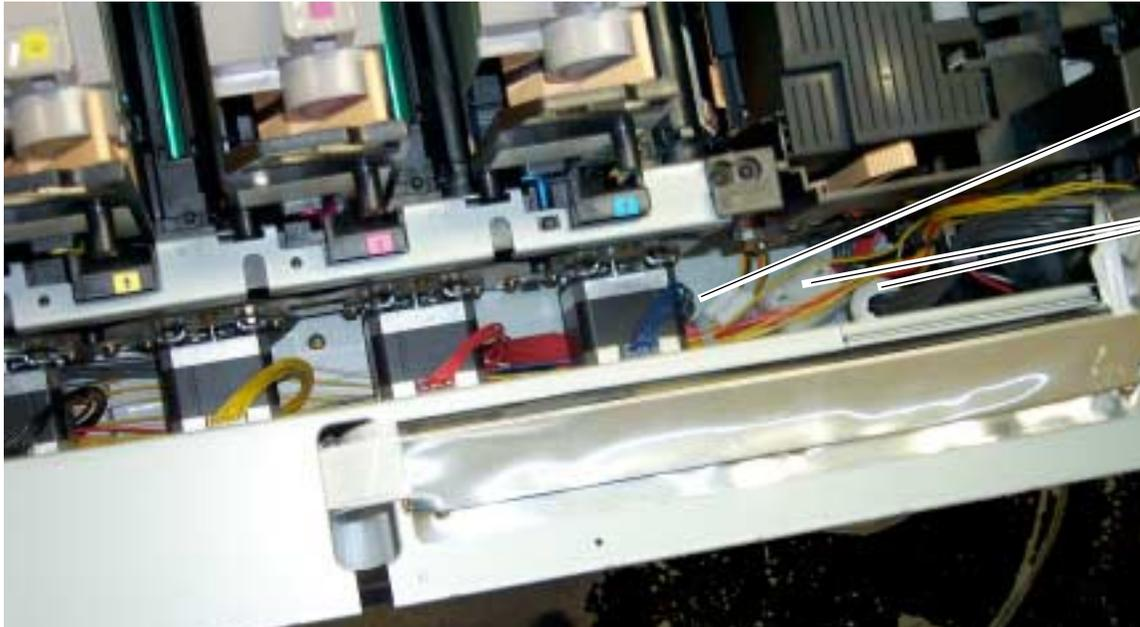
Route wiring harnesses under the imaging drum motors
