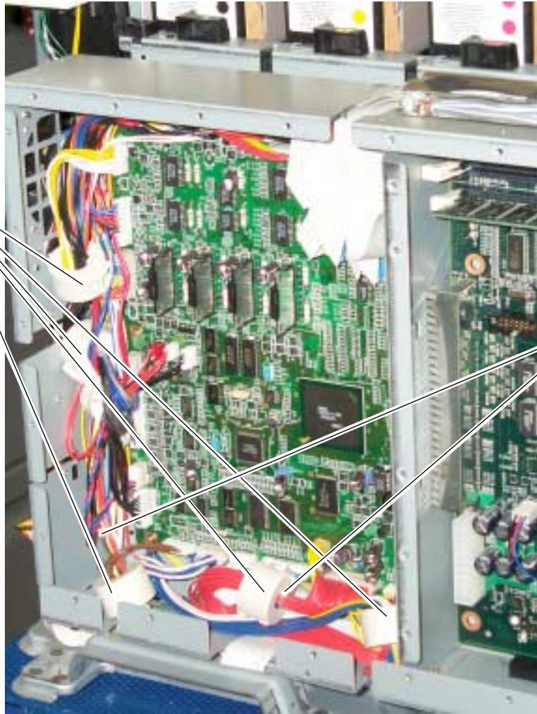
The wiring receptacles are color-coded with their plugs for correct placement
