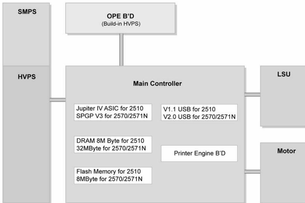
**Figure 4 :Hardware Structure**
