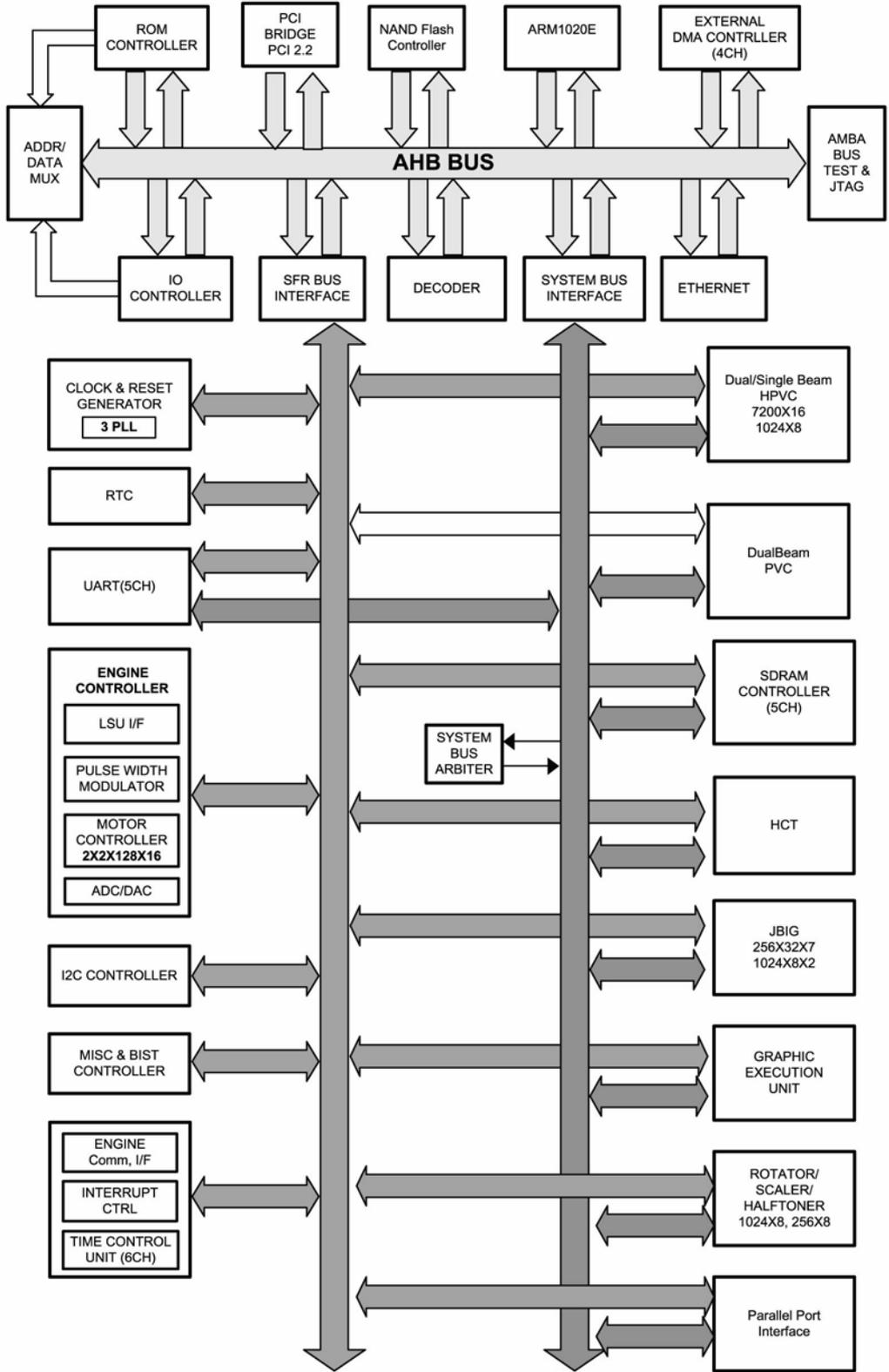
Figure 6 SPGPv3 Internal Block Diagram
