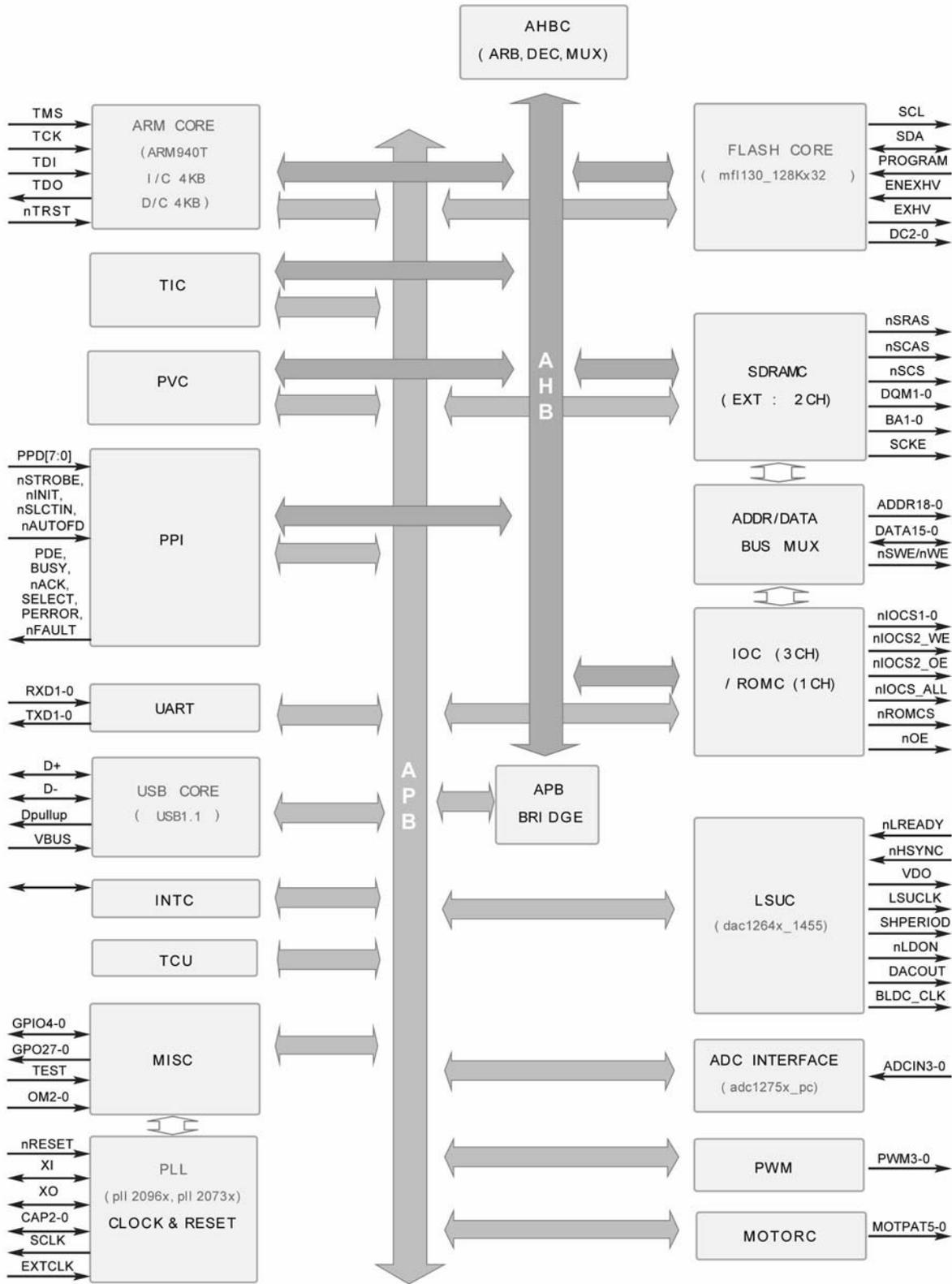
Figure 5 Jupiter4E Internal Block Diagram
