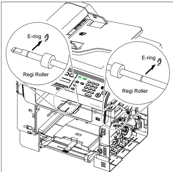
4. Take off the Sheet and then remove the Regi Pulley, as shown below.
