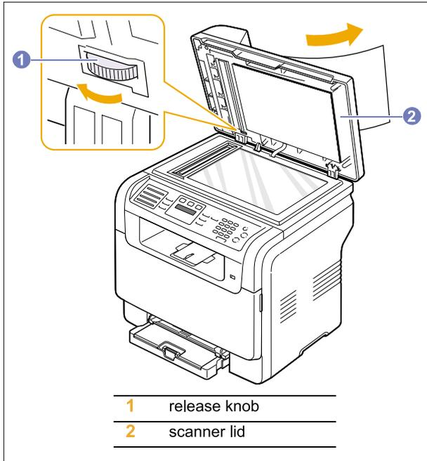
3. Close the scanner lid. Then load the removed pages back into the ADF.
