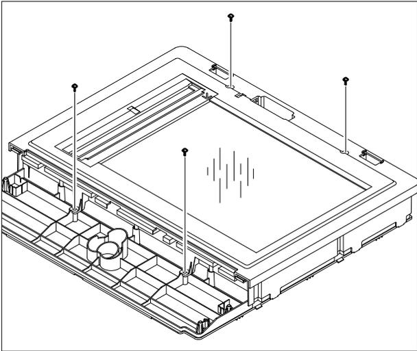
7. Release the six hooks securing the Scan Upper to the Scan Lower and remove it, as shown below.
