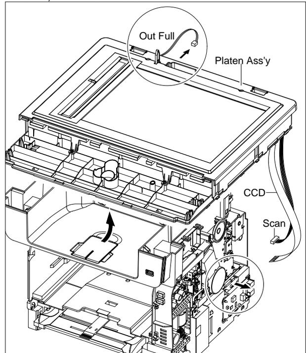
6. Remove the four screws securing the Scan Upper.
