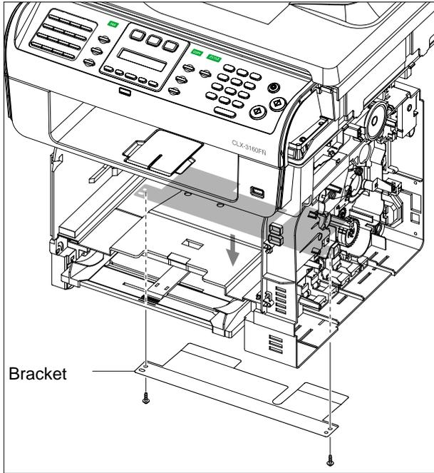
3. Remove the three screws securing the Pick Up Plate (with Pick Up Guide) and then release the Pick Up Plate in the direction of arrow.
