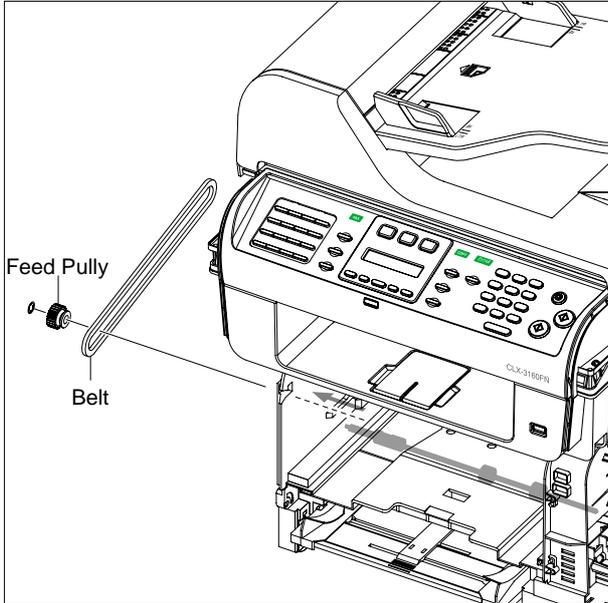
3. Remove the Feed Gear and then remove the E-ring from the Feed Shaft, as shown below.
