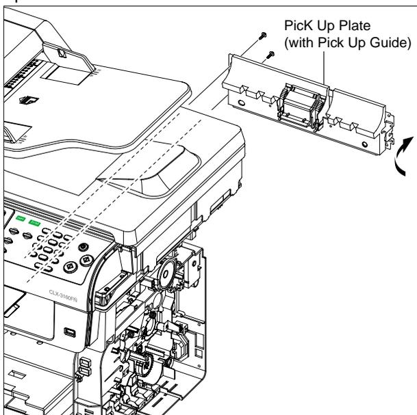
4. If necessary, remove the two screws securing the Pick Up Plate and remove it from the Pick Up Guide, as shown below.
