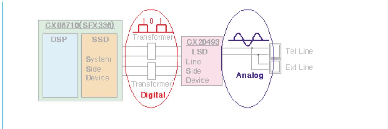
Transformer transfer Clock from SSD to LSD and Clock Frequency is 4.032MHz.
