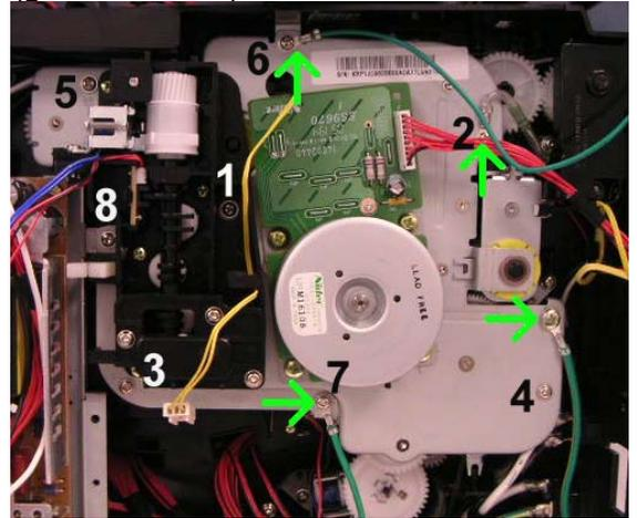
NOTE: Check wiring is secured as shown (arrow).
