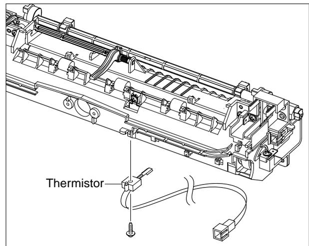
6. For easy disassembly, release the Link1 Harness and Link2 Harness, as shown below.
