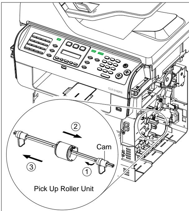
8. When if only remove the Pick Up Rubber, first pull the Pick Up Rubber(with Housing U) from the Housing B in the direction of arrow and then release the Pick Up Rubber from the Housing U, as shown below.
