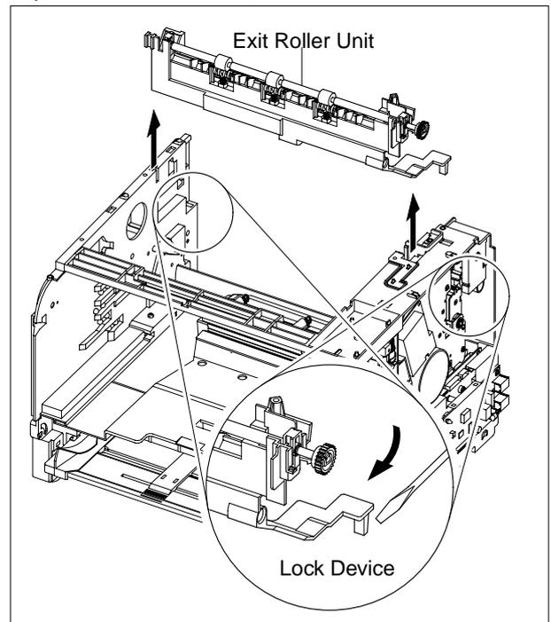
6. Remove the Holder Bearing(with Roller Exit F/Down) from the both side of the Exit Frame, as shown below and then remove the Roller Exit Main and Holder Exit F/Down.
