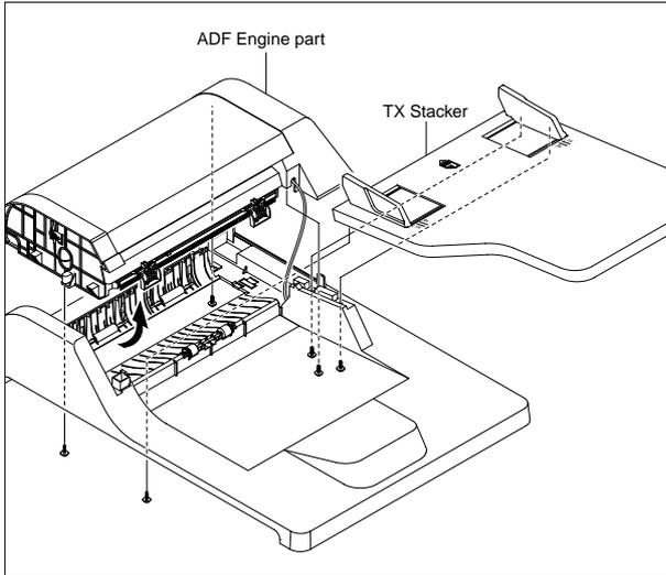
2. Remove the two screws securing the ADF Harness to the Cover Connector and then take care to thread the ADF Harness through the Cover Platen.
