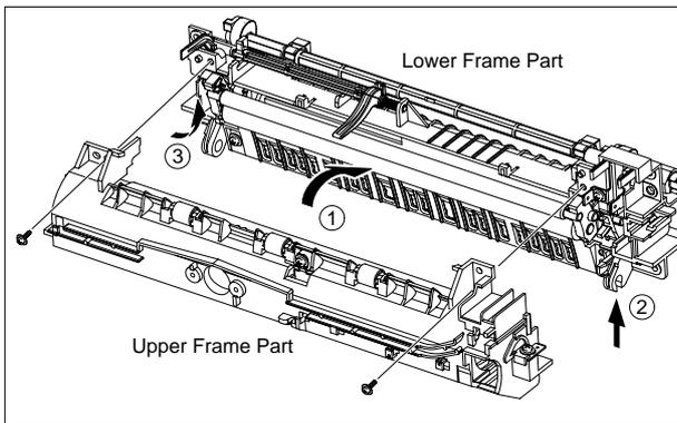
*Notice: Be careful especially not to damage the covering of the Fuser Ass'y (If the cover is damaged, it could cause an electric leakage)*
