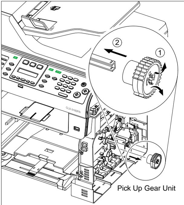
7. To remove the Pick Up Roller Unit, first lift the notch attached to the right side Pick Up Cam so that it's slide the right to left from the Pick Up Shaft, and then slide the Pick Up Roller Unit left side to right side and take out the left side, as shown below.
