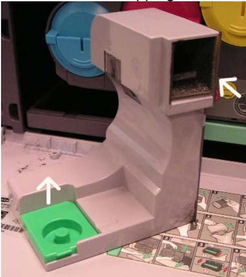
3. Remove the toner cartridges and install the clear plastic shipping cover (shipping cover is installed on all new cartridges). Secure the Cartridges into the output tray or top of the machine for shipping.
