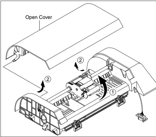
4. Release the Bush and rotate it until it reaches the slot, as shown below and then lift the Pick Up Ass'y out in the direction of arrow.
