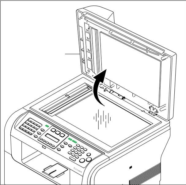
2. First remove the ADF Harness from the Platen Ass'y and then pull the ADF Ass'y upward in the direction of arrow, as shown below.
