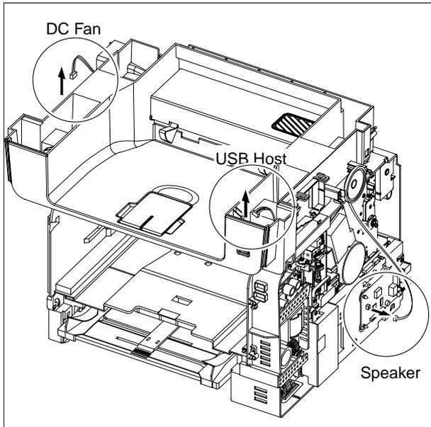
3. Remove the five screws securing the Middle Cover Ass'y and then lift the Middle Cover Ass'y, as shown below.
