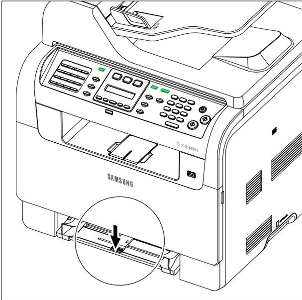
3. Apply light pressure to the both side of the MP Unit and pull it in the direction of arrow, as shown below.
