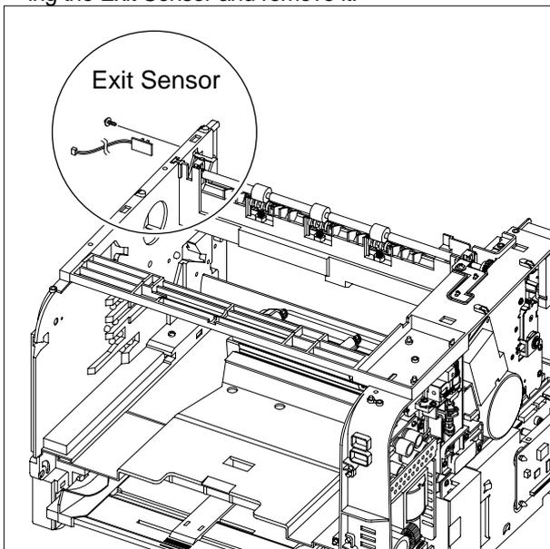
4. Remove the three screws securing the Exit Roller Unit.
