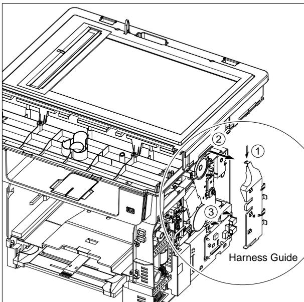
4. First release the OPE Harness in the direction of arrow and then remove the one screw securing the Ground Cable, as shown below.
