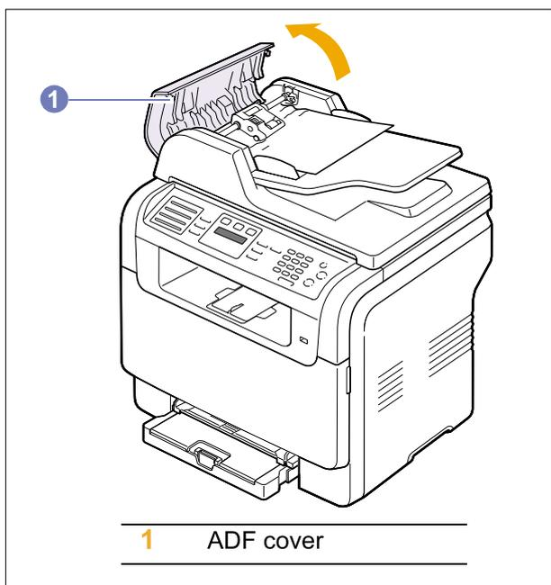
4. Close the ADF cover. Then load the removed pages, if any, back into the ADF.
