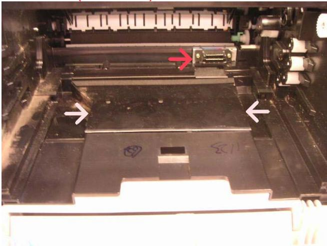
3. Disconnect left electrical plug, remove Screws (3) and lift LSU enough to access and disconnect right side electrical plug (**CAUTION:** Hold small PWB while disconnecting plug, red arrow) and remove LSU.
