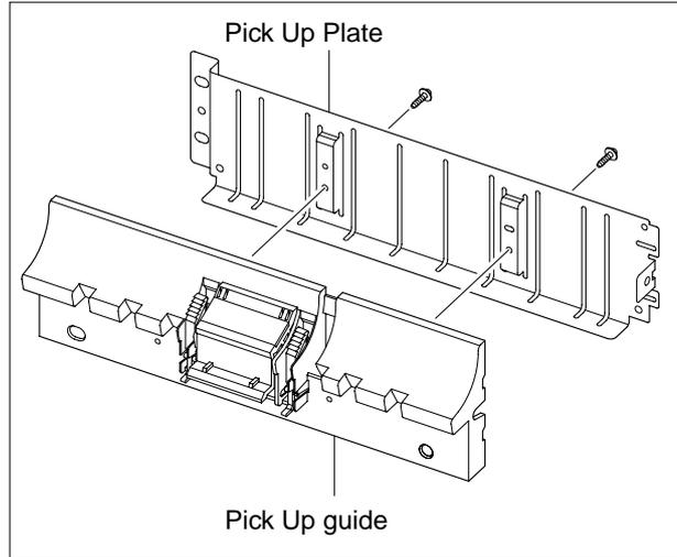
5. If necessary, pull the Pad Holder from the Pick Up Guide, as shown below.
