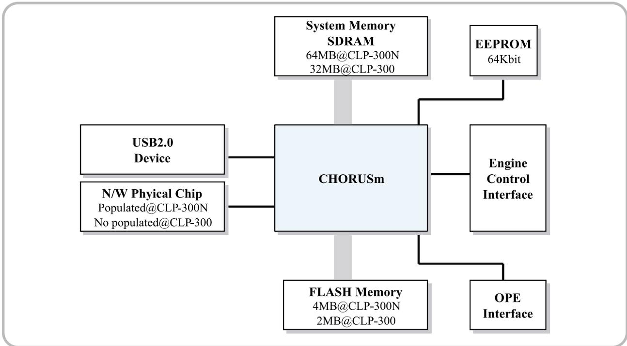
CHORUSm involves in itself the functions to control ARM Processor Core and various H/W devices. CHORUSm, therefore, controls Main PBA and all engine mechanism, processing the print job received from host and enabling the engine to print image.
