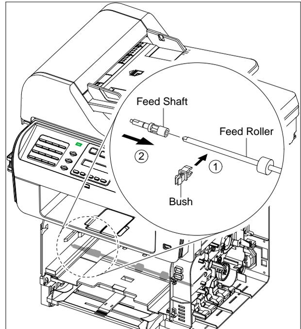
*Notice : Do not grab the rubber part of the Feed Roller, it may cause a malfunction due to a foreign object.*
