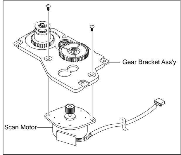
11. Remove the three screws securing the Scan Motor Ass'y and then unplug the connector from the Joint PBA.
