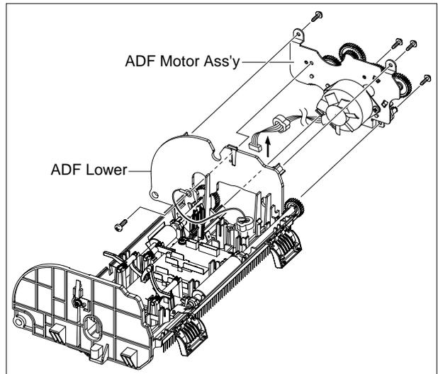
*Notice : 1) When working on the ADF Motor Ass'y take care not to contaminate any of the rubber surfaces with grease.*
