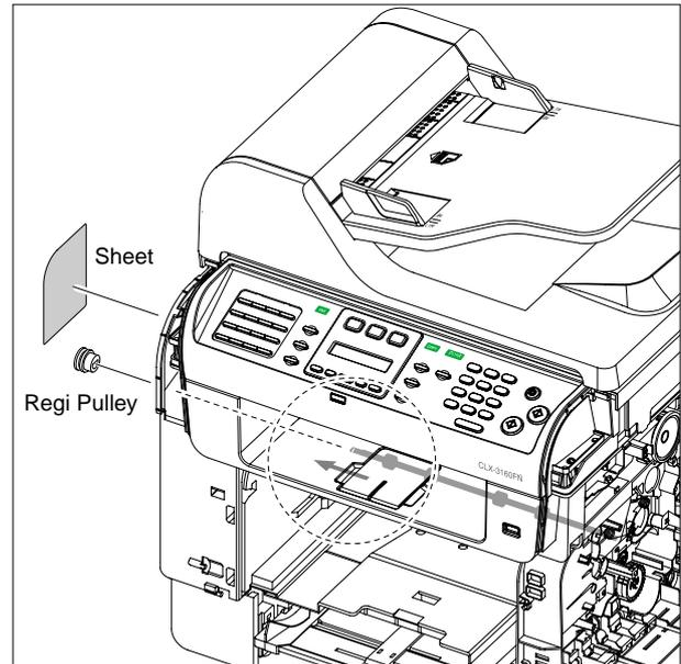
5. To remove the Regi Roller, first slide the left side to right side and then take out the left side, as shown below.
