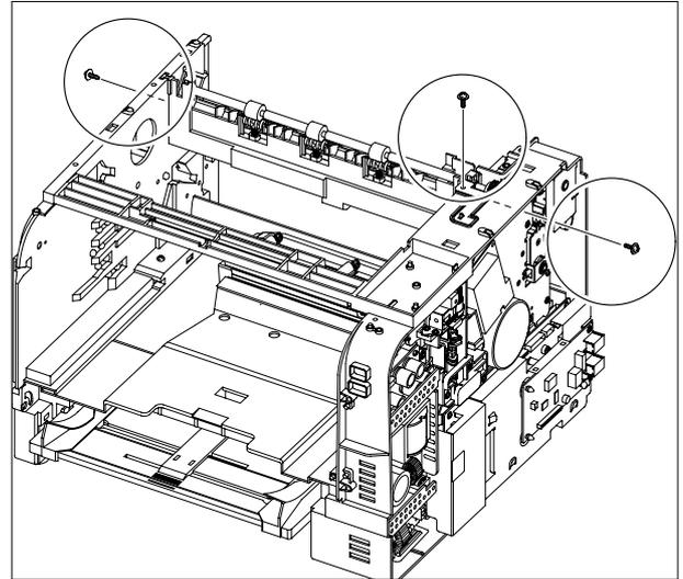
5. First unlatch the lock device below the both side of the Exit Frame using a flat-blade screwdriver and then pull the Exit Roller Unit, as shown below.
