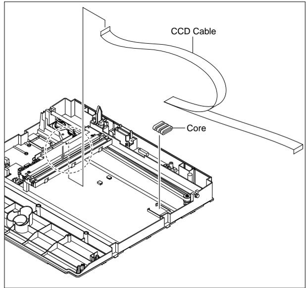
*Notice: You should connector remove the CCD Cable vertically to avoid the CCD Cable pin damage.*
