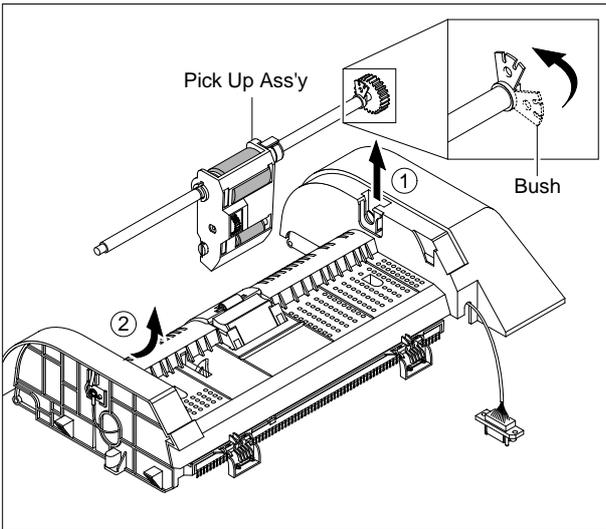
*Notice : Do not grab the rubber part of the Pick Up Ass'y, it may cause a malfunction due to a foreign object.*
