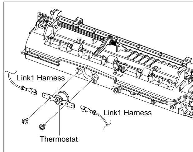
5. Remove the one screw securing the Thermistor and release it, as shown below.
