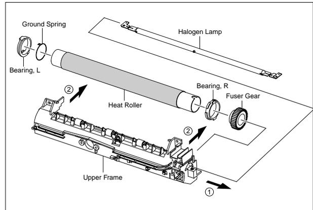
*Notice: Be careful not to damage or contaminate the surface of the roller when assembling and disassembling the Heat Roller.*
