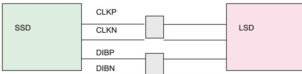
Clock from SSD to LSD has Differential structure of 180 phase difference for Noise Robustness
