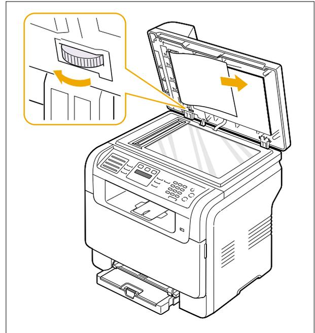
3. Close the scanner lid. Then load the removed pages back into the ADF.
