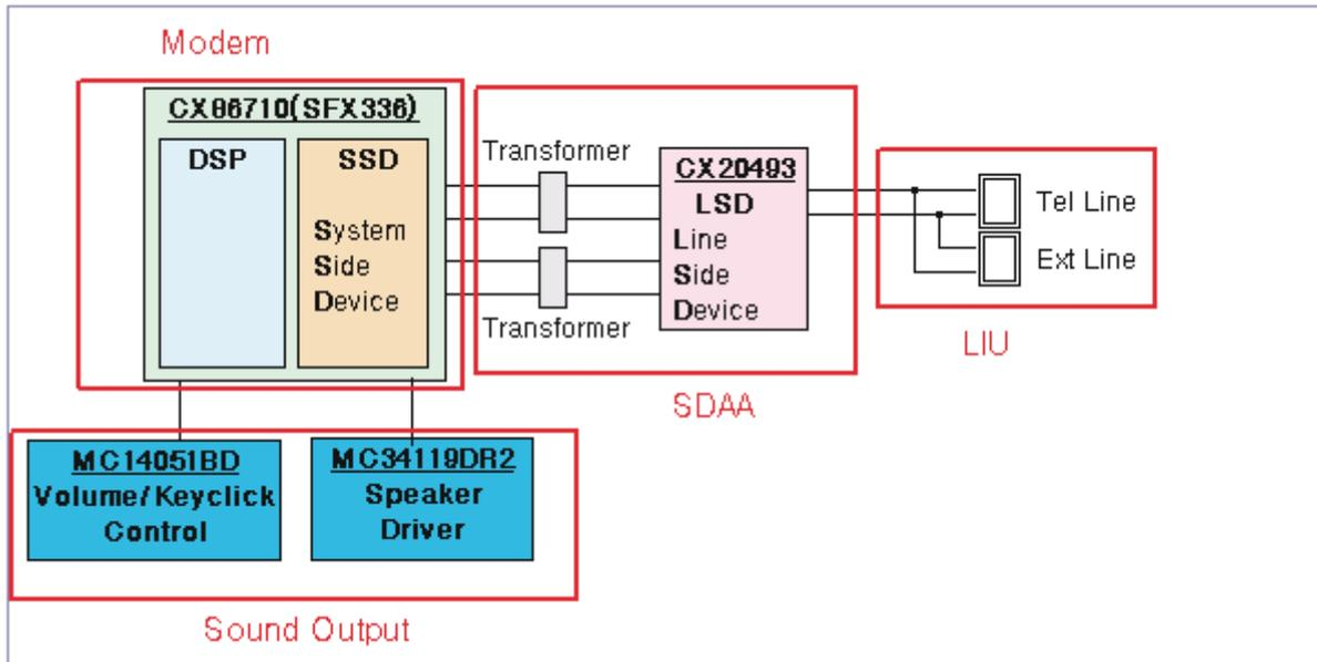
Implemented by based on Conexant DAA (Data Access Arrangement) Solution, and is roughly composed of two kinds Chip Solution
