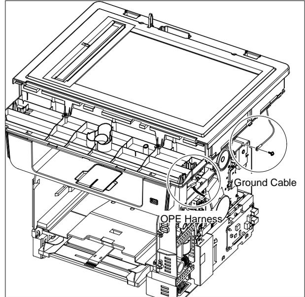
5. Unplug the two connectors (Scan, Out Full) and CCD Cable and then lift the Platen Ass'y in the direction of arrow, as shown below.
