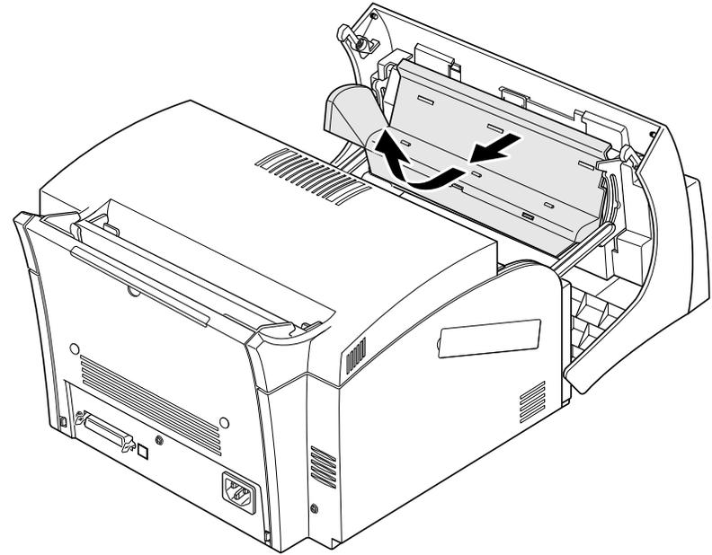
5. Remove the cover stopper securing the OPE unit. To remove the stopper, slide it until it reaches slot at the center, then take it out.
