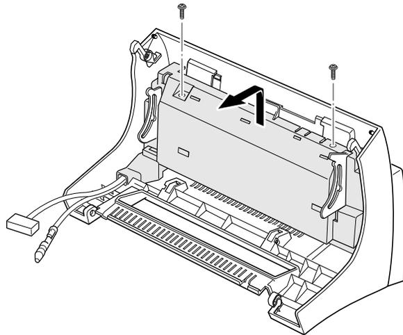
3. Unplug all connectors from the scan PBA, remove one screw, then remove the PBA.
