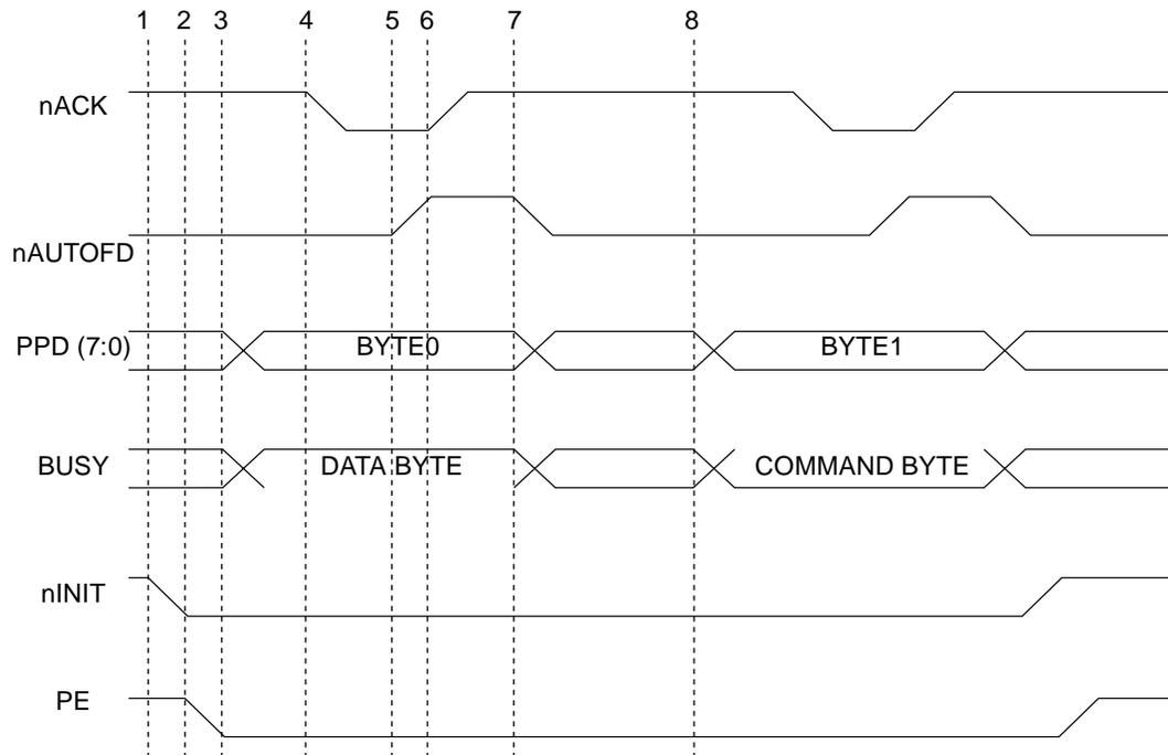
FIG. 7-7: ECP HARDWARE HANDSHAKING TIMING (REVERSE)
