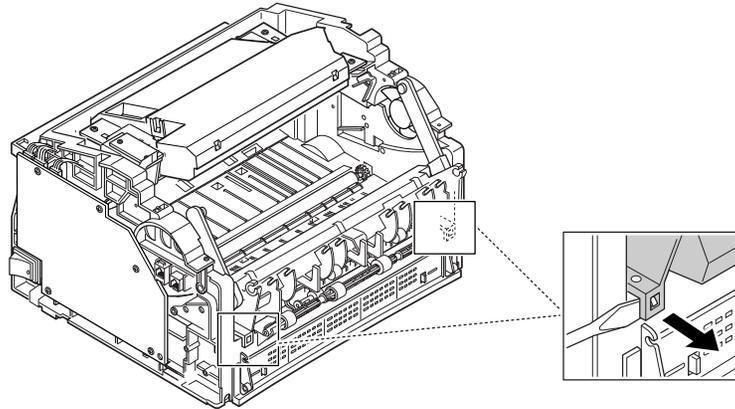
6. Unlatch the right end, then push the right end slightly inward. A flat blade screwdriver may be needed to release the pin on the right end.
