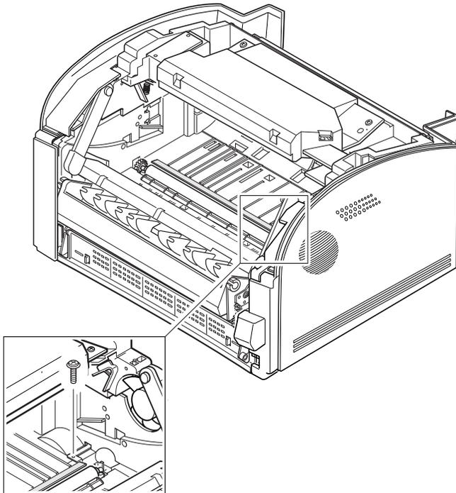
3. Unlatch the three metal tabs on the rear side of the PTL Unit, then take it out.
