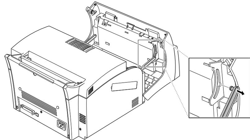
6. Wide open the cover. Pull the bottom left end of the cover toward you to unlatch the OPE cover, and take it out.
