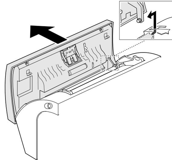
7. Remove ground wire from routing tabs on back of OPE cover.
