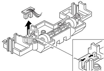
3. **To remove the P-empty actuator:**
