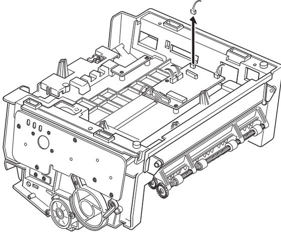
3. Remove one screw, then remove the Fuser Deve.
