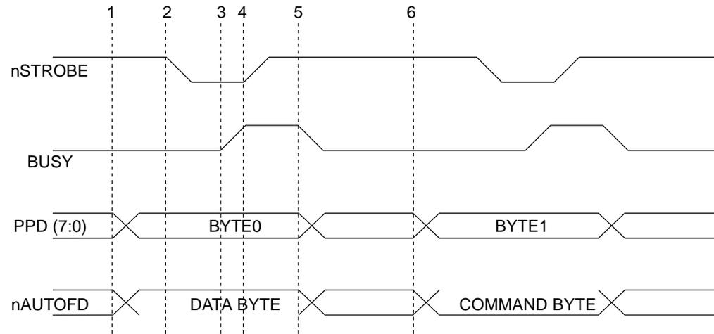
FIG. 7-6: ECP HARDWARE HANDSHAKING TIMING (FORWARD)
