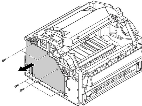
3. Unplug four connectors from the HVPS PBA, then remove the PBA.
