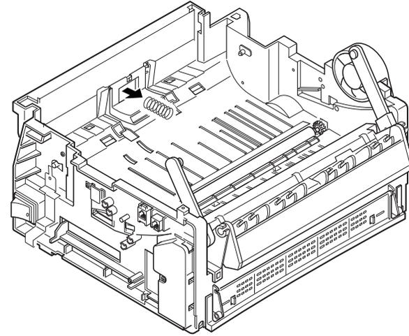
4. Remove the Spring Holder with small spring on rear post.
