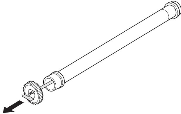
5. To remove the gear from the lamp, the metal terminal on the lamp must be positioned so that it can be extracted from the center hole and slot on the gear.
