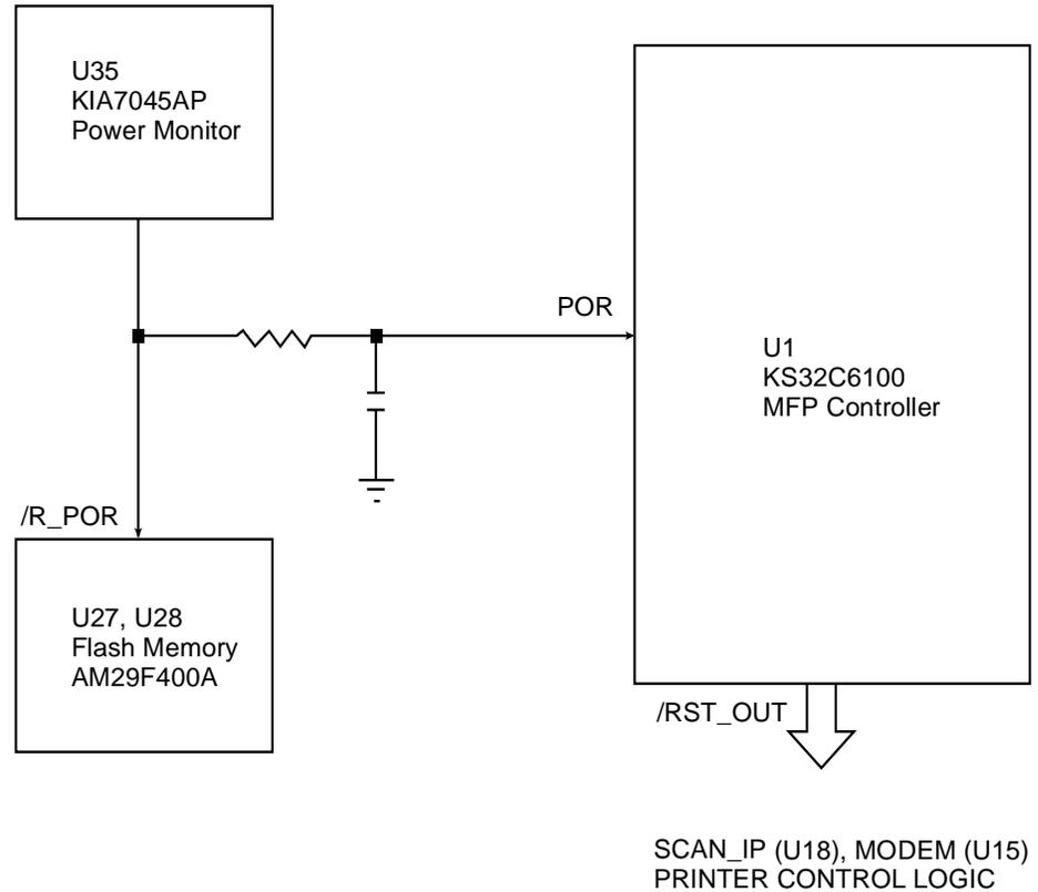
FIG. 7-8: POWER RESET DIAGRAM
