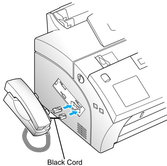
Route the excess cord so that it can be inserted into the cradle.
