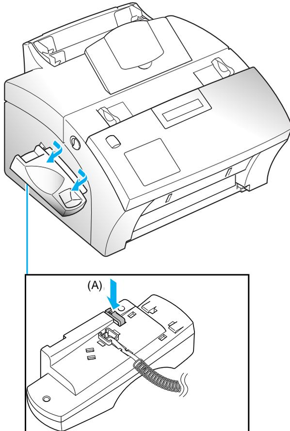
3. Disconnect the Handset and Hook Switch connectors from the machine.
