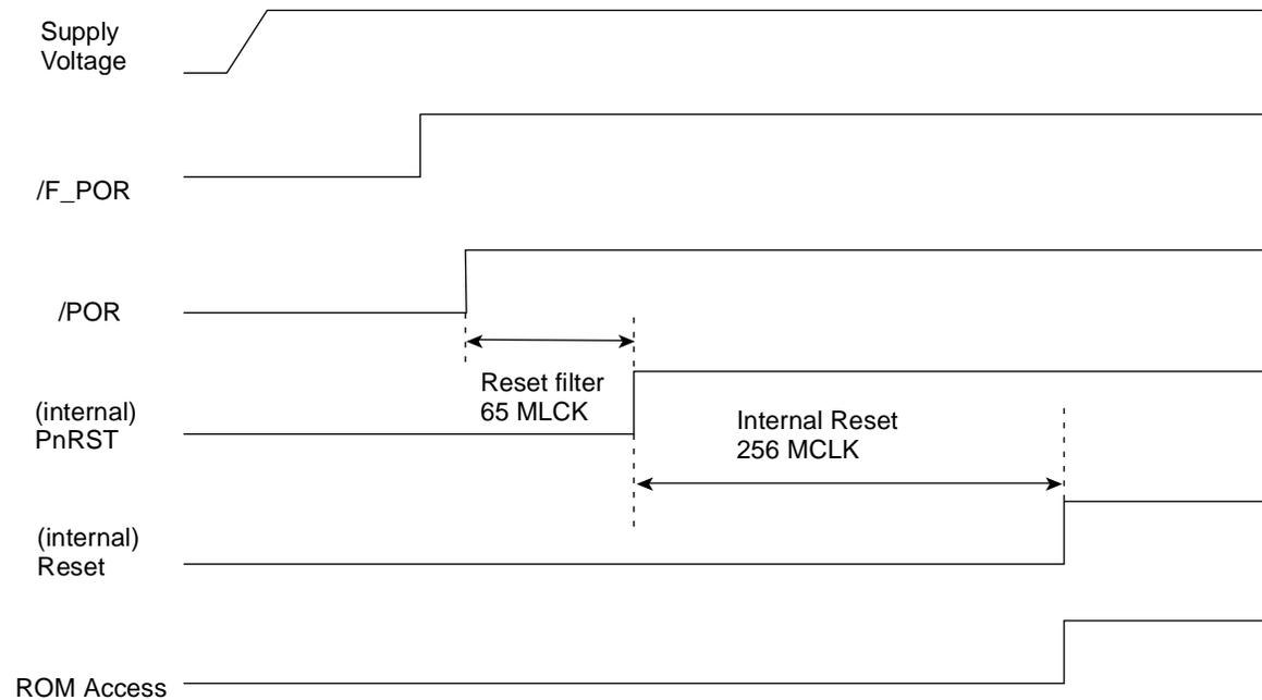
FIG. 7-9: POWER RESET TIMING DIAGRAM
