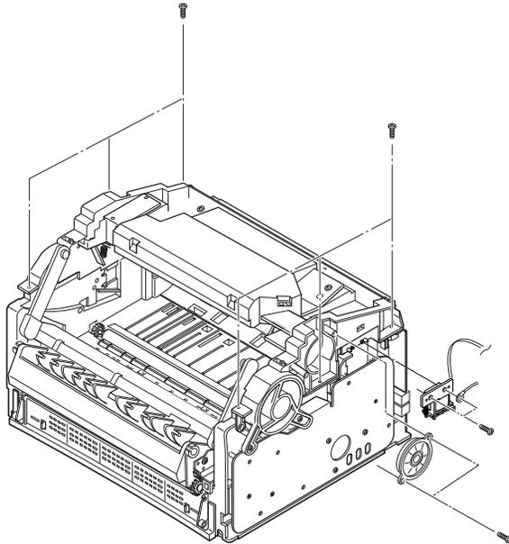
3. Unlatch the front end, then lift the upper frame up.
