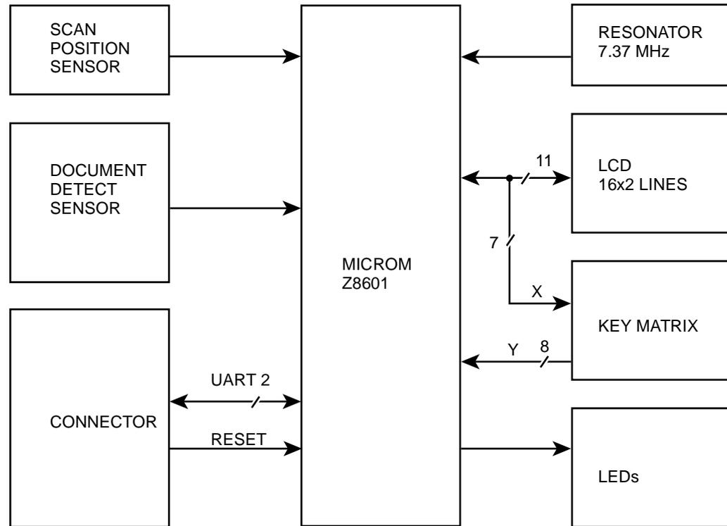
FIG. 7-13: OPE BLOCK DIAGRAM
