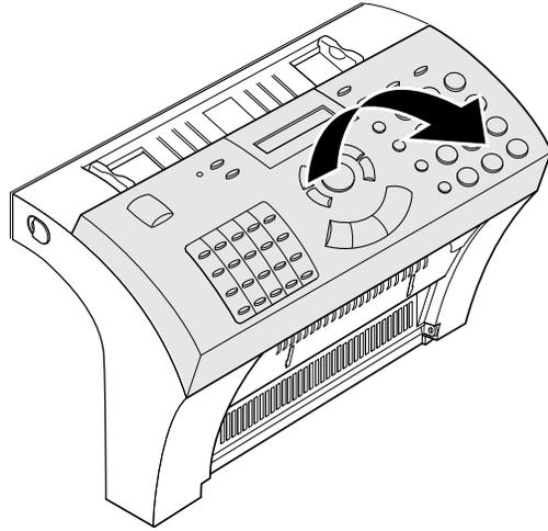
5. Remove the stopper holding the OPE Cover.
