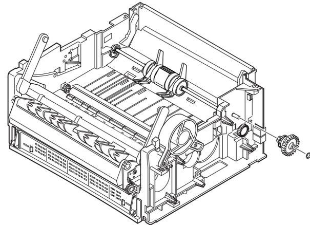
5. Pull the shaft forward and to the left to view a pin at the right end. Remove the pin passing through the shaft, then pull the roller shaft to the right, and lift it up.
