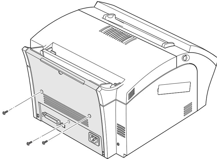
2. Unlatch the bottom ends, then remove the rear cover.
