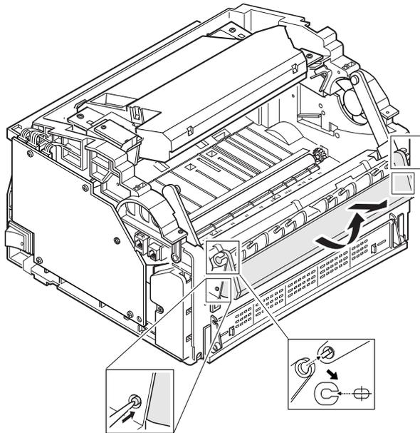
3. Remove the screw at the left side of the frame and unlatch the wire cap, then remove the cap.
