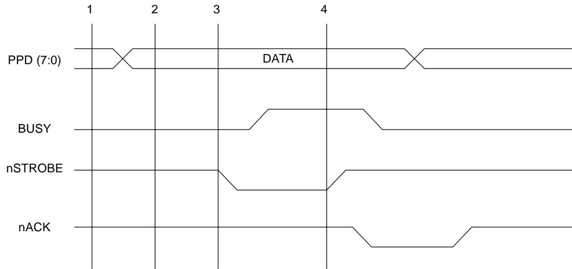
FIG. 7-5 COMPATIBILITY HARDWARE HANDSHAKING TIMING
