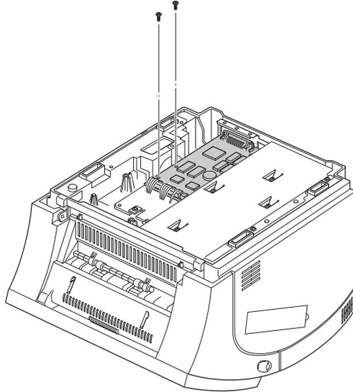
4. Remove two screws securing the printer connector.
