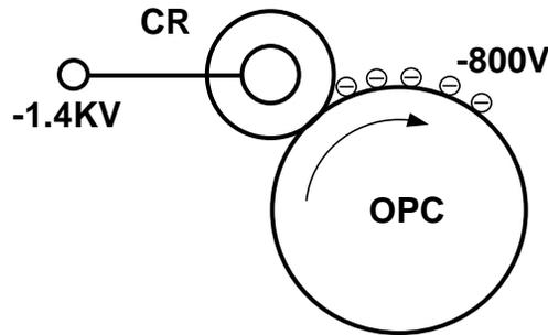
A negative voltage is applied to the surface of the OPC Drum. This is the first step in creating an electrophotograph. The high voltage section of the Engine Controller PBA supplies (-)1.4KV to the Charge Roller and transfers a charge of approximately (-)800 V to the OPC Drum.
