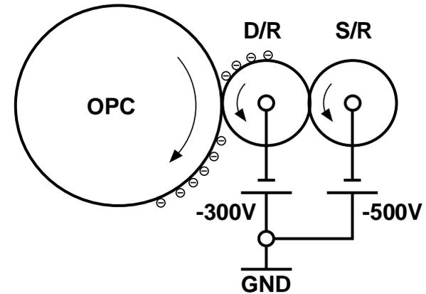
Surface moves between the DEV Roller and the OPC Drum. Negatively charged Toner is attracted to the high voltage(-50V) of the exposed portions of the OPC Drum and is exposed more easily than the more negative (-800V) surface voltage of unexposed areas of the OPC Drum, resulting in a latent image.
