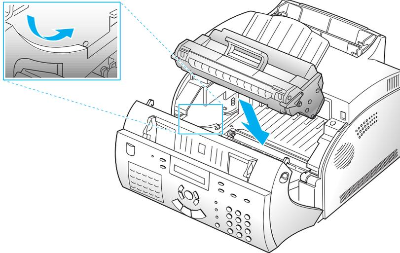
5. Grasp the handle and slide the cartridge down between the cartridge slots, until it drops into place.
