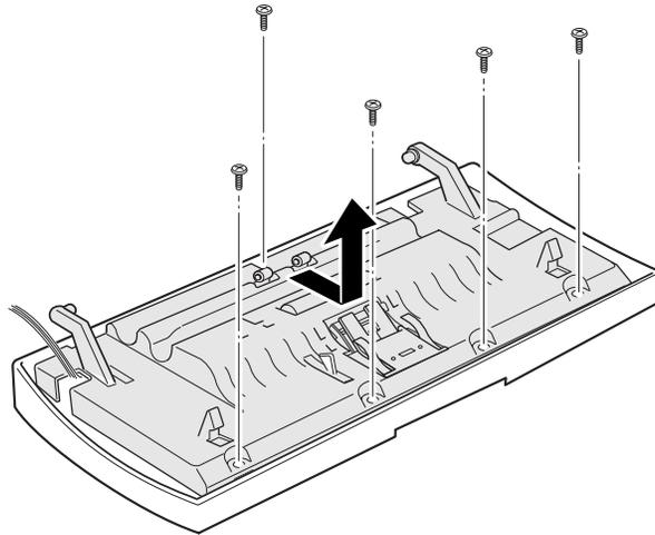
3. Remove eleven screws securing the PBA, then remove the PBA.
