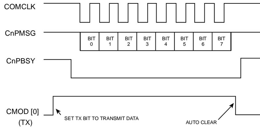
Command Message Transfers from KS32C6100 to Printer Engine
