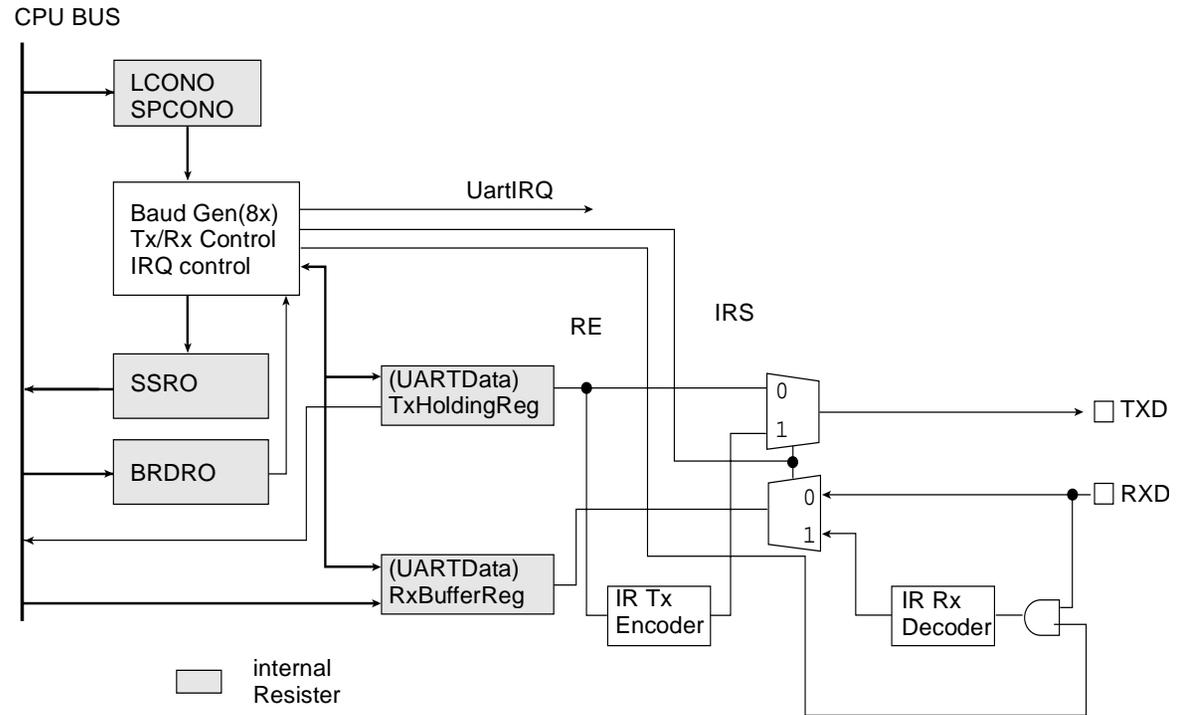
FIG. 7-2: UART BLOCK DIAGRAM
