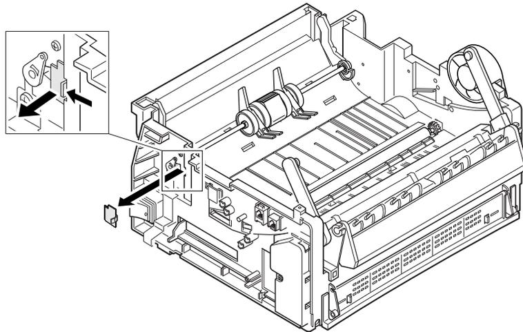
3. Remove one screw, then rotate the pickup bushing at the left end of the roller clock-wise.
