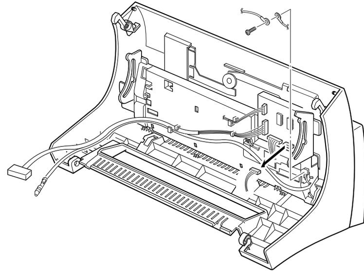
4. Lift the control panel by hand.
