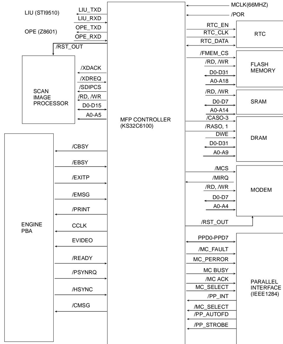
FIG. 7-1: ENTIRE STRUCTURE OF MAIN CIRCUIT FOR EACH KEY SIGNAL
