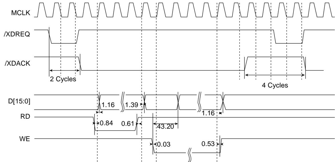
FIG. 7-4 EXTERNAL DMA TIMING DIAGRAM
