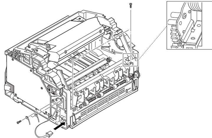
5. Unlatch the fuser using a small flat blade screwdriver.
