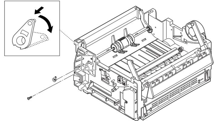
4. Remove E-ring at the right end of the roller, then remove the gear clutch.
