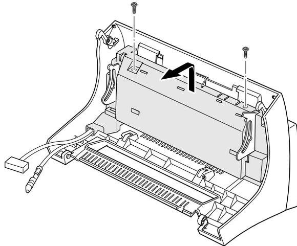
3. Unplug the OPE connector from the Scan PBA and remove ground screw.
