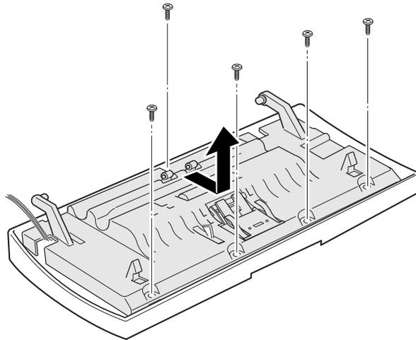
3. Turn the scan upper frame over, and remove three screws. Then, remove the Sensor bracket pinch spring, and pinch roller. To remove the pinch roller, push up from the bottom side.
