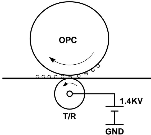
Toner moves from the surface of the OPC Drum to the paper via the Transfer Roller. Toner on the surface of the OPC DRUM will be attracted by the Transfer Roller, which is charged to approximately + 1.5 kV (600 ~ 2800V), depending upon temperature, and humidity. Toner then moves from the OPC DRUM to the paper.
