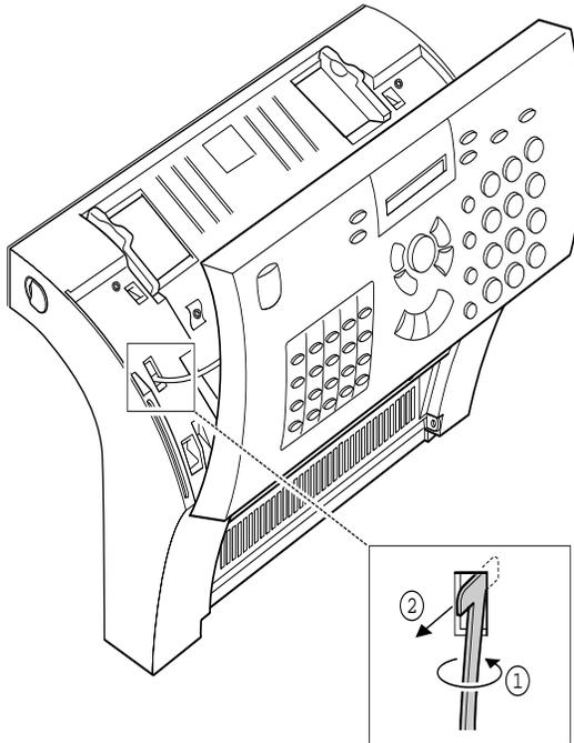
6. Unlatch the bottom ends, then remove the OPE cover.
