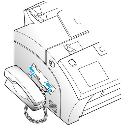
*Note: If you want to remove the handset, pushing (A) in the bottom, slide it down and towards the front of the machine, then take it out.*
