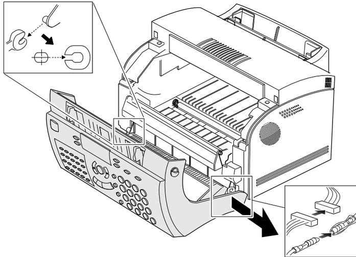
7. Disconnect the ground wire and connector.
