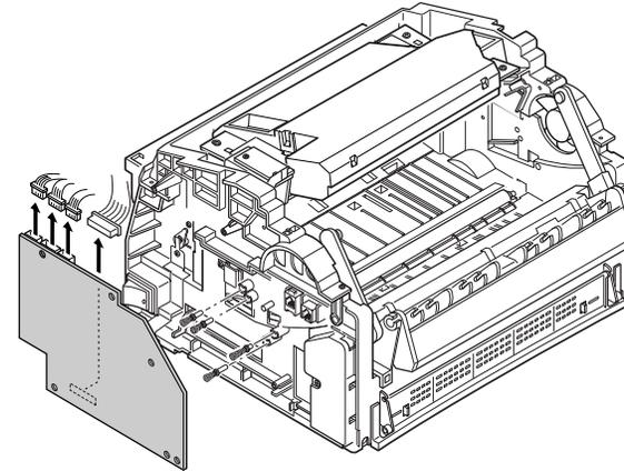
*Note: When you reassemble the HVPS PBA, make sure that the high voltage electrodes, contacts, springs and pins are inserted correctly.*
