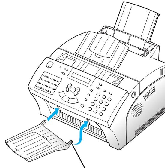
Insert one end first, then the other end by pulling this leg inward to make the tray easy to insert.
