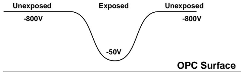
LSU receives the transferred bitmap image data from the Engine PBA and turns the LSU's laser diode on and off, exposing the OPC Drum. If there is no data to print the Laser Diode remains off and the OPC Drum is not exposed. Portions of the OPC Drum exposed charged to approximately (-)50V by the laser beam while unexposed portions charge to (-)800V. The image formed by the exposed laser beam is invisible, and is called a latent image.
