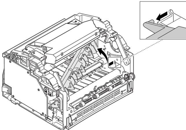
7. Release the left end, then remove the fuser.
