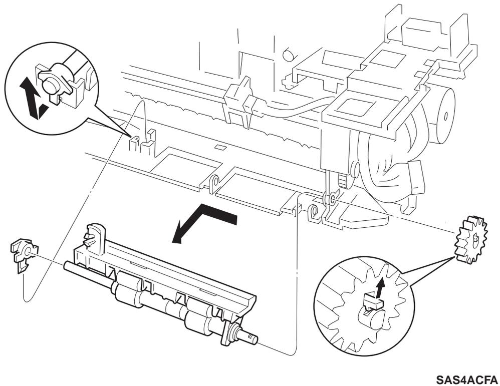
Figure 9.3.11.1 Removing the Exit Roll Assembly
