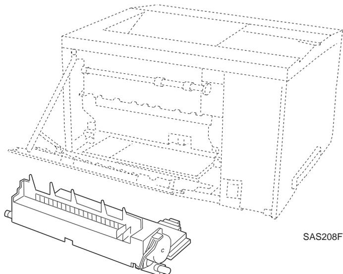
Figure 10.1.1.2.1 Installation in the Base Engine
