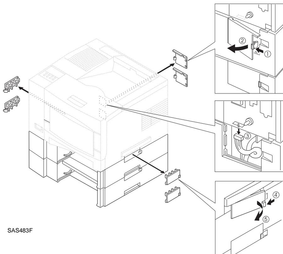
**Figure 8.3.1.1 Removing Feeder 2 and 3**
