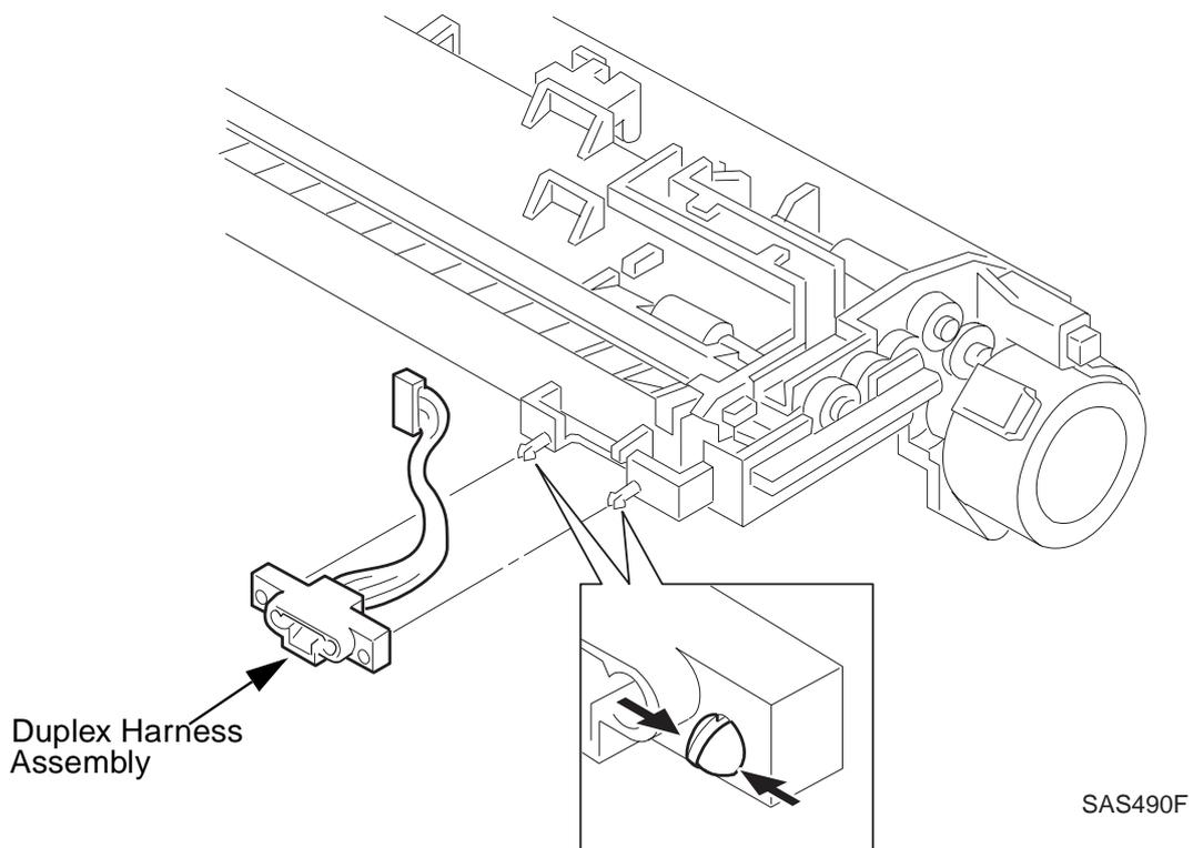
Figure 10.3.9.1 Removing the Duplex Harness Assembly
