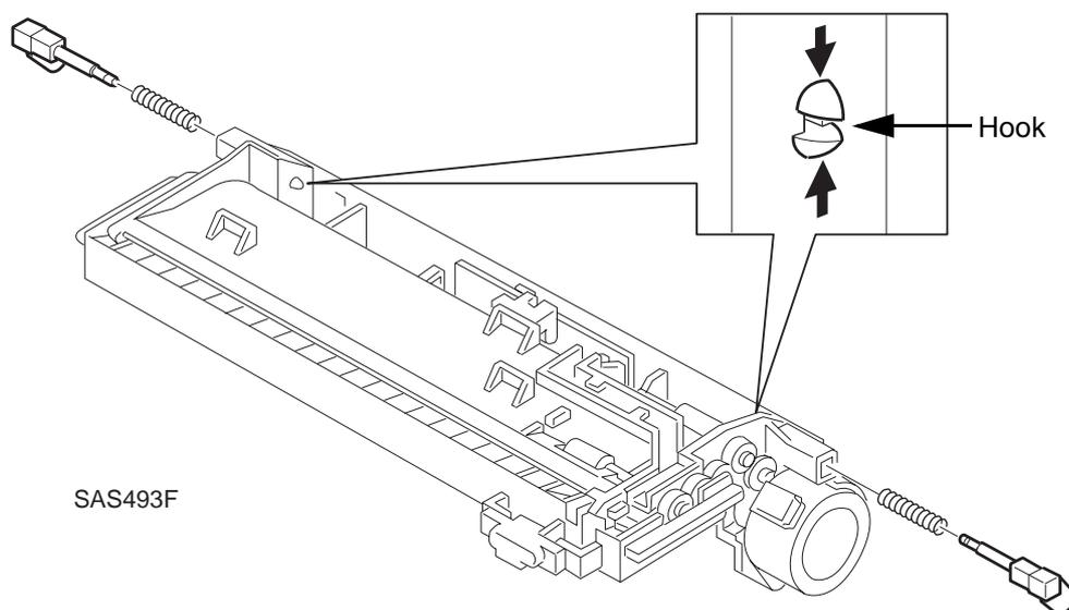
**Figure 10.3.12.1 Removing the Latch**
