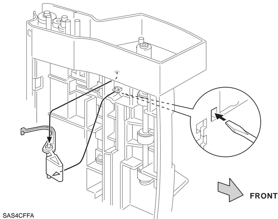
**Figure 11.3.10.1 No Paper Actuator Removal**
