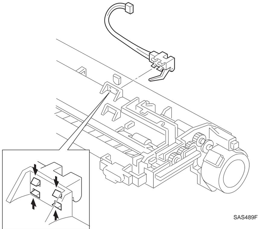
**Figure 10.3.8.1 Removing the Duplex Sensor Assembly**
