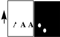
Deletion is an area of the print where the image is missing or extremely light. Spot deletions are missing spots localized to small areas of the page.
