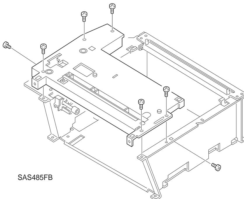
**Figure 8.3.2.1 Removing the 500 Chute Assembly**
