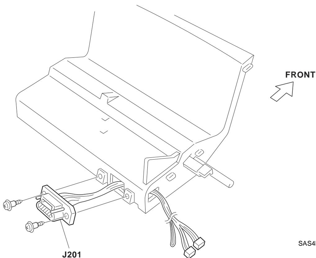
Figure 11.3.13.1 Envelope Harness Assembly Removal
