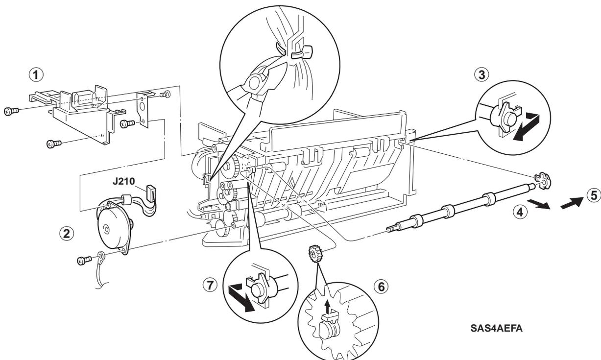
**Figure 9.3.13.1 Removing the Drive Motor Assembly/Middle Roll Assembly**
