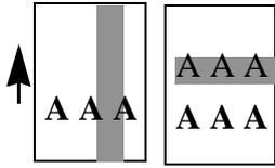
A ghost image, either from a previously printed page or the page in progress, is transferring onto the print due to incomplete cleaning at the end of printing cycle.
