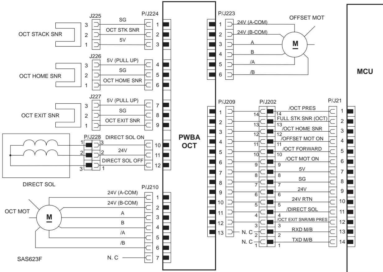
18. MCU ↔ OCT STACK SENSOR, OCT HOME SENSOR, OCT EXIT SENSOR, OCT DIRECTION SOLENOID, OCT MOTOR, AND OCT OFFSET MOTOR
