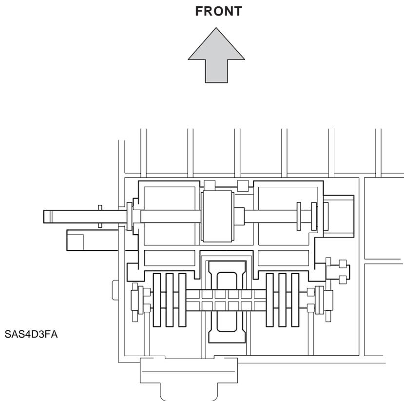
**Figure 11.3.12.2 Pinch Roll/Feed Bearing/Pinch Spring Reinstalled**
