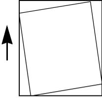
The image is not parallel to the edges of the print sheet.
