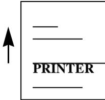
Unnecessary streaks run across the entire or partial page in a horizontal or vertical direction. The width of these streaks should be less than 1.0mm.
