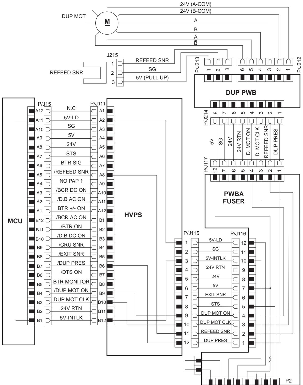
9. FUSER PWB ↔ DUPLEX PWB ↔ DUPLEX MOTOR, AND REFEED SENSOR
