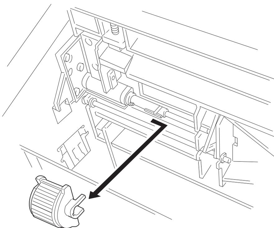
**Figure 8.3.5.1 Removing the 500 Feed Roll Assembly**
