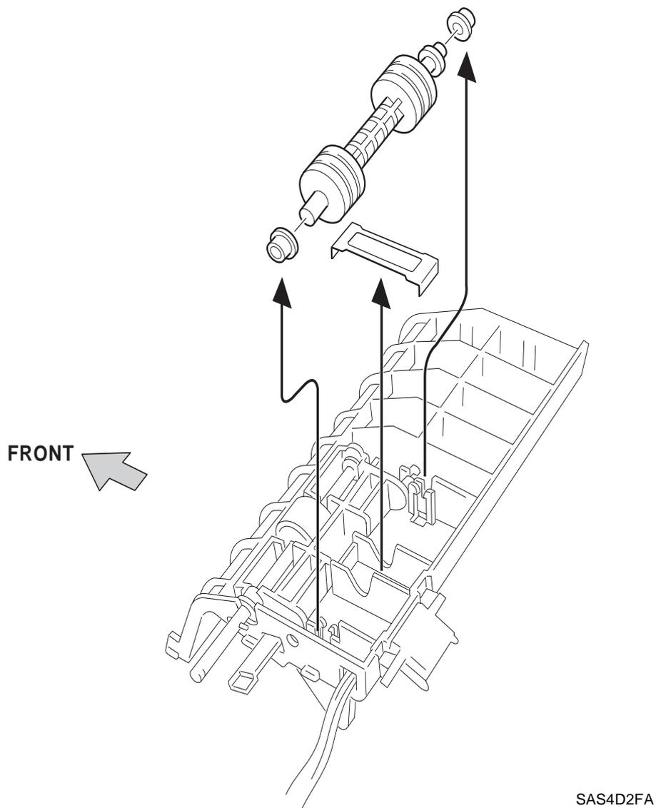
**Figure 11.3.12.1 Pinch Roll/Feed Bearing/Pinch Spring Removal**
