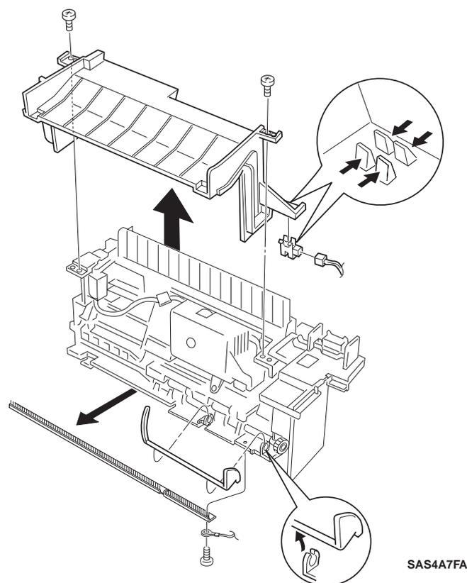
Figure 9.3.6.1 Removing the Lower Chute/Full Stack Sensor/Full Stack Actuator
