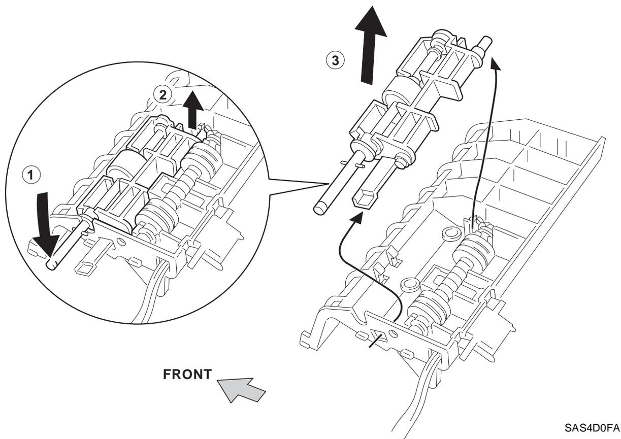
Figure 11.3.11.1 Retard Holder & Retard Roll Assembly Removal
