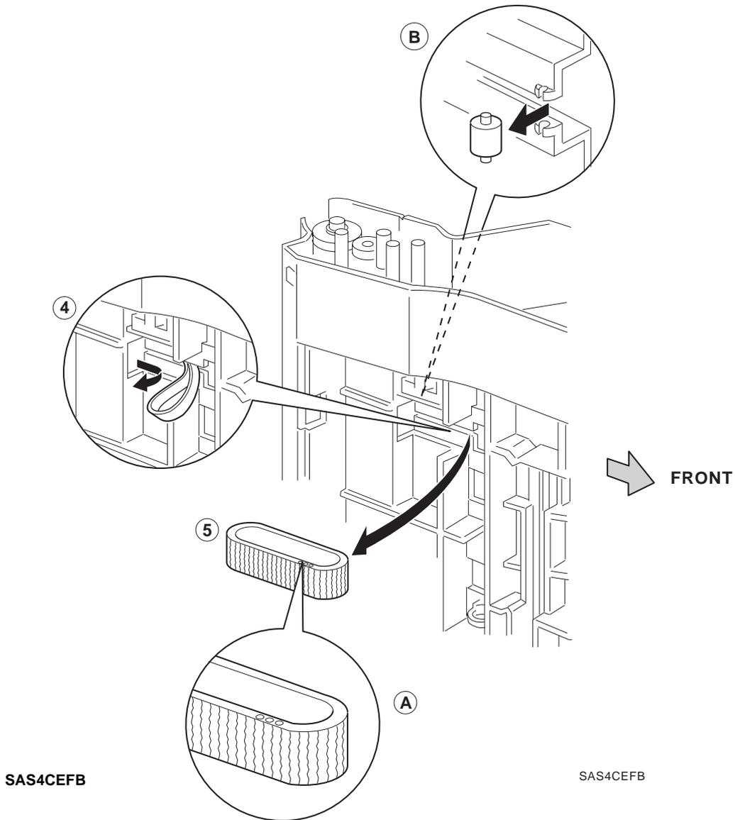
Figure 11.3.9.2 Feed Belt Removal
