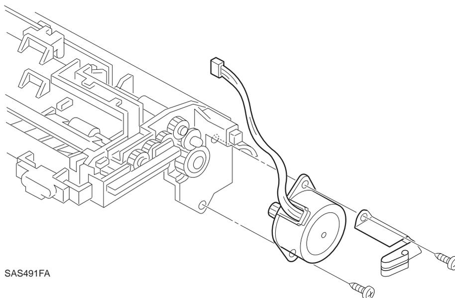
Figure 10.3.10.1 Duplex Motor Assembly
