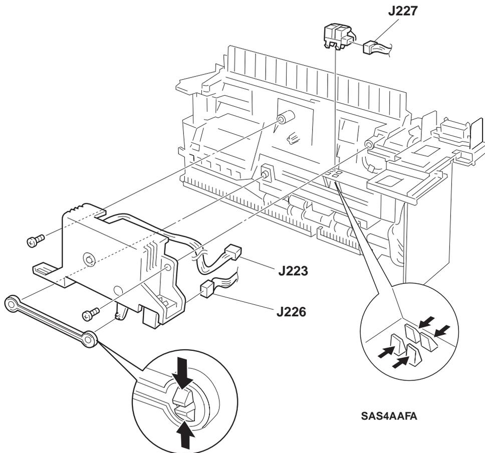
Figure 9.3.9.1 Removing the Offset Assembly/Exit Sensor Assembly
