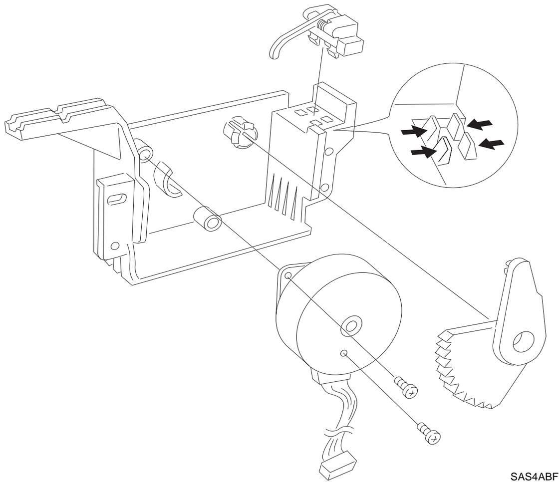
Figure 9.3.10.1 Removing the Offset Motor/OCT Sensor/Cam Gear
