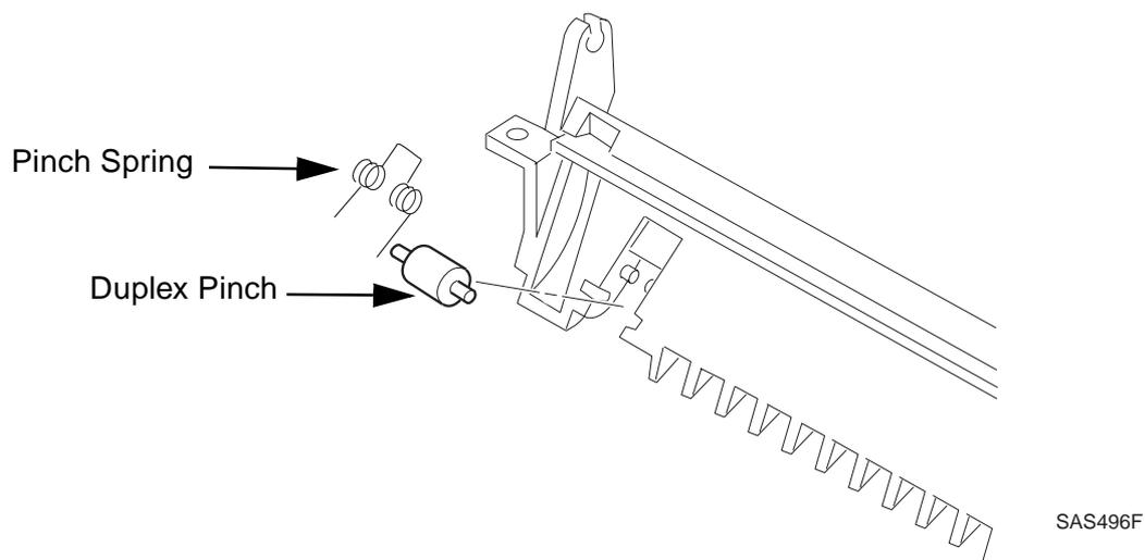
Figure 10.3.3.1 Removing the Duplex Pinch Roll
