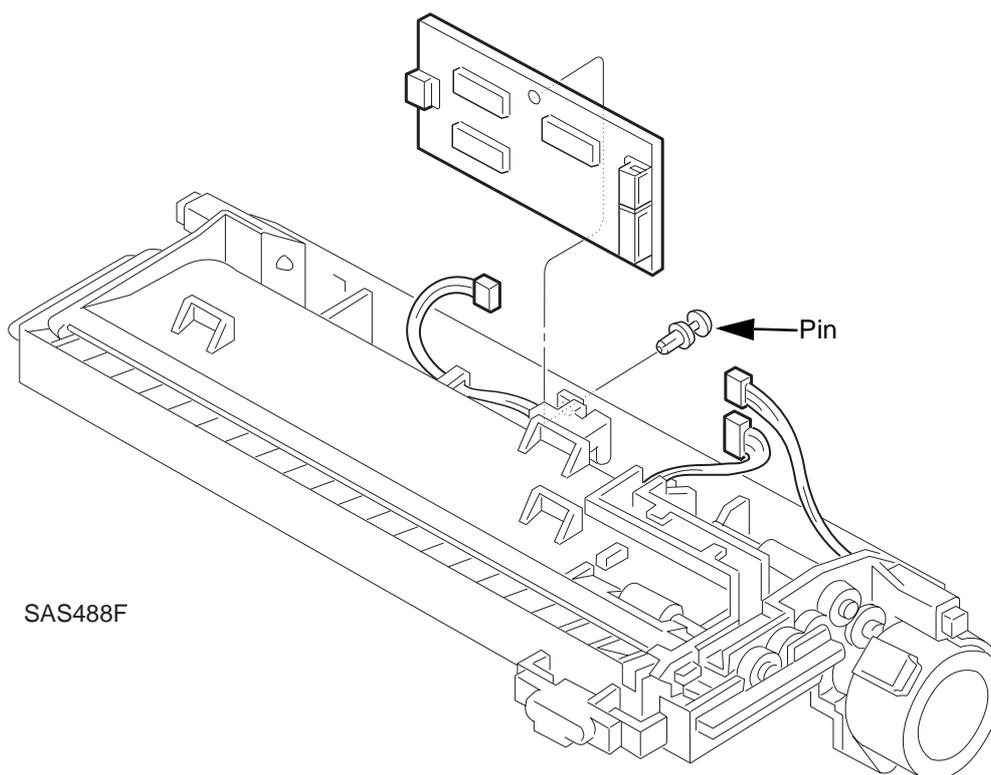
**Figure 10.3.7.1 Removing the Duplex PWB Assembly**
