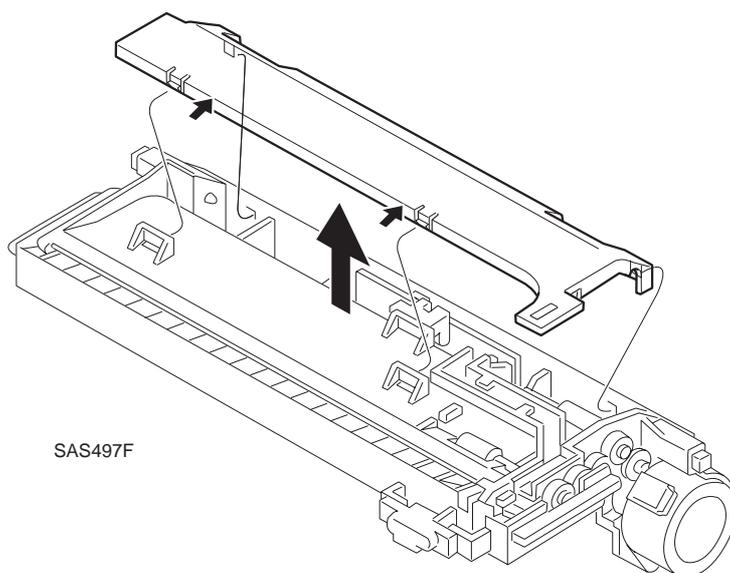
Figure 10.3.4.1 Removing the Duplex Cover
