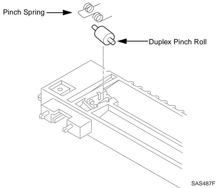
Figure 10.3.6.1 Removing the Duplex Pinch Roll (Connector Chute Side)
