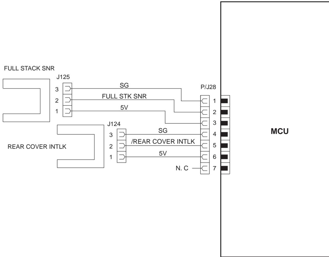
16. MCU ↔ FULL STACK SENSOR AND REAR COVER SENSOR
