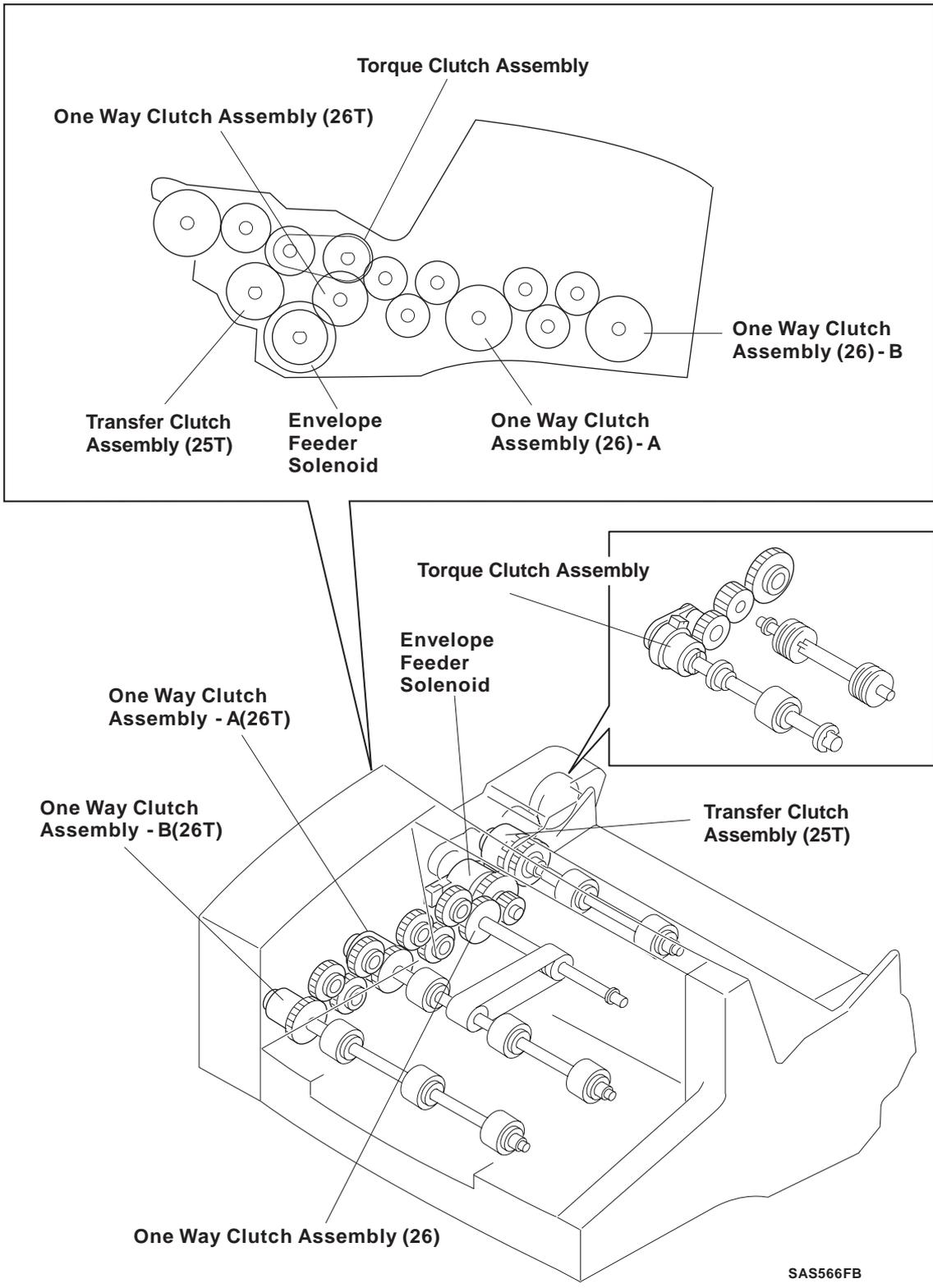
**Figure 11.6.2b Major Components of the Envelope Feeder**
